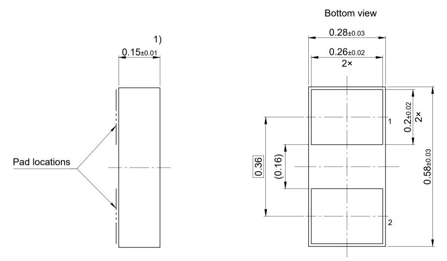
1) The total package height includes the pad thickness
