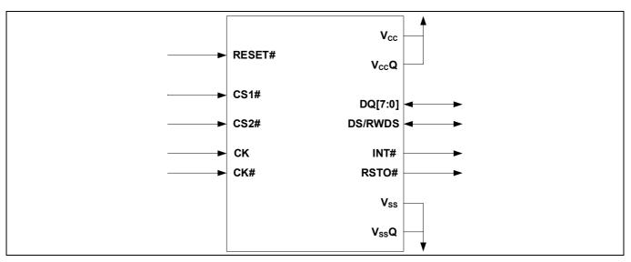
Figure 1 HYPERBUS™ MCP signal diagram
