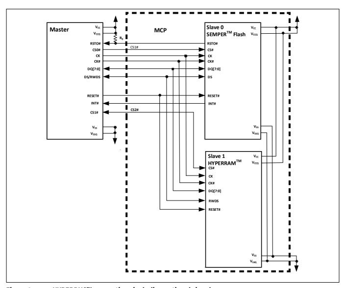
Figure 2 HYPERBUS™ connections including optional signals
