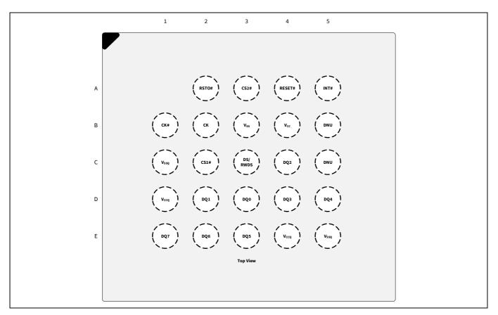
Figure 3 24-ball FBGA, 8 × 8 mm, 5 × 5 ball footprint (top view)
