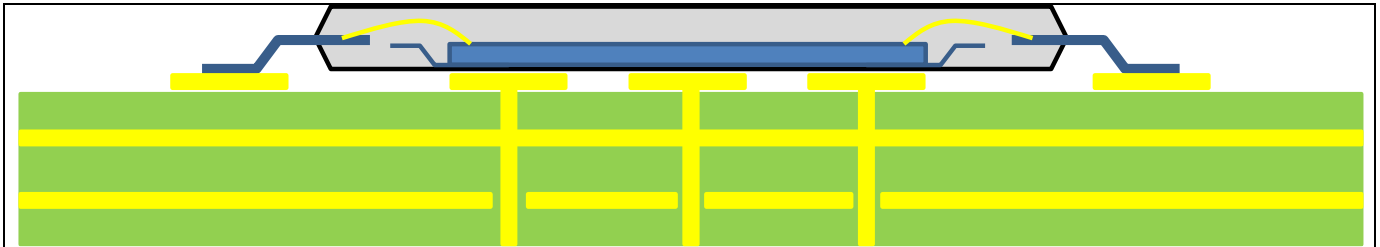
Figure 7-1: Example Thermal Via Holes on PCB.
