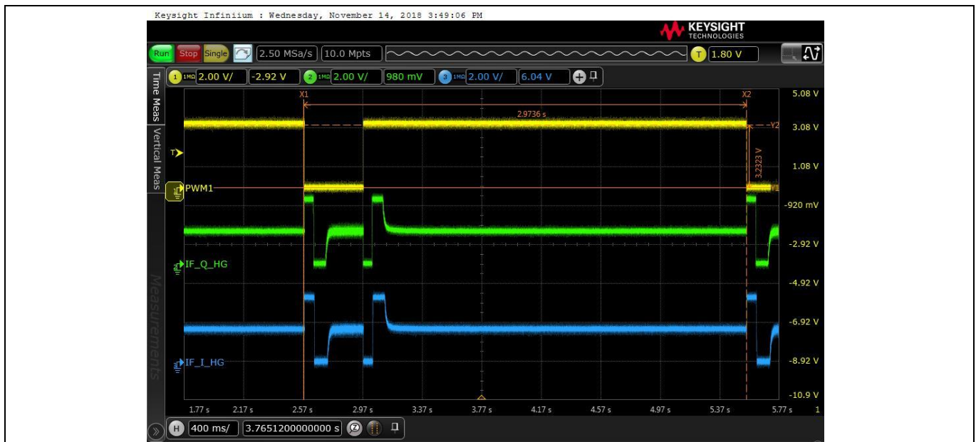
Figure 15 PWM1, IF_Q and IF_I signals for on-time = 400 ms and frame interval time = 3000 ms
