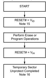
Figure 7. Temporary Sector Unprotect Operation<sup>[15, 16]</sup>
