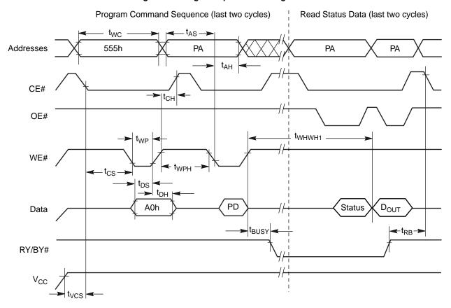
Figure 20. Accelerated Program Timing Diagram
