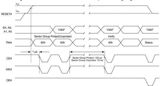
Figure 27. Sector/Sector Block Protect and Unprotect Timing Diagram<sup>[80]</sup>
