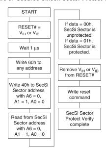
Figure 8. Secured Silicon Sector Protect Verify
