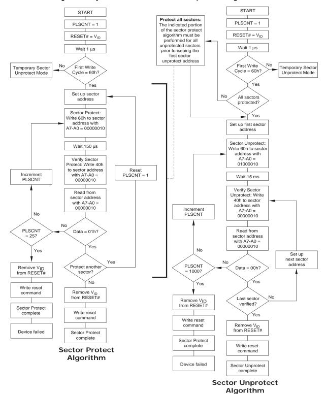
Figure 6. In-System Sector Protection/Sector Unprotection Algorithms
