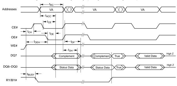
Figure 23. Data# Polling Timings (During Embedded Algorithms)<sup>[76]</sup>
