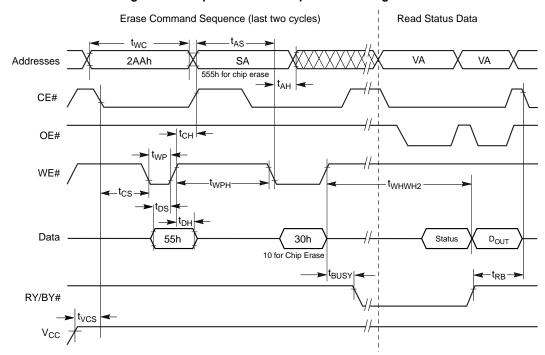
Figure 21. Chip/Sector Erase Operation Timings [75]
