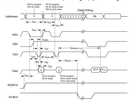
Figure 28. Alternate CE# Controlled Write (Erase/Program) Operation Timings  $^{[83,\ 84,\ 85]}$
