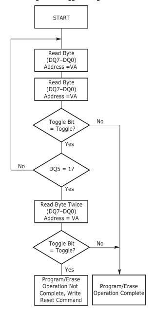
Figure 12. Toggle Bit Algorithm $^{[52]}$
