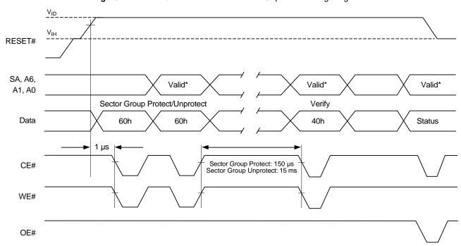
Figure 17.4 Sector/Sector Block Protect and Unprotect Timing Diagram<sup>[61]</sup>
