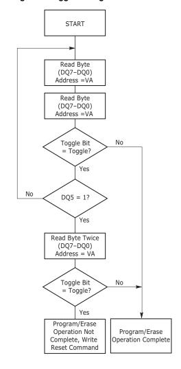
Figure 7. Toggle Bit Algorithm<sup>[29]</sup>
