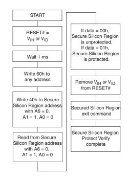
Figure 3. Secured Silicon Region Protect Verify
