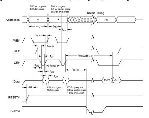
Figure 21. Alternate CE# Controlled Write (Erase/Program) Operation Timings<sup>[64, 65, 66, 67]</sup>
