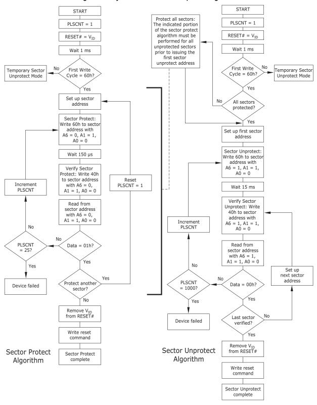
Figure 2. In-System Sector Protect/Unprotect Algorithms
