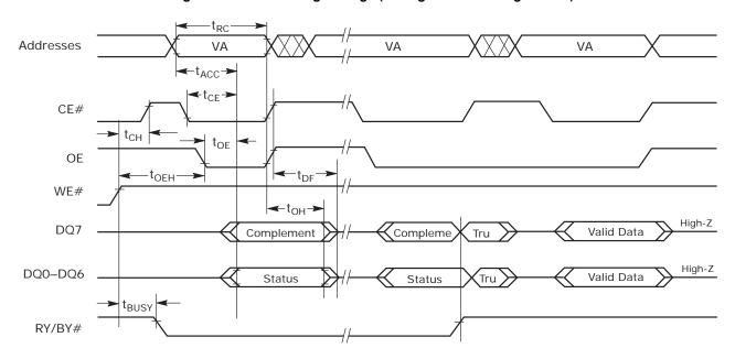
Figure 18. Data# Polling Timings (During Embedded Algorithms)<sup>[57]</sup>
