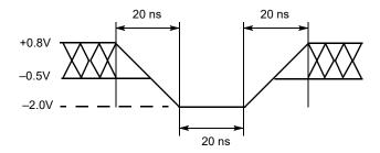
Figure 9. Maximum Positive Overshoot Waveform
