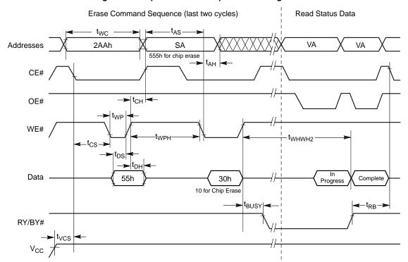
Figure 16. Chip/Sector Erase Operation Timings<sup>[55, 56]</sup>
