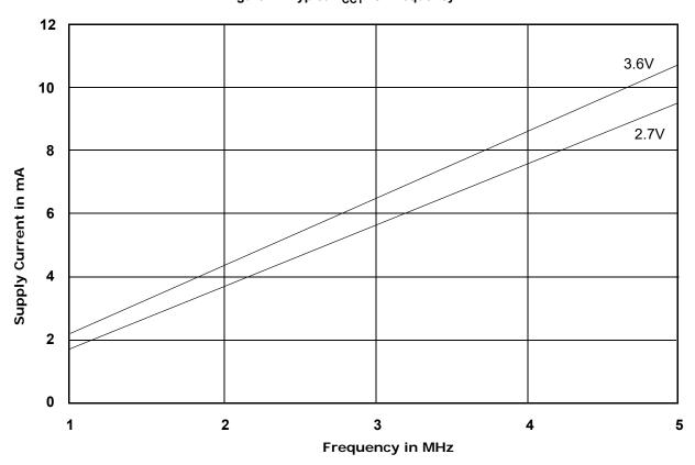
Figure 11. Typical I<sub>CC1</sub> vs. Frequency<sup>[43]</sup>
