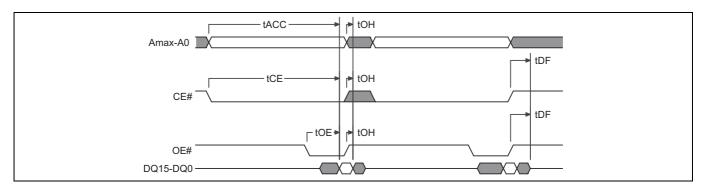
Figure 24 Back to Back Read (t<sub>ACC</sub>) operation timing diagram
