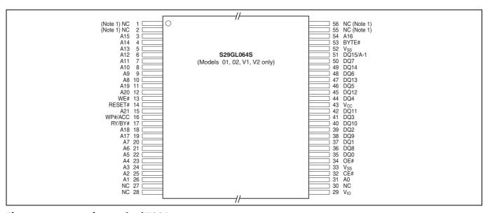
Figure 3 56-pin standard TSOP
