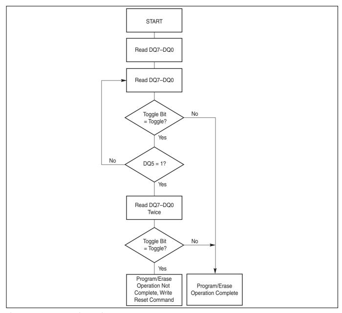
Figure 14 Toggle bit algorithm
