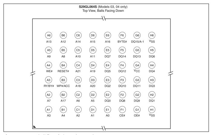
Figure 5 48-ball fine-pitch BGA (VBK 048)
