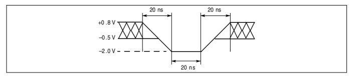
Figure 17 Maximum negative overshoot waveform
