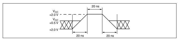
Figure 18 Maximum positive overshoot waveform
