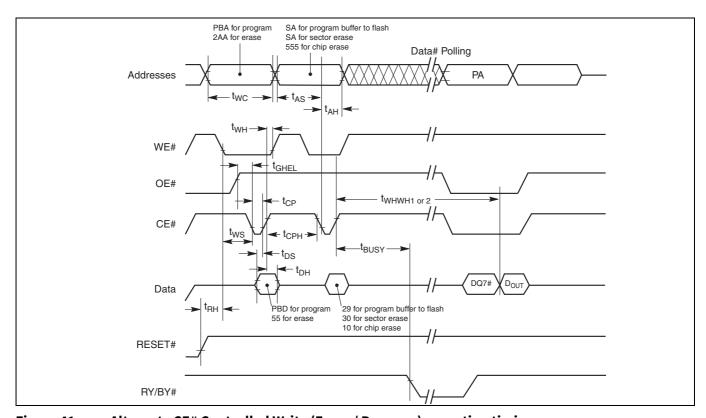
Figure 41 Alternate CE# Controlled Write (Erase / Program) operation timings
