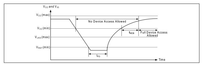
Figure 16 Power-down and voltage drop
