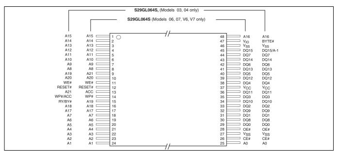
Figure 2 48-pin standard TSOP
