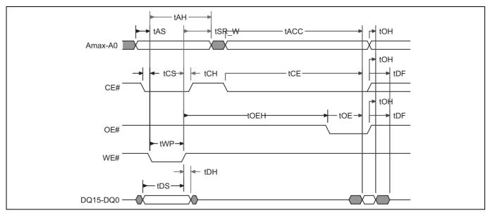
Figure 30 Write to Read (t<sub>CE</sub>) operation timing diagram
