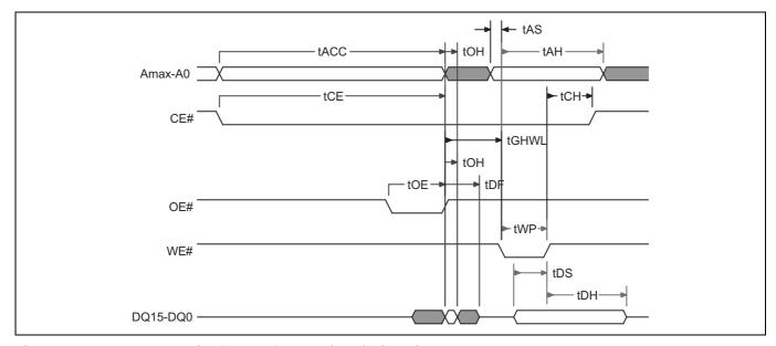
Figure 31 Read to Write (CE# V<sub>IL</sub>) operation timing diagram
