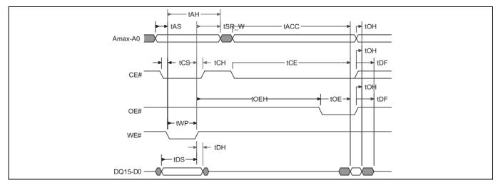
Figure 40 (CE#) Write to Read operation timing diagram
