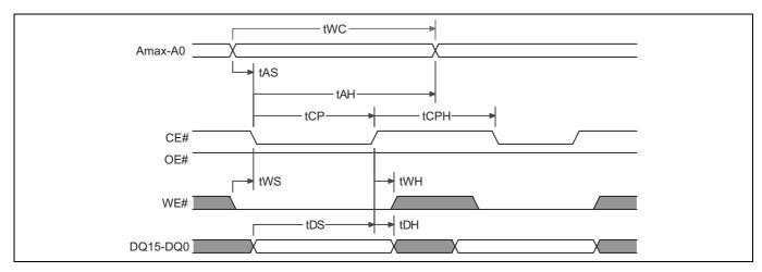
Figure 39 Back to Back (CE#) Write operation timing diagram
