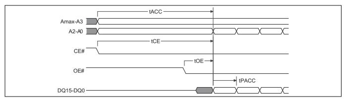
Figure 26 Page Read timing diagram
