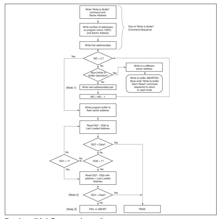
Figure 9 Write buffer programming operation
