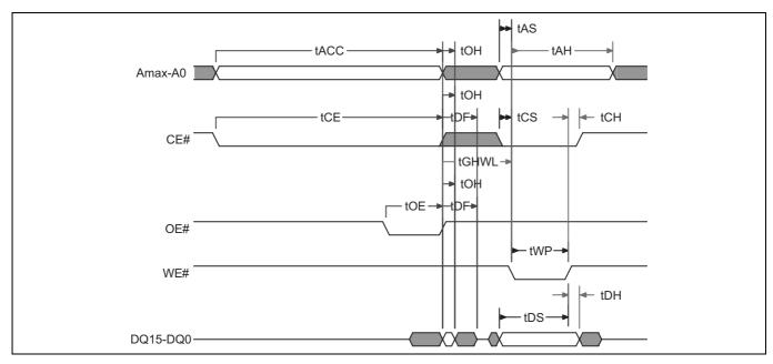
Figure 32 Read to Write (CE# Toggle) operation timing diagram
