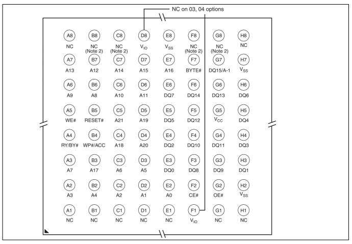
Figure 4 64-ball fortified BGA
