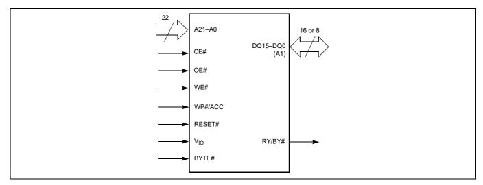
Figure 6 S29GL064S logic symbol (models 01, 02, V1, V2)
