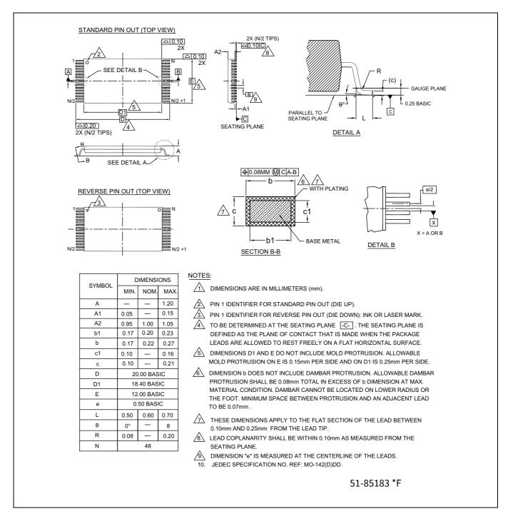
Figure 42 48-pin TSOP (18.4 × 12.0 × 1.2 mm) package outline, 51-85183
