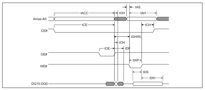
Figure 24 Read to write (CE# V<sub>IL</sub>) operation timing diagram
