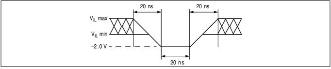
Figure 11 Maximum negative overshoot waveform
