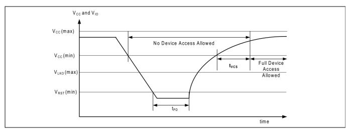
Figure 10 Power-down and voltage drop
