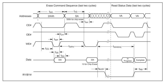
Figure 27 Chip/sector erase operation timing diagram<sup>[98]</sup>
