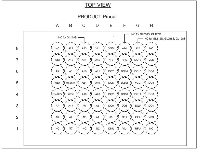
Figure 36 64-ball Fortified Ball Grid Array<sup>[107, 108, 109]</sup>
