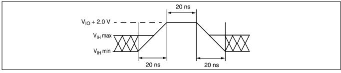
Figure 12 Maximum positive overshoot waveform
