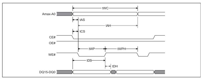
Figure 21 Back-to-back (CE#VIL) write operation timing diagram
