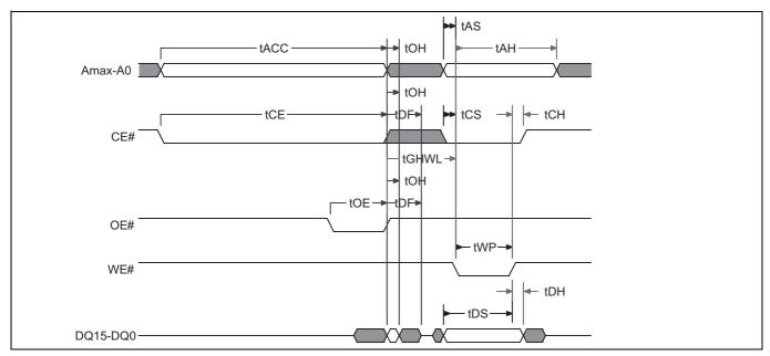
Figure 25 Read to write (CE# Toggle) operation timing diagram
