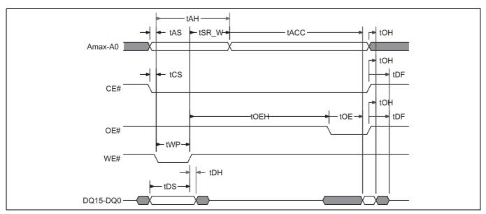
Figure 22 Write to read (t<sub>ACC</sub>) operation timing diagram
