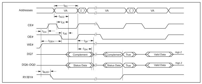
Figure 29 Data# Polling timing diagram (During Embedded Algorithms)<sup>[101]</sup>
