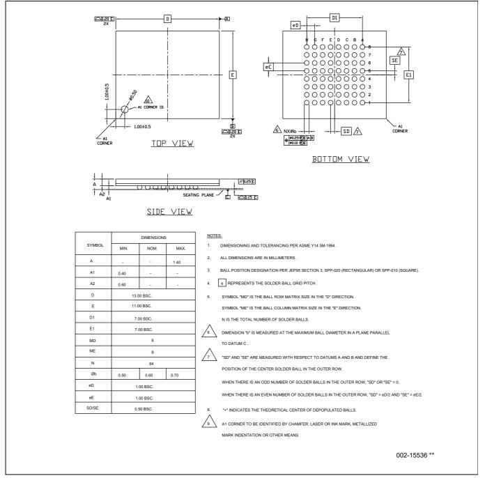
Figure 38 LAA064–64-ball Fortified Ball Grid Array (FBGA)
