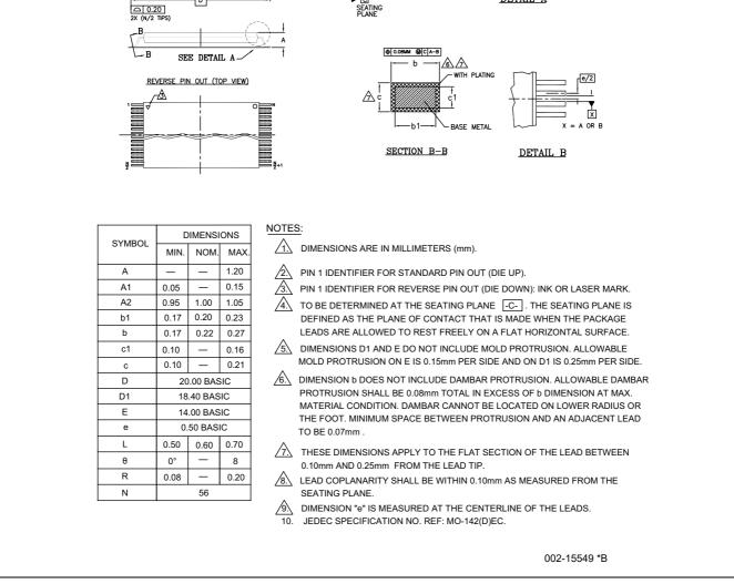
Figure 35 56-pin thin small outline package (TSOP), 14 x 20 mm
