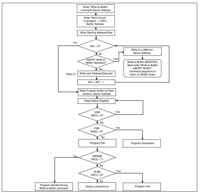
Figure 5 Write Buffer Programming Operation with Status Register
