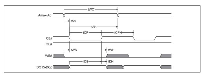
Figure 32 Back-to-back (CE#) write operation timing diagram
