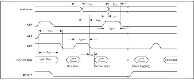
Toggle bit timing diagram (During Embedded Algorithms)<sup>[102]</sup> Figure 30
