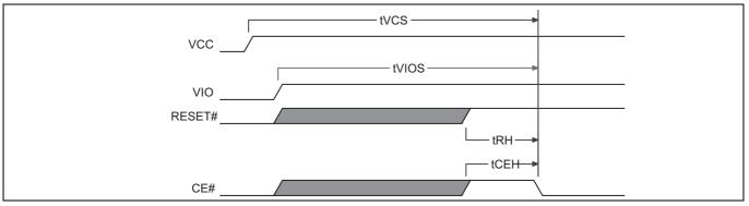
Figure 15 Power-Up diagram
