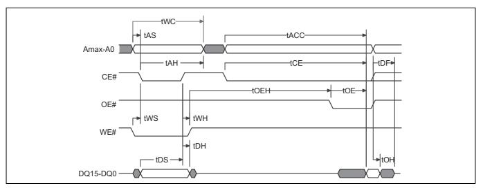
Figure 33 (CE#) write to read operation timing diagram
