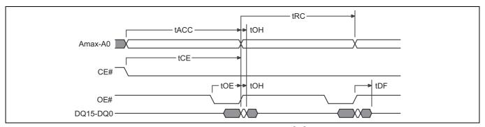
Figure 18 Back-to-back read operation (t<sub>RC</sub>) timing diagram<sup>[91]</sup>
