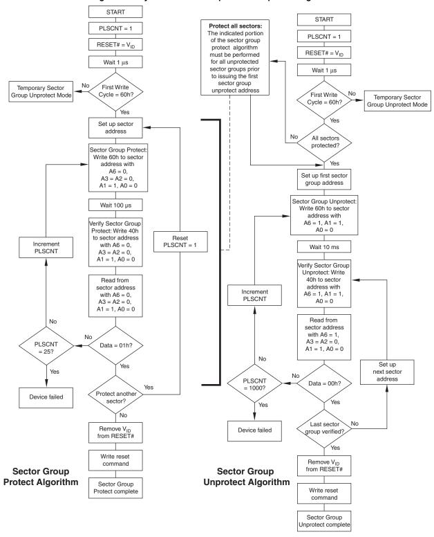
Figure 1. In-System Sector Group Protect/Unprotect Algorithms
