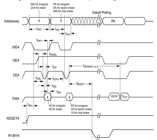
Figure 23. Alternate CE# Controlled Write Operation Timings  $^{[80,\;81,\;82]}$
