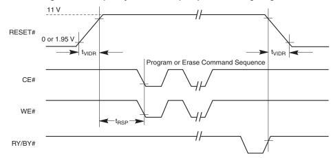
Figure 22. Sector Group Protect/Unprotect Timing Diagram<sup>[77]</sup>
