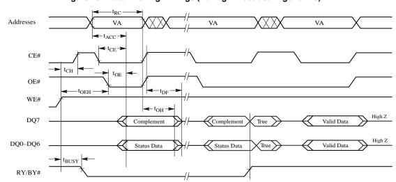
Figure 18. Data# Polling Timings (During Embedded Algorithms)[73]
