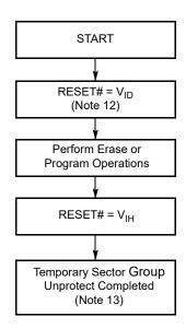
Figure 2. Temporary Sector Group Unprotect Operation
