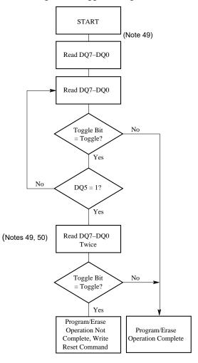
Figure 7. Toggle Bit Algorithm
