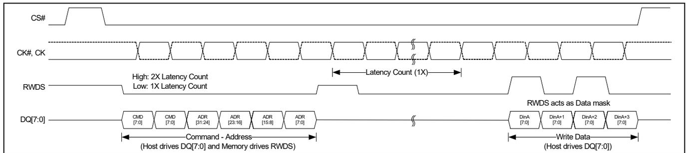
**Figure 15** WRITE with 1X latency transaction (DDR)<sup>[22, 23]</sup>
