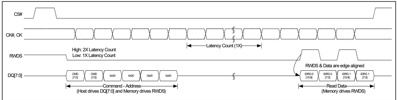
Figure 10 READ ID with 1X latency transaction (DDR)<sup>[16]</sup>
