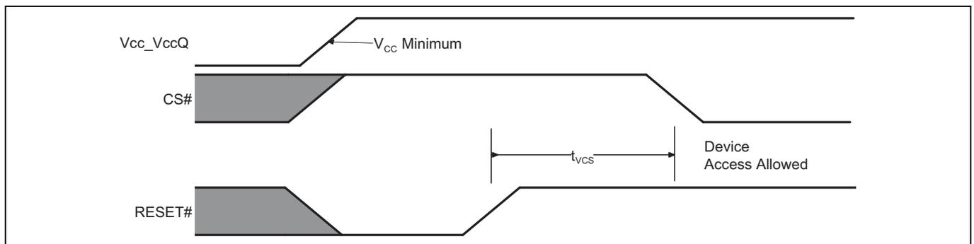
Figure 30 Power-up with RESET# LOW
