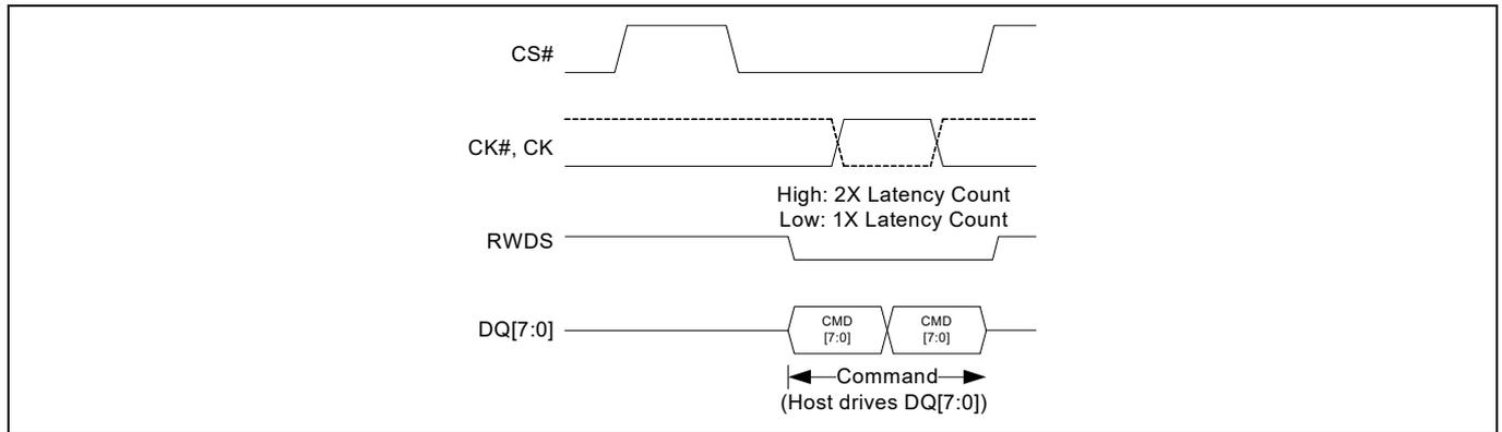
Figure 1 xSPI (Octal) command only transaction (DDR)
