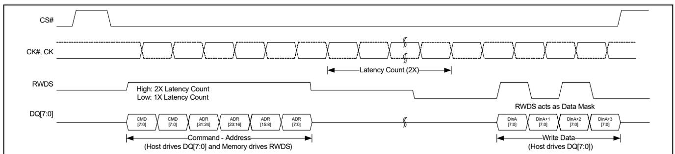
**Figure 16** WRITE with 2X latency transaction (DDR)<sup>[22, 23]</sup>
