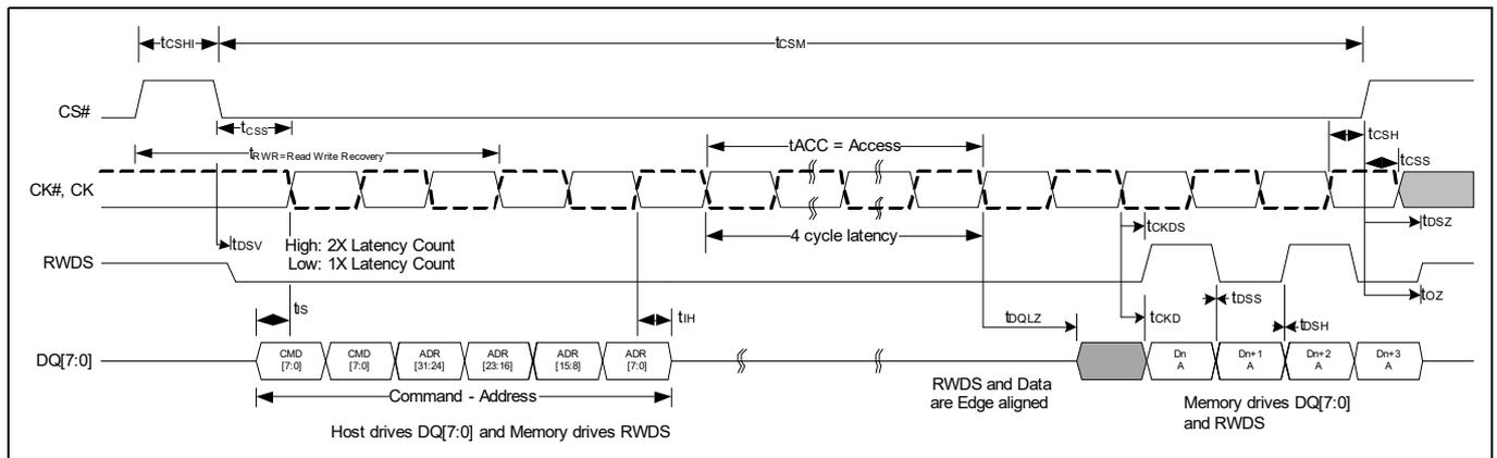
**Figure 36 Read timing diagram – No additional latency required**
