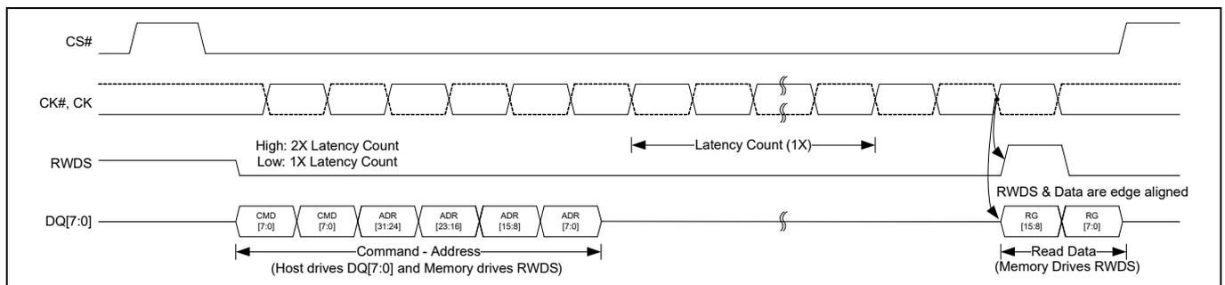
**Figure 19** READ ANY REGISTER with 1X latency transaction (DDR)<sup>[24]</sup>
