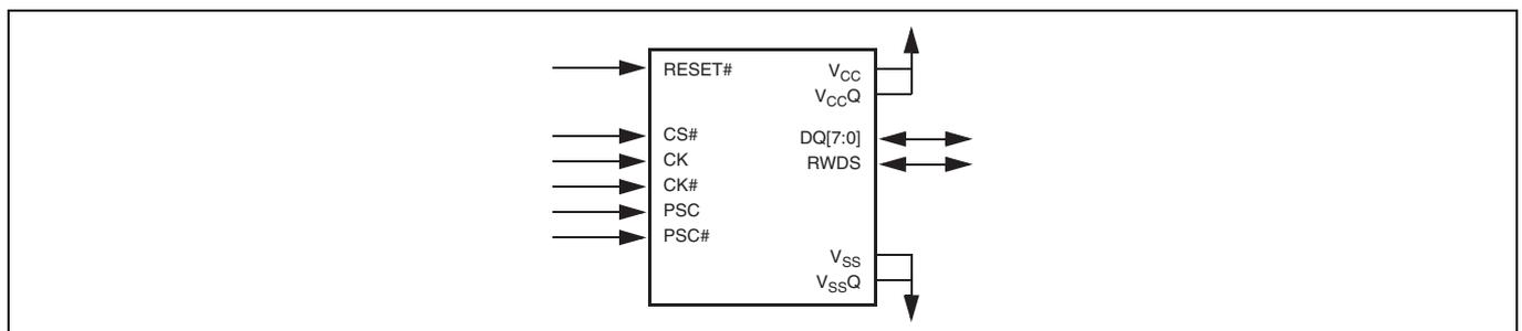
Figure 42 xSPI product with DCARS signal diagram
