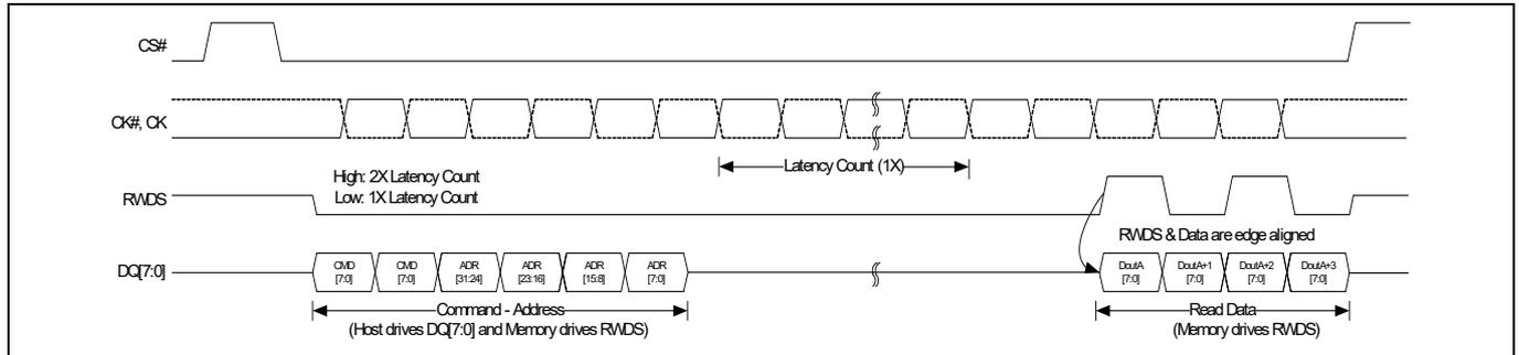
**Figure 13** READ with 1X latency transaction (DDR)<sup>[18]</sup>
