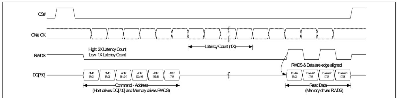
Figure 5 xSPI (Octal) read with 1X latency transaction (DDR) (All reads)<sup>[6]</sup>
