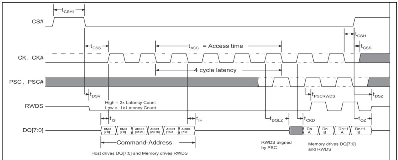
Figure 44 HYPERRAM™ memory DCARS timing diagram<sup>[61, 62, 63]</sup>
