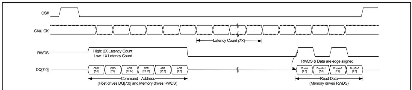
**Figure 14** READ with 2X latency transaction (DDR)<sup>[19]</sup>
