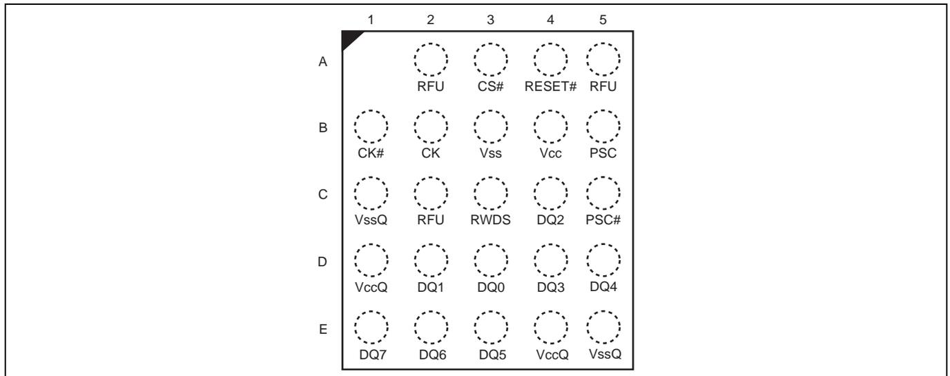
Figure 43 24-ball FBGA, 5 × 5 ball footprint, Top view
