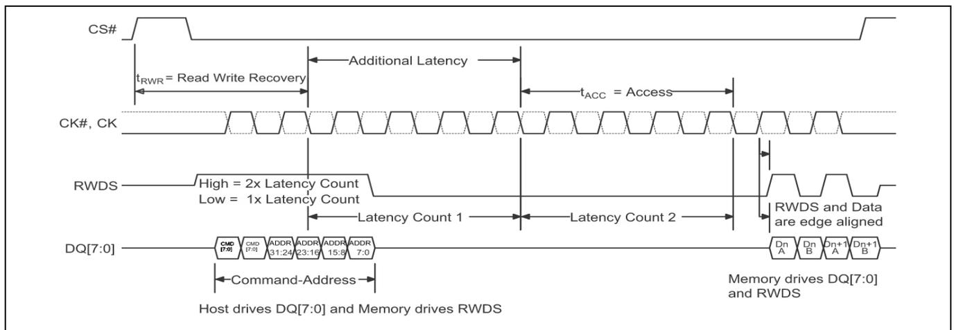
**Figure 37 Read timing diagram – With additional latency required**
