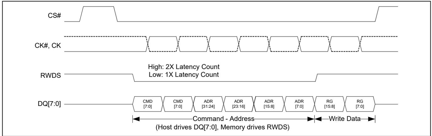
**Figure 21** xSPI (Octal) Write with no latency transaction (DDR) (Register writes)<sup>[26, 27]</sup>
