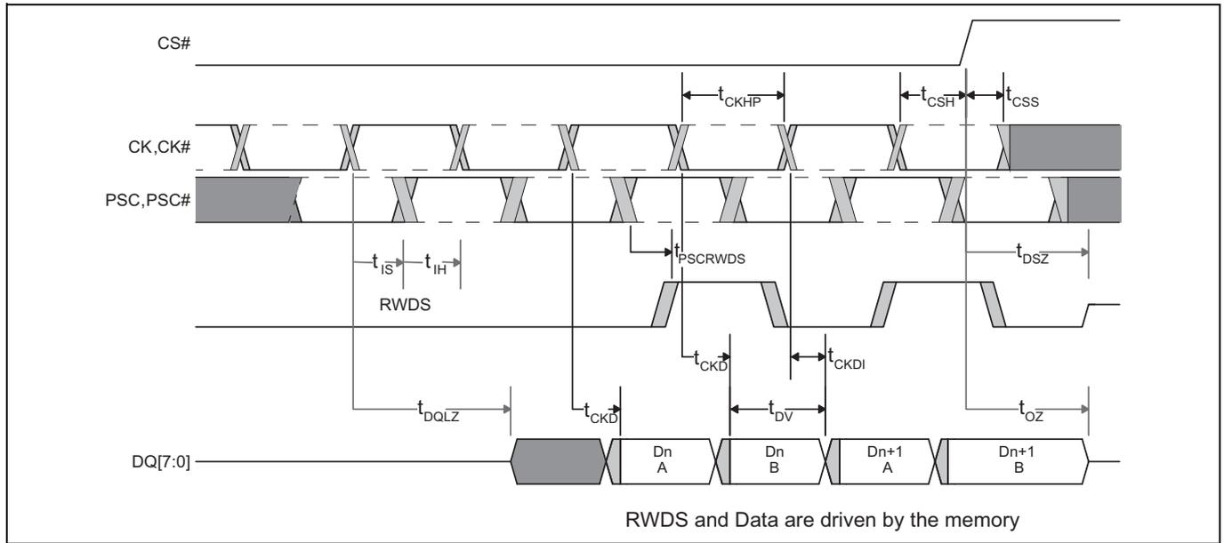
Figure 45 DCARS data valid timing<sup>[64, 65, 66, 67]</sup>
