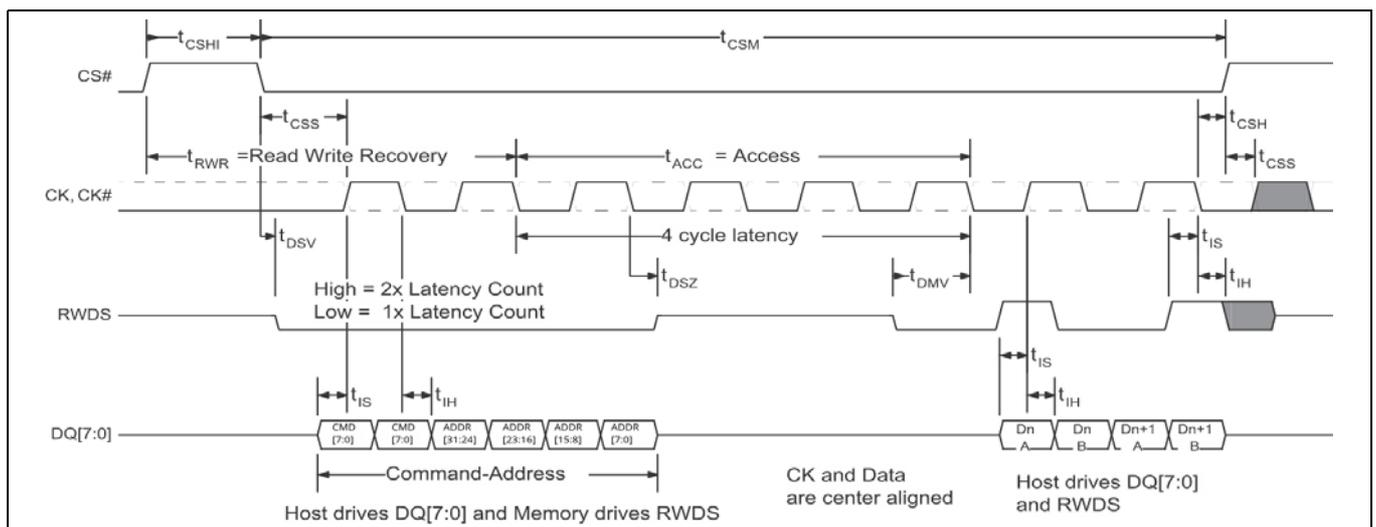
Figure 39 Write timing diagram – No additional latency
