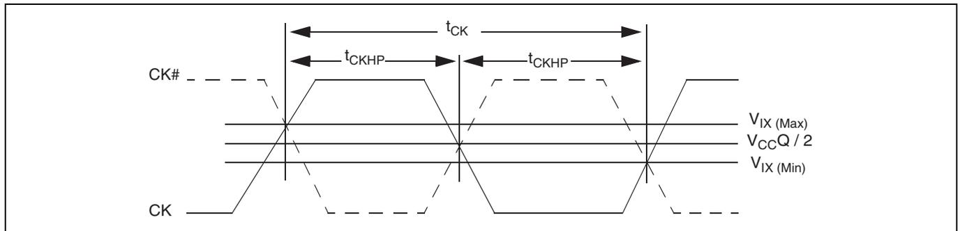
Figure 35 Clock characteristics
