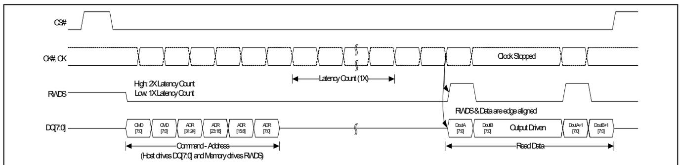
Figure 22 Active clock stop during Read transaction (DDR)<sup>[30]</sup>
