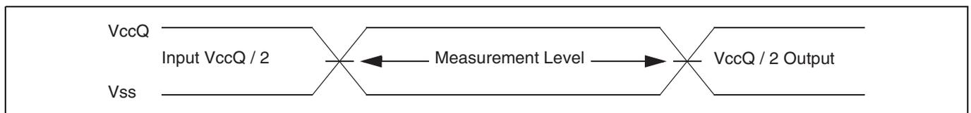
**Figure 34** Input waveforms and measurement levels<sup>[48]</sup>
