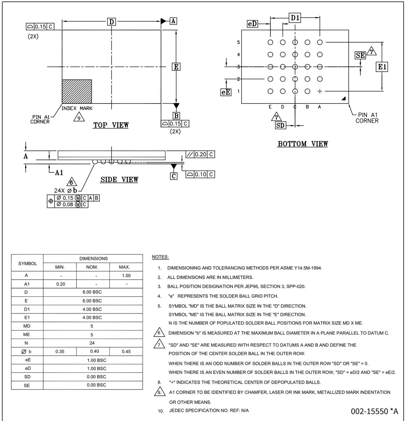
Figure 41 Fortified ball grid array 24-ball 6 × 8 × 1.0 mm (VAA024)
