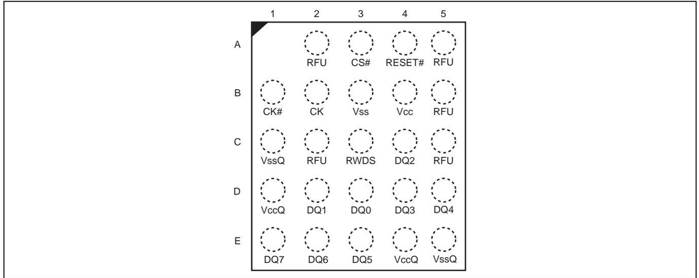
Figure 40 24-ball FBGA, 6 × 8 mm, 5 × 5 ball footprint, Top view
