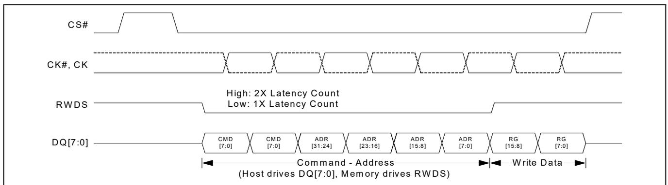
Figure 2 xSPI (Octal) write with no latency transaction (DDR) (Register writes)<sup>[1]</sup>
