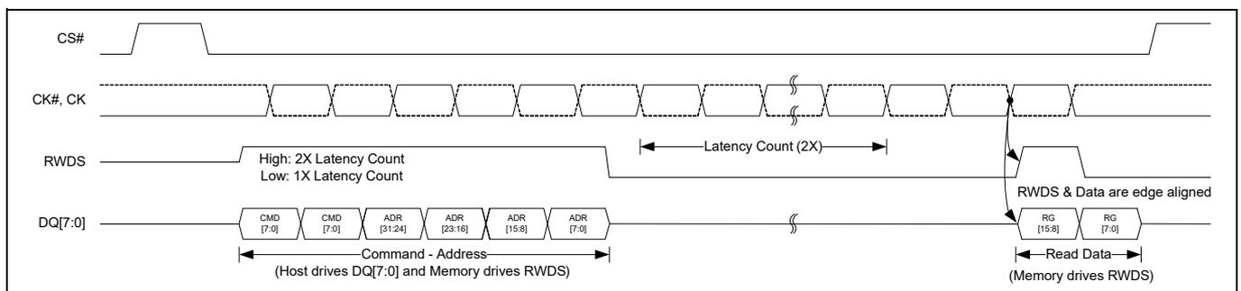
**Figure 20** READ ANY REGISTER with 2X latency transaction (DDR)<sup>[25]</sup>
