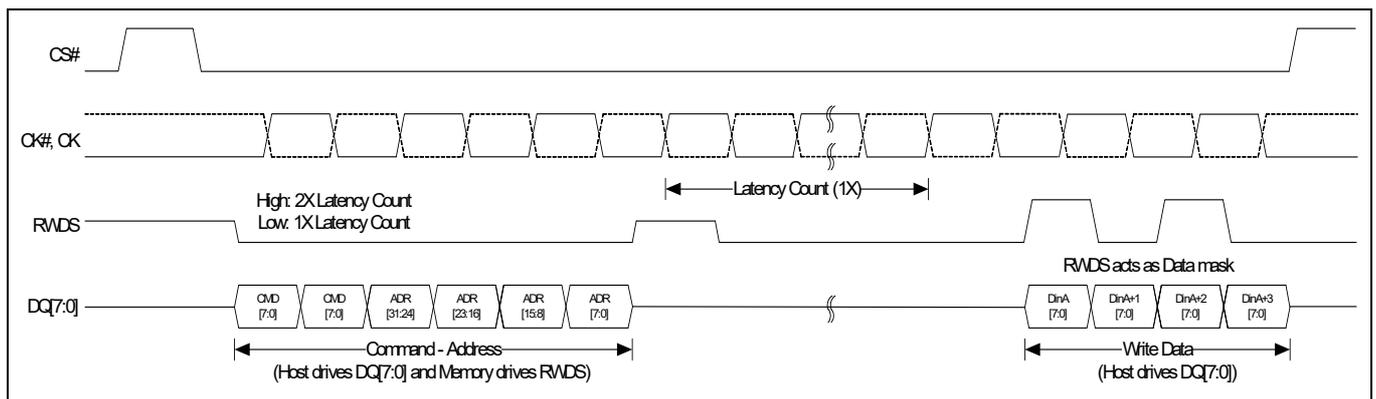
Figure 3 xSPI (Octal) write with 1X latency transaction (DDR) (Memory array writes)<sup>[2, 3]</sup>
