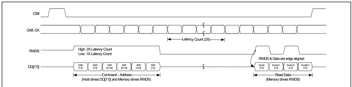
Figure 6 xSPI (Octal) read with 2X latency transaction (DDR) (All reads)<sup>[7]</sup>
