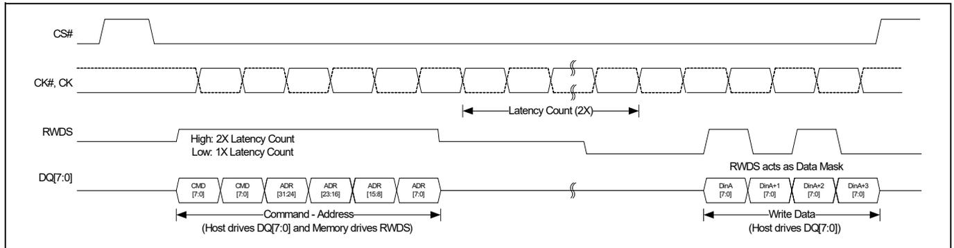
Figure 4 xSPI (Octal) write with 2X latency transaction (DDR) (Memory array writes)<sup>[4, 5]</sup>
