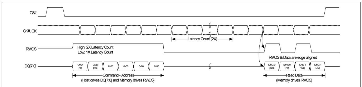
Figure 11 READ ID with 2X latency transaction (DDR)<sup>[17]</sup>
