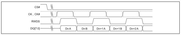
Figure 4-2 Data Placement During a Read Transaction<sup>[12, 13, 14, 15, 16]</sup>
