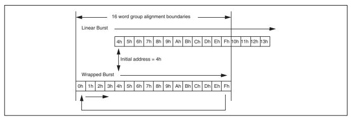
Figure 1-4 Linear Versus Wrapped Burst Sequence
