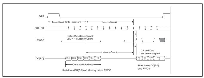
Figure 4-7 Write Transaction Without Additional Initial Latency<sup>[32-36]</sup>
