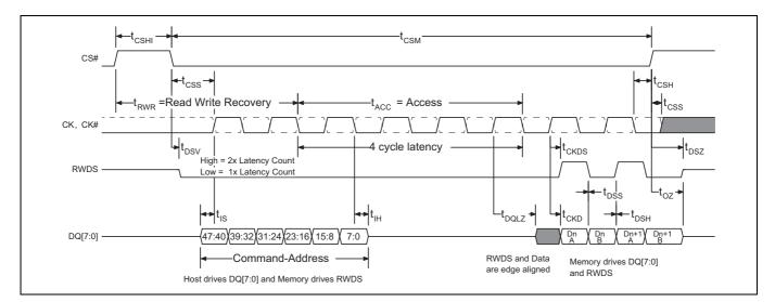
Figure 10-5 Read Timing Diagram – No Additional Latency Required
