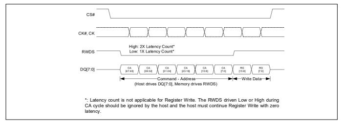
Figure 4-8 Write Operation without Initial Latency
