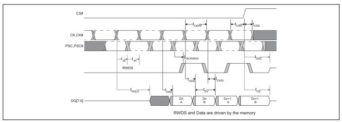
Figure 12-4 DCARS Data Valid Timing<sup>[72, 70, 70]</sup>
