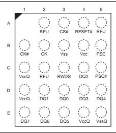
Figure 12-2 24-ball FBGA, 5 × 5 Ball Footprint, Top View
