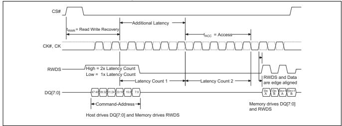
The clock is not required to be free-running. The clock may remain idle while CS# is HIGH.
