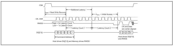
Figure 4-6 Write Transaction with Additional Initial Latency<sup>[30-36]</sup>
