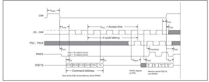
Figure 12-3 HyperRAM Memory DCARS Timing Diagram<sup>[65, 66, 67]</sup>
