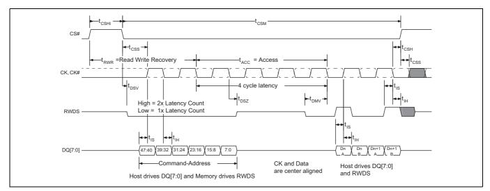
Figure 10-7 Write Timing Diagram – No Additional Latency
