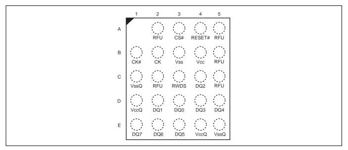
Figure 11-1 24-Ball FBGA, 6 × 8 mm, 5 × 5 Ball Footprint, Top View
