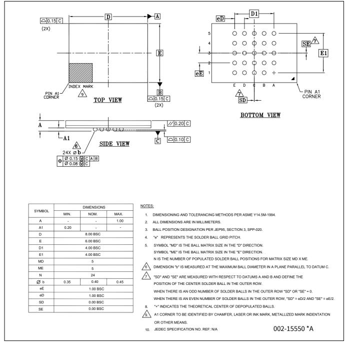
Figure 11-2 Fortified Ball Grid Array 24-ball 6 × 8 × 1.0 mm (VAA024)
