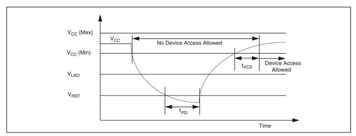
Figure 9-5 Power Down or Voltage Drop
