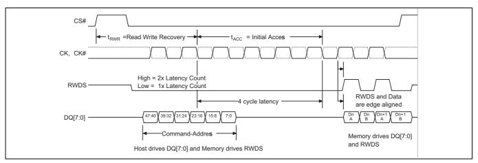
Figure 4-5 Read Transaction Without Additional Initial Latency<sup>[29]</sup>
