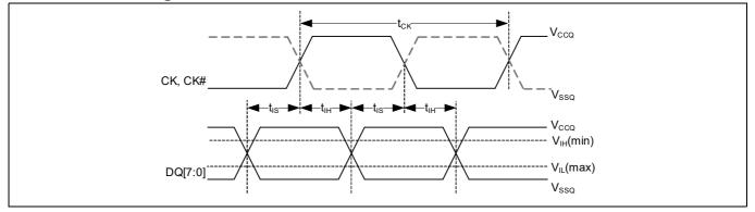
Figure 10-8 DDR Input Timing Reference Levels
