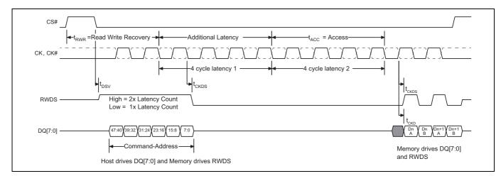
Figure 10-6 Read Timing Diagram – With Additional Latency Required
