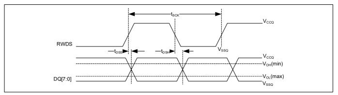
Figure 10-9 DDR Output Timing Reference Levels
