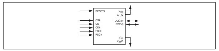
Figure 12-1 HyperBus Product with DCARS Signal Diagram
