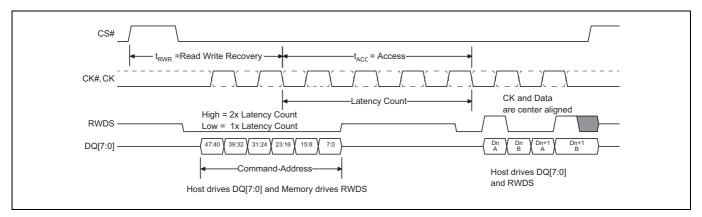
Figure 1-3 Write Transaction, Single Initial Latency Count
