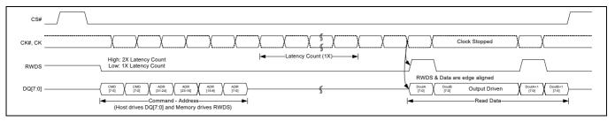
Figure 8-1 Active Clock Stop During Read Transaction (DDR)<sup>[41]</sup>
