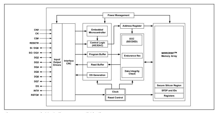
Figure 2 Logic block diagram monolithic die
