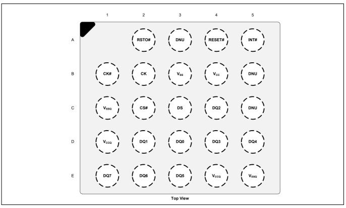
Figure 1 24-ball BGA pinout configuration<sup>[1]</sup>
