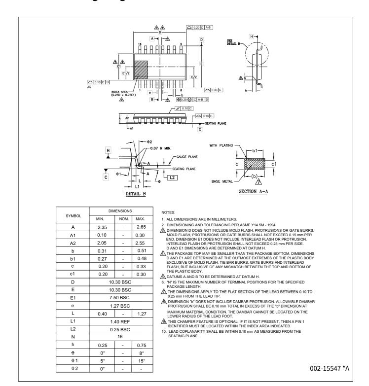
Figure 115 **SOIC 16-lead, 10.30 × 7.50 × 2.65 mm (SO3016) (PG-DSO-16)**
