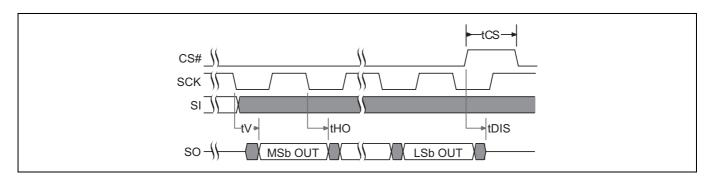
Figure 33 SPI single bit output timing
