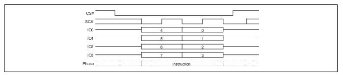
Figure 90 Erase or Program Suspend command sequence QPI mode
