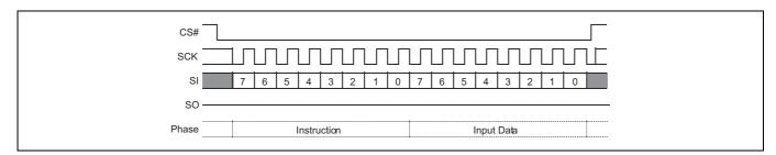
Figure 67 Set Burst Length command sequence
