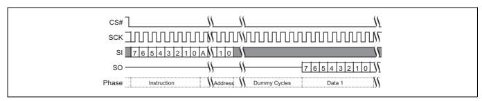
Figure 69 Fast Read (FAST\_READ) command sequence (3-byte address, 0Bh [CR2V[7] = 0)<sup>[52]</sup>
