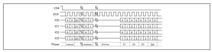
Figure 44 RSFDP QPI mode command sequence
