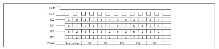
Figure 41 Read Identification (RDID) QPI mode command
