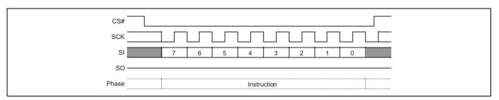
Figure 89 Erase or Program Suspend command sequence
