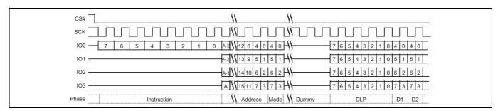
Figure 75 DDR Quad I/O Read Initial Access (EDh or EEh)<sup>[62, 63]</sup>
