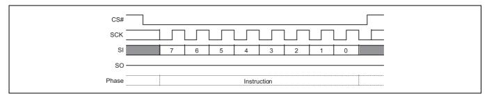
Figure 111 Deep Power-Down command sequence
