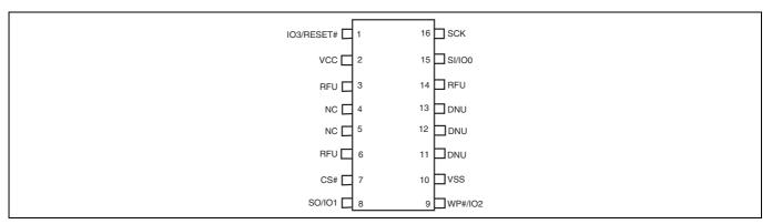
Figure 1 16-lead SOIC package, Top view<sup>[9]</sup>
