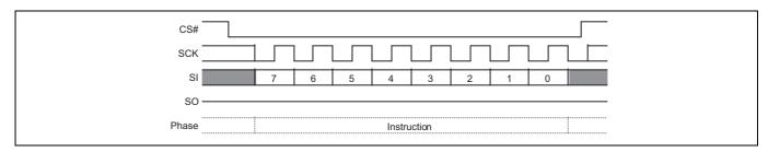
Figure 54 Write Disable (WRDI) command sequence
