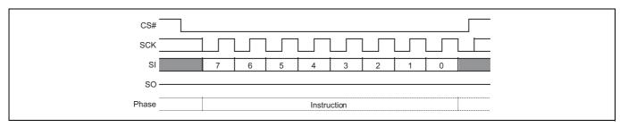
Figure 101 PPB erase command sequence
