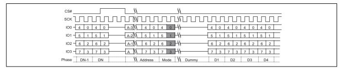
Figure 74 Continuous Quad I/O Read command sequence (EBh or ECh)<sup>[60, 61]</sup>
