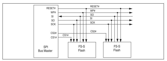
Figure 4 Bus master and memory devices on the SPI bus — single bit data path
