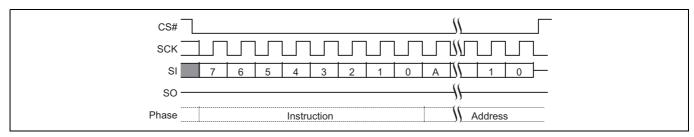
Figure 82 Sector Erase (SE D8h or 4SE DCh) command sequence<sup>[66]</sup>
