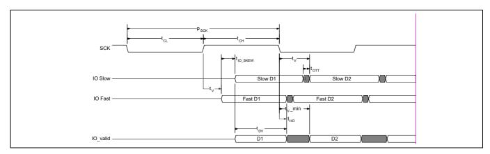
Figure 38 SPI DDR data valid window
