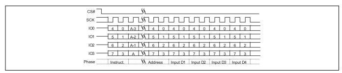
Figure 79 Page Program (PP 02h or 4PP 12h) QPI mode command sequence<sup>[64]</sup>
