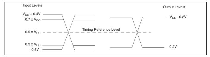
Figure 25 Input, output, and timing reference levels
