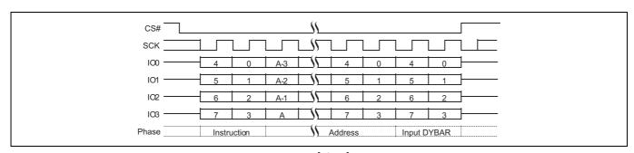
Figure 98 DYBWR QPI mode command sequence<sup>[70, 71]</sup>
