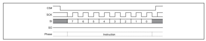
Figure 56 Clear Status Register (CLSR) command sequence
