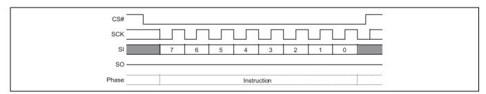
Figure 64 Enter 4-Byte Address mode (4BAM B7h) command sequence
