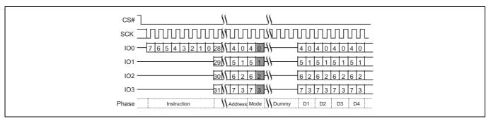
Figure 15 Quad I/O command
