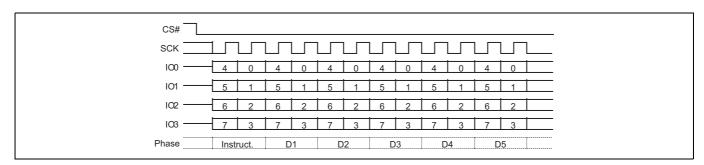
Figure 46 Read Status Register 1 (RDSR1) QPI Mode command
