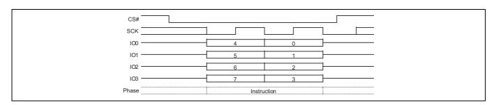
Figure 112 DPD command sequence QPI mode
