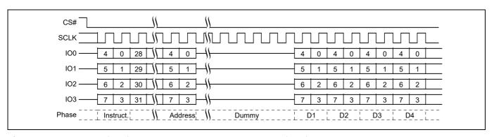
Figure 60 ECCRD (19h), QPI mode, CR2[7] = 1, or 4ECCRD (18h) command sequence
