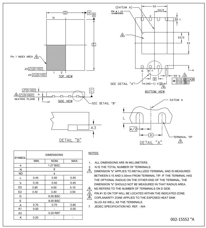
Figure 116 WSON 8-lead DFN  $6.0 \times 8.0 \times 0.8$  mm (WNH008) WNH008  $4.0 \times 3.4$  mm E-Pad (SAWN)(PG-WSON-8)
