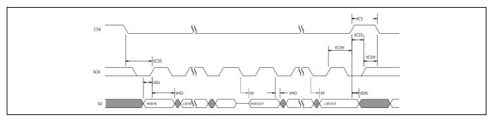
Figure 34 SPI SDR MIO timing
