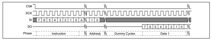
Figure 58 ECC Status Register Read command sequence [48, 49]
