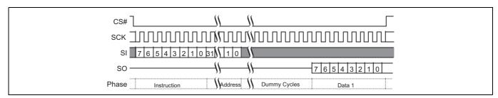
Figure 13 Single Bit Wide I/O command with latency
