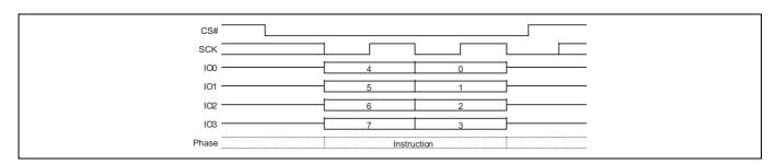
Figure 110 Mode Bit Reset command sequence QPI mode
