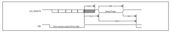
Figure 30 Hardware reset when Quad mode and IO3 / reset# are enabled
