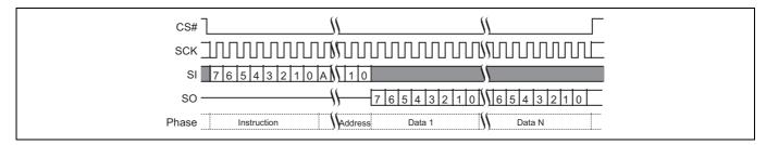
Figure 68 Read command sequence (3-byte address, 03h or 13h)
