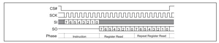
Figure 48 Read Configuration Register (RDCR) command sequence
