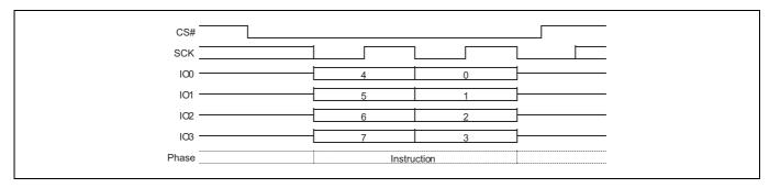
Figure 92 Erase or Program Resume command sequence QPI mode
