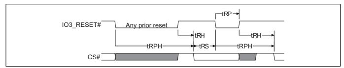
Figure 29 Hardware reset when Quad mode is not enabled and IO3 / reset# is enabled
