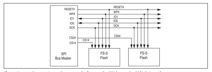
Figure 5 Bus master and memory devices on the SPI bus — dual bit data path
