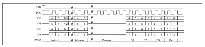
Figure 66 Read Any Register, QPI Mode, command sequence<sup>[50]</sup>
