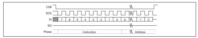
Figure 80 Parameter Sector Erase (P4E 20h or 4P4E 21h) command sequence<sup>[65]</sup>
