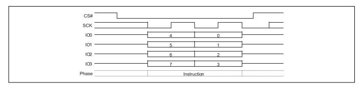
Figure 114 RES command sequence QPI mode
