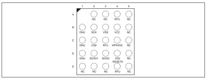
Figure 3 24-ball BGA, 5 x 5 ball footprint (FAB024), top view<sup>[9, 11]</sup>
