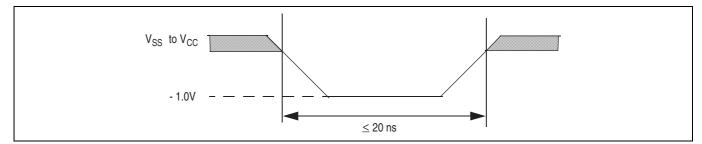
Figure 19 Maximum negative overshoot waveform
