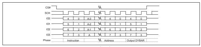
Figure 96 DYBRD QPI mode command sequence [68, 69]
