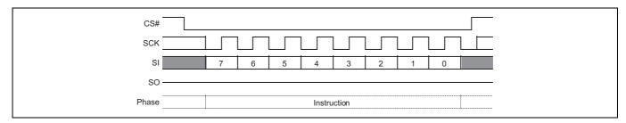
Figure 84 Bulk Erase command sequence
