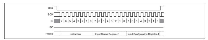
Figure 50 Write Registers (WRR) command sequence – 16 data bits
