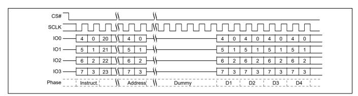
Figure 59 ECCRD (19h), QPI mode, CR2[7] = 0, command sequence
