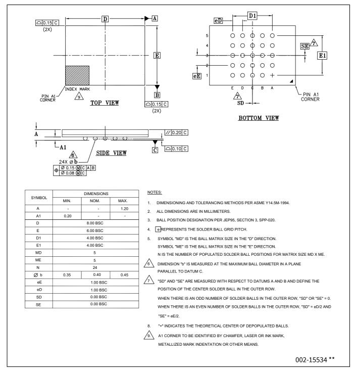
Figure 117 Ball grid array 24-ball FBGA  $8.0 \times 6.0 \times 1.2$  mm (FAB024) (PG-TFBGA-24)
