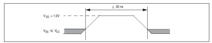
Figure 20 Maximum positive overshoot waveform
