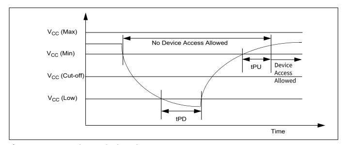
Figure 22 Power-down and voltage drop
