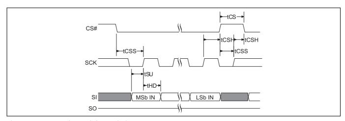
Figure 32 SPI single bit input timing
