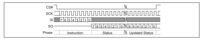
Figure 47 Read Status Register 2 (RDSR2) command
