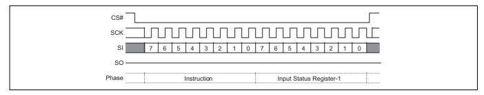
Figure 49 Write Registers (WRR) command sequence – 8 data bits
