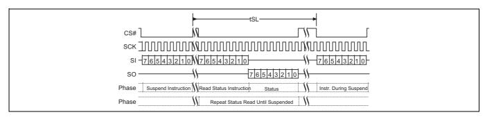
Figure 88 Program or Erase Suspend command sequence
