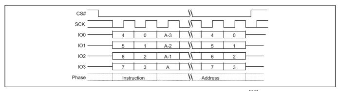
Figure 83 Sector Erase (SE D8h or 4SE DCh) QPI mode command sequence<sup>[66]</sup>
