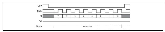
Figure 113 Release from Deep Power-Down command sequence
