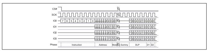
Figure 17 **DDR Quad I/O Read**
