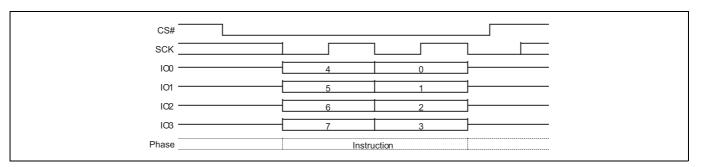
Figure 53 Write Enable (WREN) command sequence QPI mode
