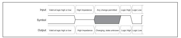
Figure 23 Waveform element meaning
