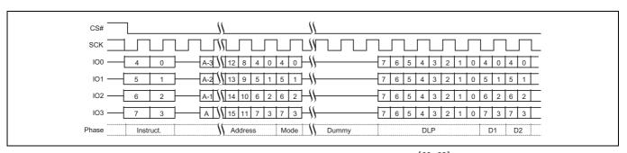
Figure 77 DDR Quad I/O Read Initial Access (EDh or EEh), QPI mode [62, 63]
