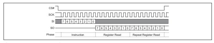
Figure 102 PPB Lock Register Read command sequence
