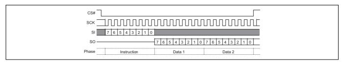
Figure 11 Single Bit Wide Output command
