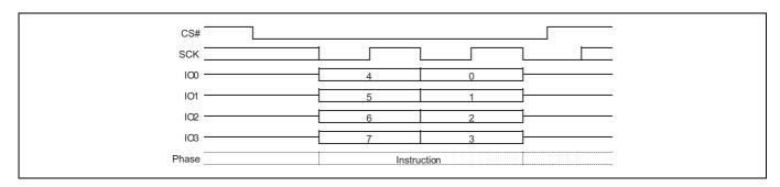
Figure 55 Write Disable (WRDI) command sequence QPI mode
