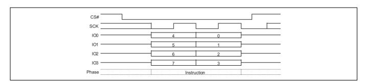
Figure 108 Software Reset command sequence QPI mode
