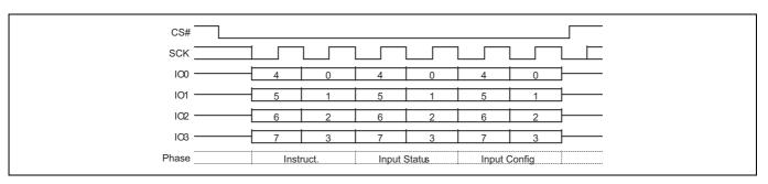
Figure 51 Write Registers (WRR) command sequence – 16 data bits QPI mode
