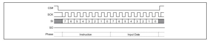
Figure 62 Write VDLR (WVDLR) command sequence
