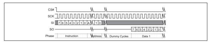
Figure 65 Read Any Register Read command sequence<sup>[50]</sup>
