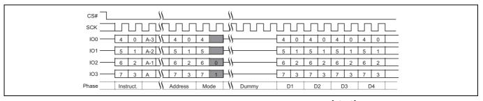
Figure 73 Quad I/O Read command sequence (EBh or ECh), QPI Mode<sup>[58, 59]</sup>
