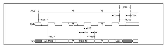
Figure 36 **SPI DDR input timing**
