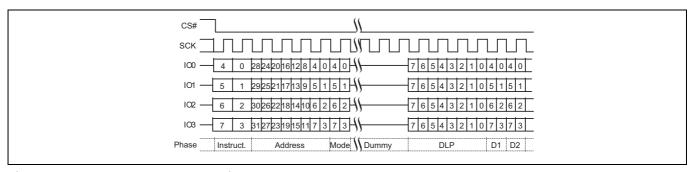
Figure 18 DDR Quad I/O Read in QPI mode
