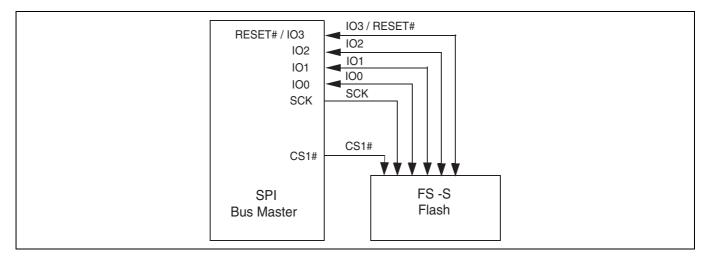
Figure 6 Bus master and memory devices on the SPI bus — quad bit data path
