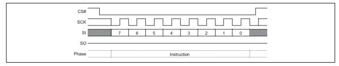
Figure 52 Write Enable (WREN) command sequence
