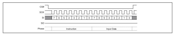
Figure 61 Program NVDLR (PNVDLR) command sequence
