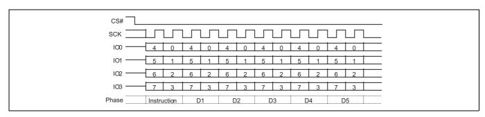
Figure 42 Read Quad Identification (RDQID) command sequence
