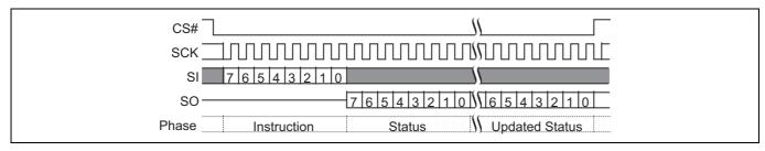
Figure 45 Read Status Register 1 (RDSR1) command sequence
