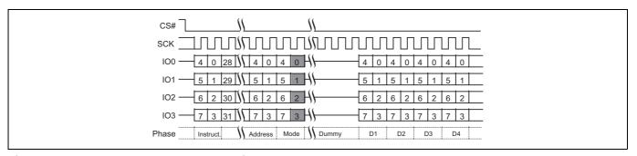
Figure 16 Quad I/O Read command in QPI mode
