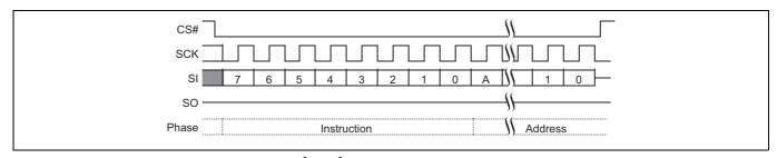
Figure 100 PPBP command sequence<sup>[74, 75]</sup>
