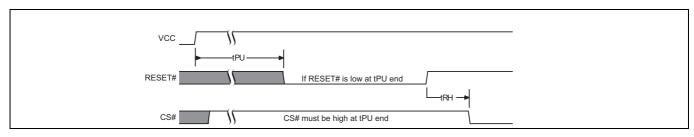
Figure 26 Reset LOW at the end of POR
