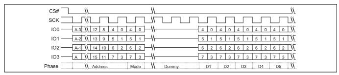
Figure 76 Continuous DDR Quad I/O Read Subsequent Access (EDh or EEh)[62, 63]
