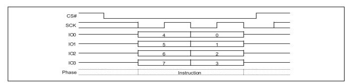
Figure 57 Clear Status Register (CLSR) command sequence QPI mode
