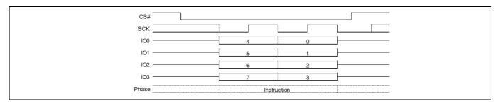
Figure 85 Bulk Erase command sequence QPI mode
