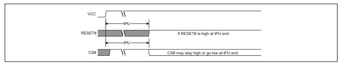
Figure 27 Reset HIGH at the end of POR
