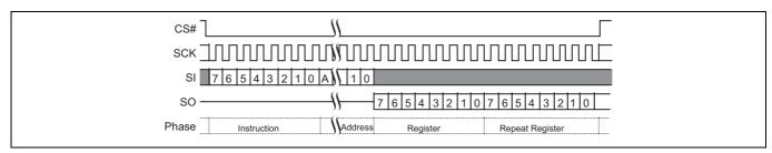
Figure 99 PPBRD command sequence<sup>[72, 73]</sup>
