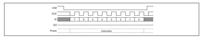
Figure 103 PPB Lock Bit Write command sequence
