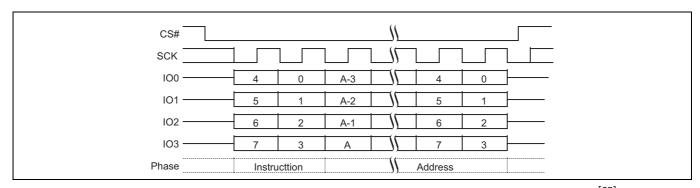
Figure 81 Parameter Sector Erase (P4E 20h or 4P4E 21h) QPI mode command sequence<sup>[65]</sup>
