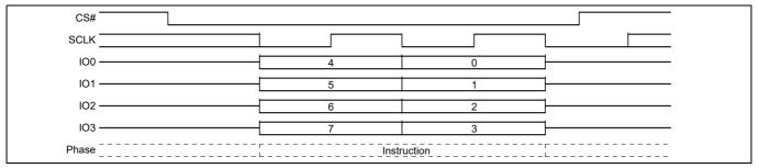
Figure 92 Bulk Erase Command sequence QPI mode
