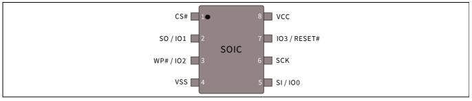
Figure 1 8-pin plastic small outline package (SOIC8)
