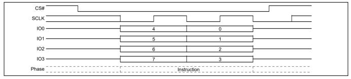
Figure 96 Program or Erase Suspend command sequence QPI mode
