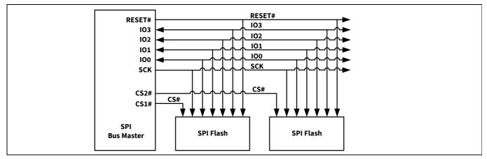
Figure 6 Bus master and memory devices on the SPI bus - Quad bit data path - Separate RESET#
