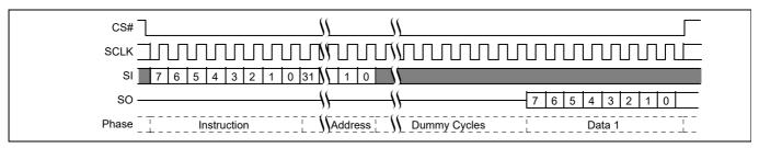
Figure 13 Single Bit Wide I/O command with latency
