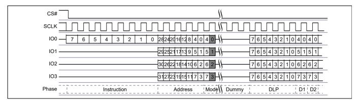
Figure 19 DDR Quad I/O Read command<sup>[7]</sup>
