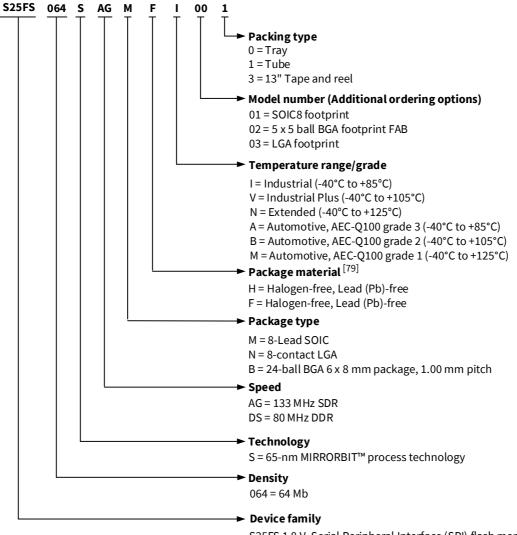
S25FS 1.8 V, Serial Peripheral Interface (SPI) flash memory
