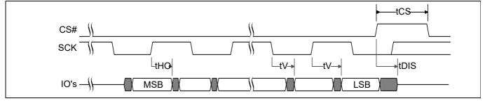
Figure 36 SPI DDR output timing
