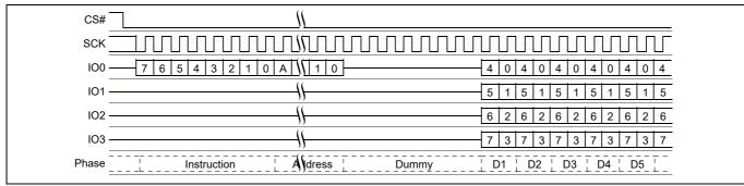
Figure 75 Quad Output Read command sequence<sup>[45]</sup>
