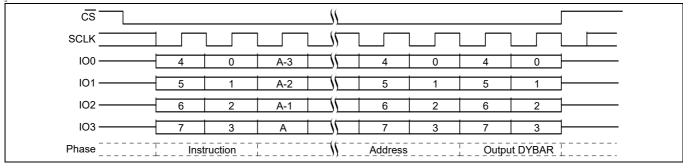
Figure 103 DYBRD QPI mode command sequence<sup>[58, 60]</sup>
