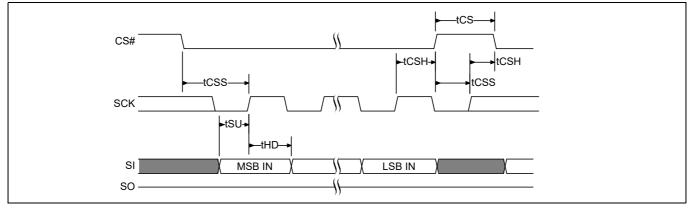
Figure 31 SPI single bit input timing
