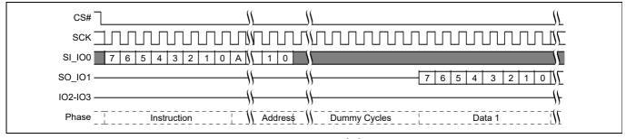
Figure 73 Fast Read (FAST\_READ) command sequence<sup>[43]</sup>
