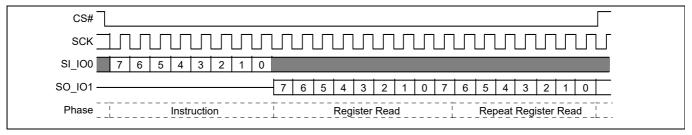
Figure 109 PPB Lock Register command sequence
