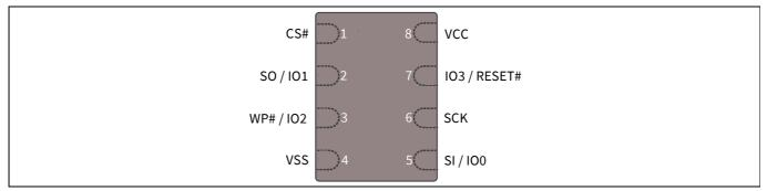
Figure 2 8-pad LGA 5 × 6 (W9A008), top view<sup>[4]</sup>
