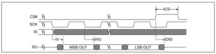
Figure 32 SPI single bit output timing
