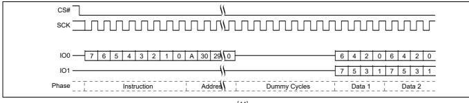
Figure 74 Dual Output Read command sequence<sup>[44]</sup>
