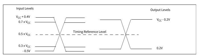
Figure 23 Input, output, and timing reference levels
