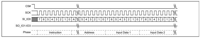
Figure 104 DYB Write command sequence<sup>[61, 62]</sup>
