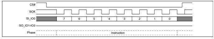
Figure 118 Release from Deep Power Down (RES) command sequence
