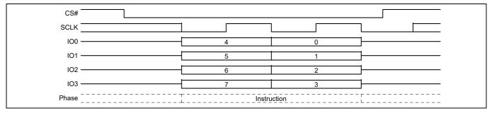
Figure 119 Release from Deep Power Down (RES) command sequence – QPI mode
