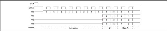
Figure 43 Read Quad Identification (RDQID) command sequence Quad mode
