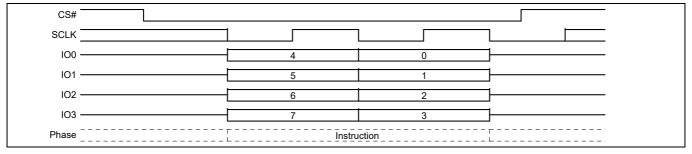
Figure 115 Software reset/mode bit command sequence – QPI mode
