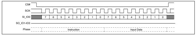
Figure 64 Write VDLR (WVDLR) command sequence
