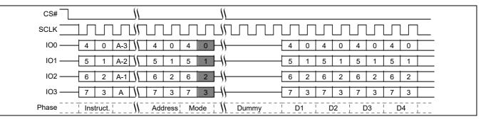
Figure 79 Quad I/O Read Initial Access command sequence QPI mode<sup>[48]</sup>
