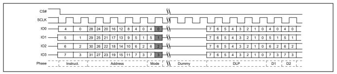
Figure 20 DDR Quad I/O Read command QPI mode<sup>[7]</sup>
