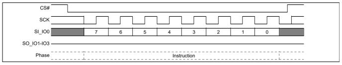
Figure 110 PPB Lock Bit command sequence
