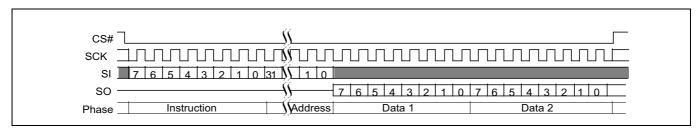
Figure 10 Single bit wide I/O command without latency
