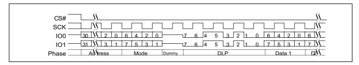
Figure 88 Continuous DDR dual I/O read subsequent access (4-byte address, EHPLC= 01b)
