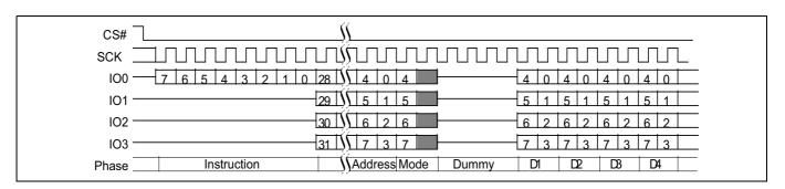
Figure 15 Quad I/O command
