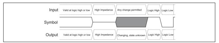
Figure 23 Waveform element meanings
