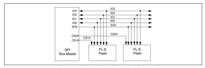
Figure 4 Bus master and memory devices on the SPI bus — Quad bit data path
