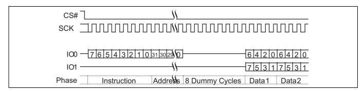
Figure 70 Dual output read command sequence (4-byte address, 3Ch or 3Bh [ExtAdd=1, LC=10b])
