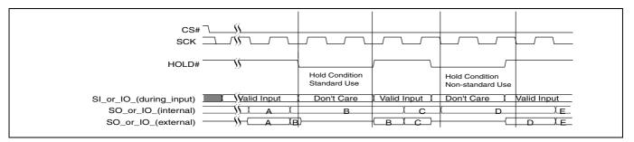
Figure 1 HOLD mode operation
