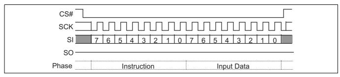
Figure 64 Write VDLR (WVDLR 4Ah) command sequence
