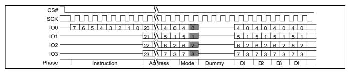
Figure 78 Quad I/O read command sequence (3-byte address, EBh [ExtAdd=0], LC=00b)
