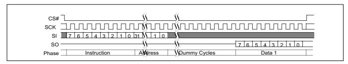
Figure 11 Single bit wide I/O command with latency
