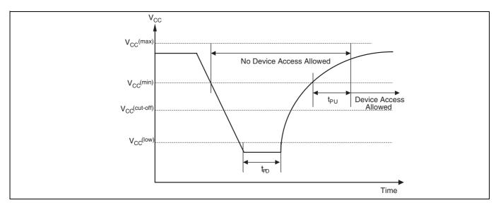
Figure 22 Power-down and voltage drop
