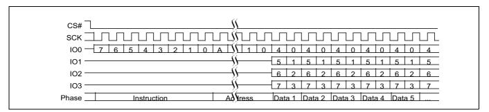
Figure 95 Quad 512-byte page program command sequence
