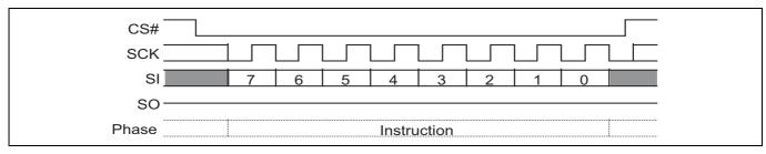
Figure 55 Write enable (WREN 06h) command sequence
