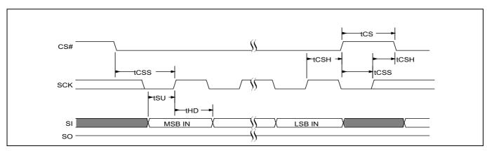
SPI single bit input timing Figure 31
