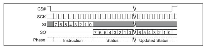
Figure 47 Read status register-1 (RDSR1 05h) command sequence
