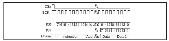
Figure 71 Dual output read command sequence (4-byte address, 3Ch or 3Bh [ExtAdd=1, LC=11b])
