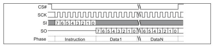
Figure 61 AutoBoot register read (ABRD 14h) Command
