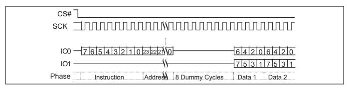
Figure 69 Dual output read command sequence (3-byte address, 3Bh [ExtAdd=0], LC=10b)
