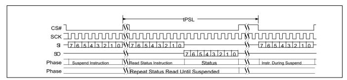
Figure 96 Program suspend (PGSP 85h) command sequence
