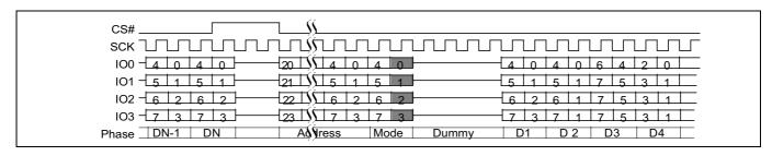
Figure 79 Continuous quad I/O read command sequence (3-byte address), LC=00b
