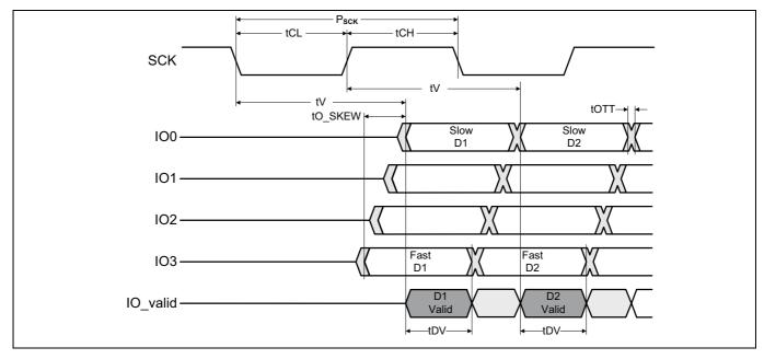
Figure 38 SPI DDR data valid window
