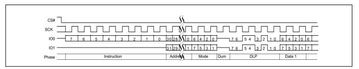
Figure 17 DDR dual I/O read with EHPLC = 01b and DLP
