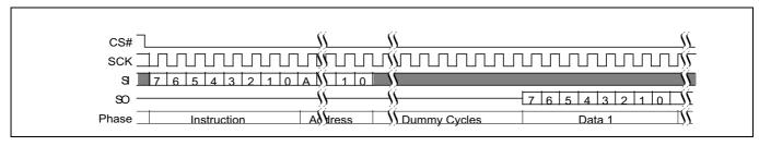
Figure 67 Fast read (FAST\_READ 0Bh or 0Ch) command sequence with read latency
