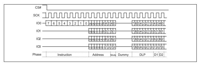
Figure 18 DDR quad I/O read
