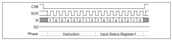
Figure 53 Write registers (WRR 01h) command sequence - 8 data bits
