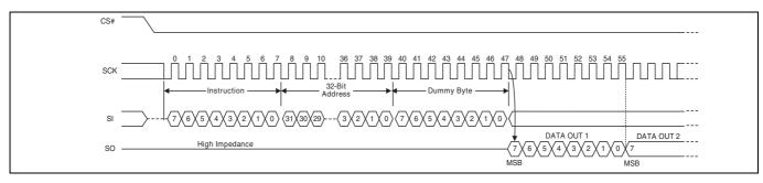
Figure 58 ECC status register read command sequence
