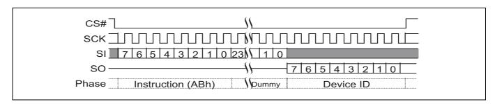
Figure 45 Read electronic signature (RES ABh) command sequence
