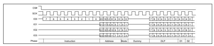
Figure 90 DDR quad I/O read initial access (3-byte address, EDh [ExtAdd=0], HPLC=11b)
