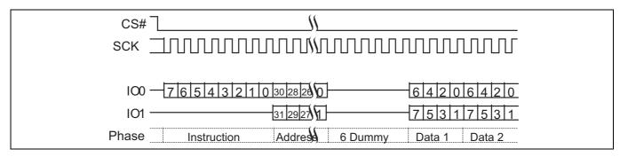
Figure 75 Dual I/O read command sequence (4-byte address, BBh [ExtAdd=1], HPLC=10b)
