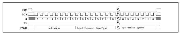
Figure 115 Password unlock (PASSU E9h) command sequence
