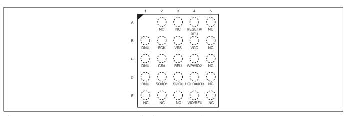
Figure 39 24-ball BGA, 5 x 5 ball footprint (FAB024), top view
