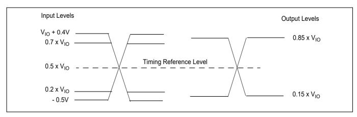
Figure 24 Input, output, and timing reference levels
