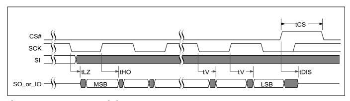
Figure 37 SPI DDR output timing
