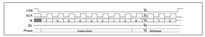
Figure 98 Sector erase (SE D8h or 4SE DCh) command sequence
