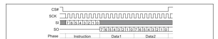
Figure 9 Single bit wide output command
