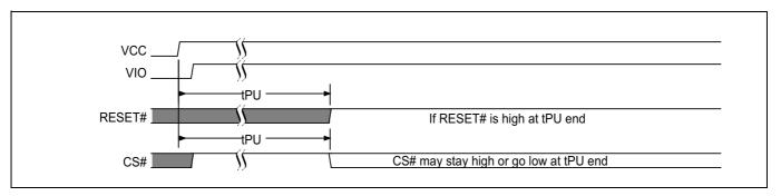
Figure 27 Reset high at the end of POR
