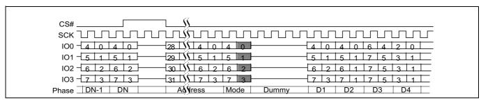
Figure 81 Continuous quad I/O read command sequence (4-byte address), LC=00b
