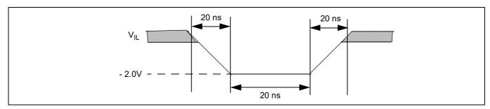
Figure 19 **Maximum negative overshoot waveform**
