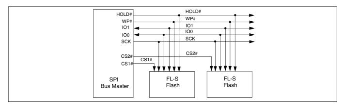
Figure 3 Bus master and memory devices on the SPI bus — Dual bit data path
