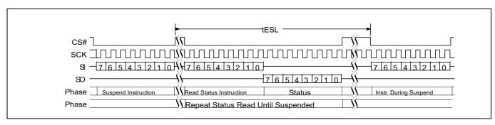
Figure 100 Erase suspend (ERSP 75h) command sequence
