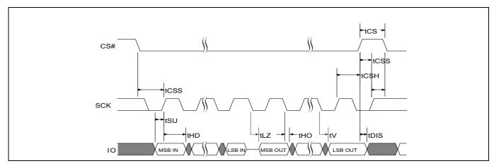
Figure 33 SPI SDR MIO timing
