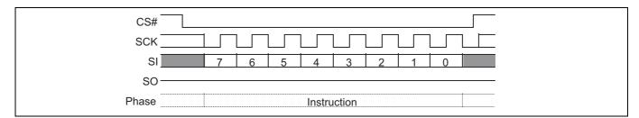
Figure 97 10.55 Program resume (PGRS 8Ah) command sequence
