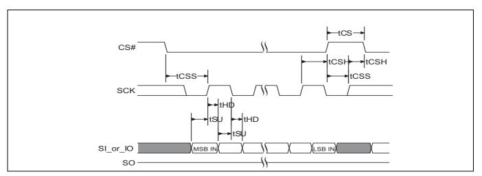
Figure 36 SPI DDR input timing
