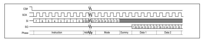
Figure 16 DDR fast read with EHPLC = 00b
