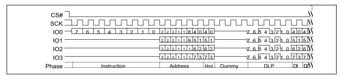
Figure 92 DDR quad I/O read initial access (4-byte address, EEh or EDh [ExtAdd=1], EHPLC=01b)<sup>[44]</sup>
