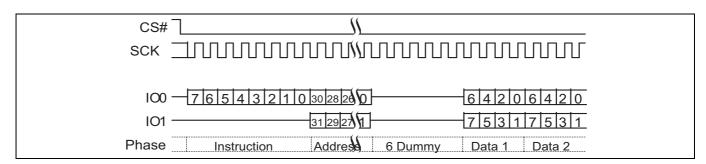
Figure 12 **Dual output command**
