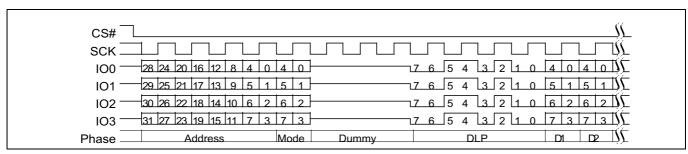
Figure 93 Continuous DDR quad I/O read subsequent access (4-byte address, EHPLC=01b)<sup>[44]</sup>
