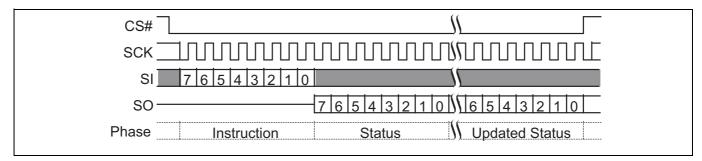
Figure 48 Read status register-2 (RDSR2 07h) command sequence
