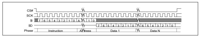
Figure 66 Read command sequence (READ 03h or 13h)
