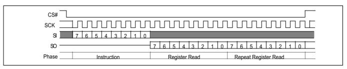
Figure 49 Read configuration register (RDCR 35h) command sequence
