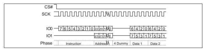
Figure 74 Dual I/O read command sequence (3-byte address, BBh [ExtAdd=0], HPLC=00b)
