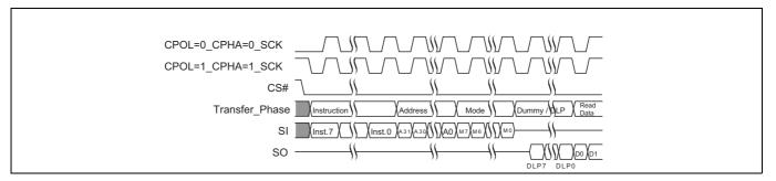
Figure 6 SPI DDR modes supported
