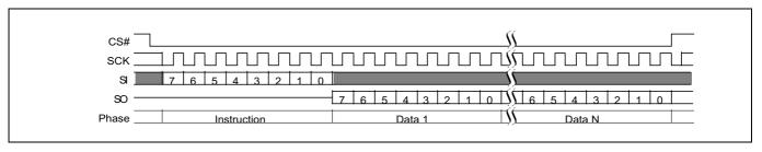
Figure 44 Read identification (RDID 9Fh) command sequence
