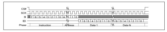
Figure 68 Fast read command (FAST\_READ 0Bh or 0Ch) sequence without read latency
