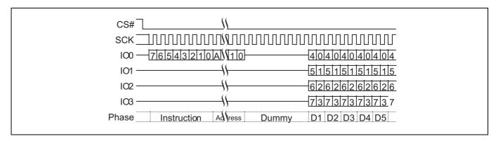
Figure 72 Quad output read (QOR 6Bh or 4QOR 6Ch) command sequence with read latency
