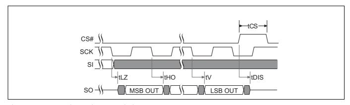
Figure 32 SPI single bit output timing
