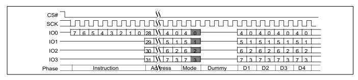
Figure 80 Quad I/O read command sequence(4-byte address, ECh or EBh [ExtAdd=1], LC=00b)
