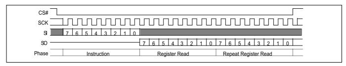
Figure 111 PPB lock register read command sequence
