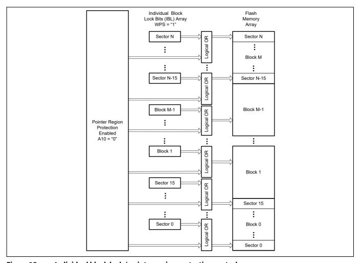
Figure 25 Individual block lock / pointer region protection control
