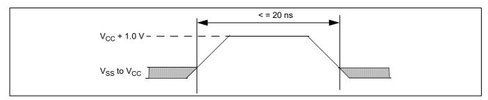
Figure 130 Maximum positive overshoot waveform
