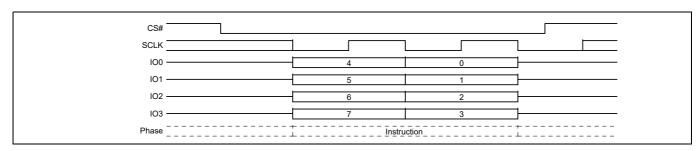
Figure 87 Chip Erase command sequence QPI mode
