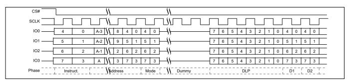
Figure 23 DDR Quad I/O Read command QPI mode
