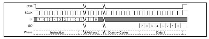
Figure 16 Single Bit Wide I/O command with latency
