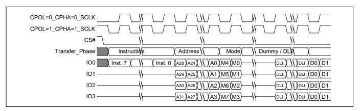
Figure 12 SPI DDR modes supported
