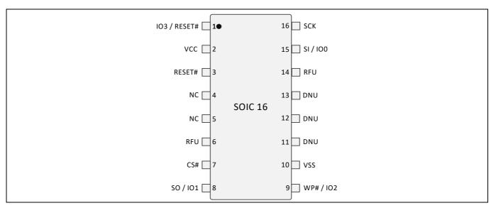
Figure 1 16-lead SOIC package (SO3016), top view
