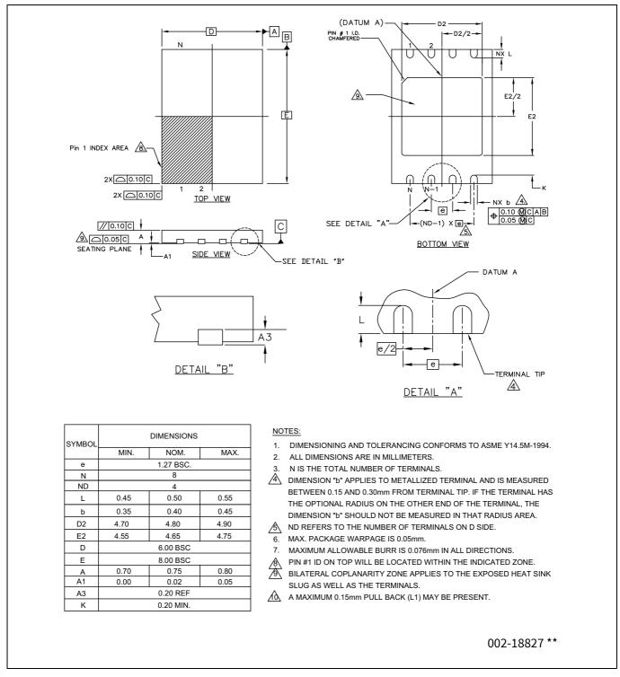
Figure 153 8-lead DFN ((6 × 8 × 0.8 mm) 4.80 × 4.65 mm E-Pad (Sawn)) package outline (PG-WSON-8), 002-18827
