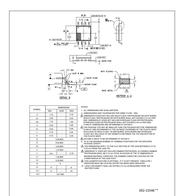
Figure 151 8-lead SOIC (5.28 × 5.28 × 2.16 mm) package outline (PG-DSO-8), 002-15548
