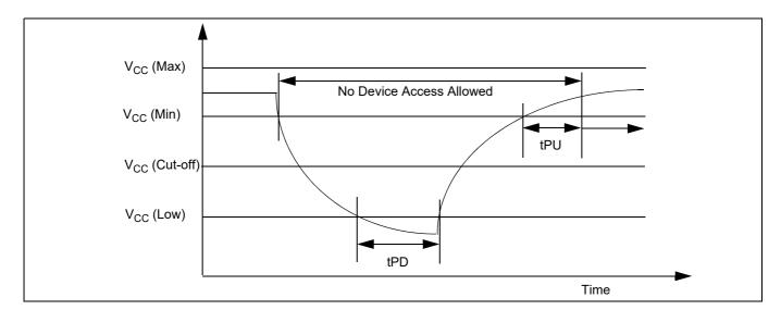
Figure 132 Power-down and voltage drop
