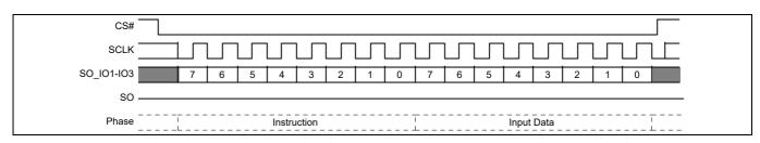
Figure 14 **Single Bit Wide Input command**
