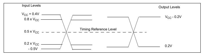
Figure 135 Input, output, and timing reference levels
