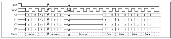
Figure 60 Read Any Register, QPI mode, command sequence<sup>[31]</sup>
