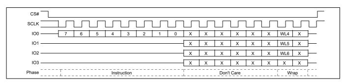
Figure 61 Set Burst Length command sequence quad I/O mode
