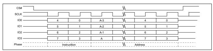
Figure 81 Sector Erase (SE 20h or 4SE 21h) QPI mode command sequence<sup>[46]</sup>
