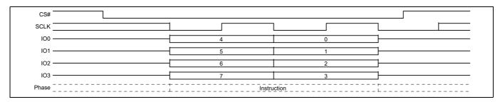
Figure 42 Write Enable (WREN) command sequence QPI mode
