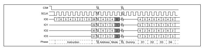
Figure 20 Quad I/O command<sup>[8]</sup>
