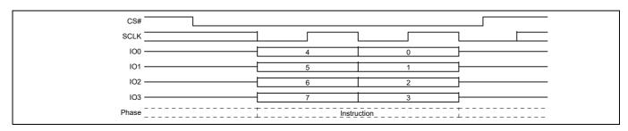
Figure 122 Software reset / Mode Bit command sequence - QPI mode
