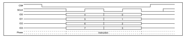
Figure 44 Write Disable (WRDI) command sequence QPI mode
