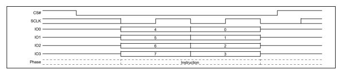
Figure 58 Exit 4 Byte Address QPI mode
