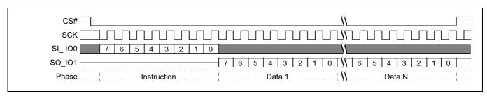
Figure 27 Read Identification (RDID) command sequence
