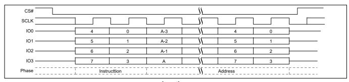
Figure 98 IBL command sequence QPI mode<sup>[55, 56]</sup>
