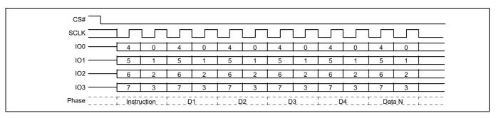
Figure 28 Read Identification (RDID) QPI mode command
