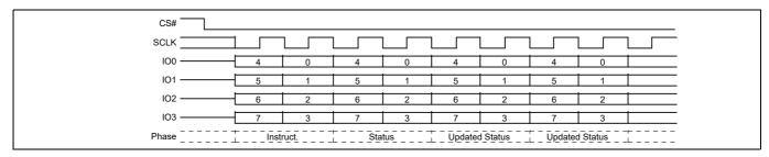
Figure 36 Read Status Register 1 (RDSR1) QPI Mode Command
