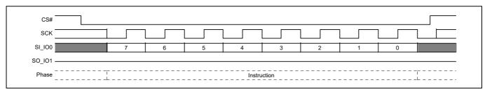
Figure 86 Chip Erase command sequence
