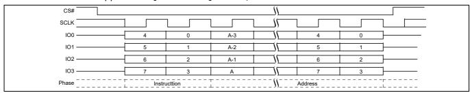
Figure 106 SPRP command sequence QPI mode<sup>[59, 60]</sup>
