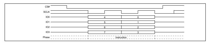
Figure 92 Erase or Program Resume command sequence QPI mode
