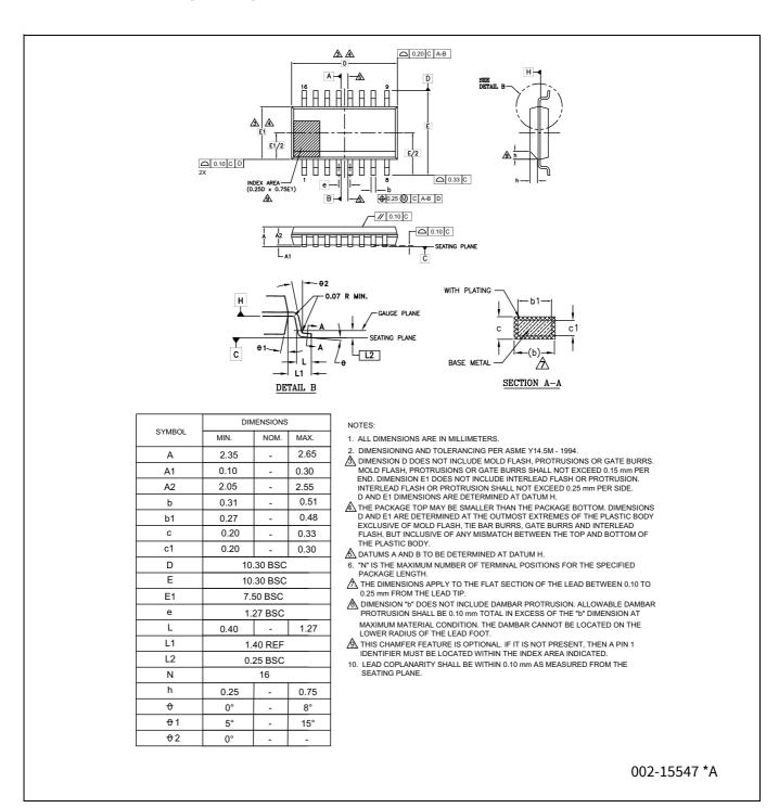
Figure 150 16-lead SOIC (10.30 × 7.50 × 2.65 mm) package outline (PG-DSO-16), 002-15547
