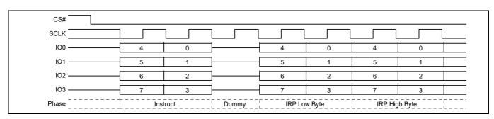
Figure 108 IRPRD command sequence - QPI mode
