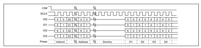
Figure 32 RSFDP QPI mode command sequence
