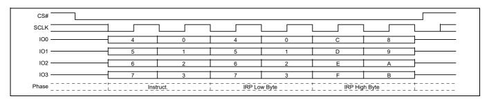
Figure 110 IRP Program (IRPP) command QPI
