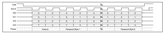
Figure 118 Password Program (PASSP) command sequence QPI mode
