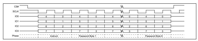
Figure 120 Password Unlock (PASSU) command sequence QPI mode
