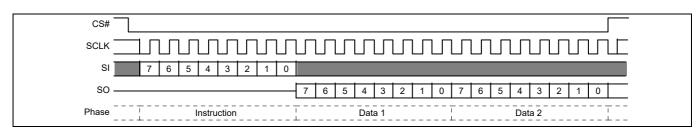
Figure 15 **Single Bit Wide Output command without latency**
