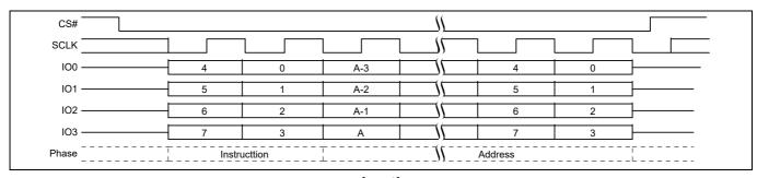
Figure 100 IBUL command sequence QPI mode<sup>[57, 58]</sup>
