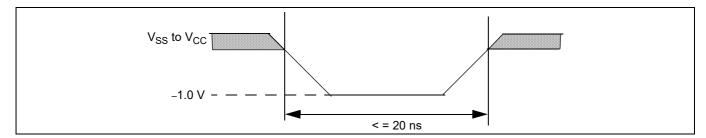
Figure 129 Maximum negative overshoot waveform
