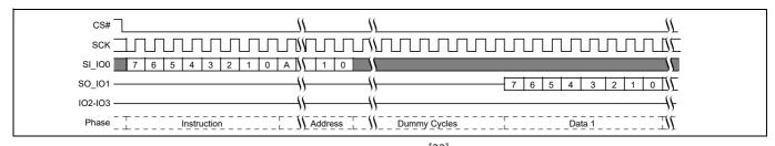
Figure 66 Fast Read (FAST\_READ) command sequence<sup>[33]</sup>
