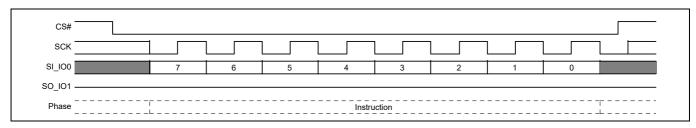
Figure 125 Release from Deep Power Down (RES) command sequence
