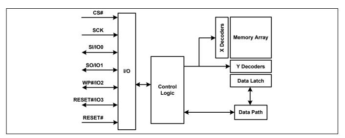
Figure 6 Logic block diagram
