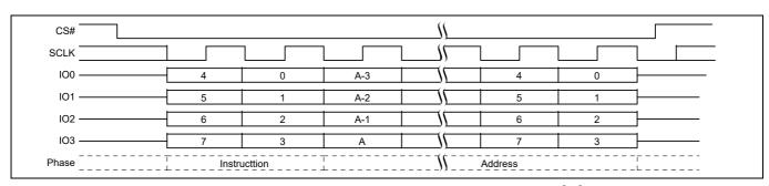
Figure 85 Block Erase (BE D8h or 4BE DCh) QPI mode command sequence [49]
