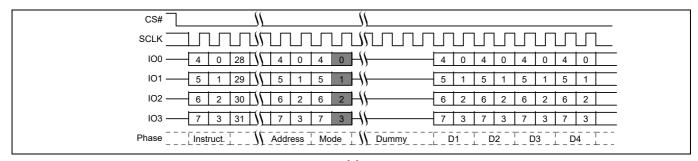
Figure 21 Quad I/O Read command in QPI mode<sup>[8]</sup>
