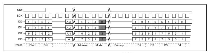
Figure 73 Continuous Quad I/O Read command sequence<sup>[38, 39]</sup>
