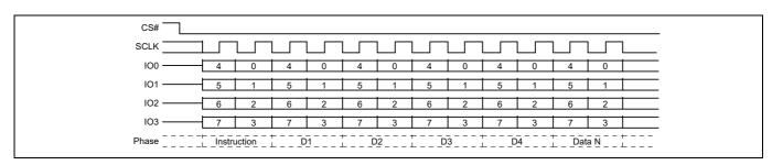
Figure 29 Read Quad Identification (RDQID) command sequence QPI mode
