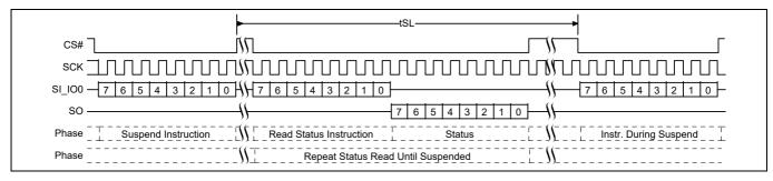
Figure 90 Program or Erase Suspend command with continuing instruction commands sequence
