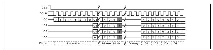
Figure 71 Quad I/O Read initial access command sequence<sup>[38]</sup>
