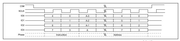
Figure 83 Half Block Erase (HBE 52h or 4HBE 53h) QPI mode command sequence<sup>[47, 48]</sup>
