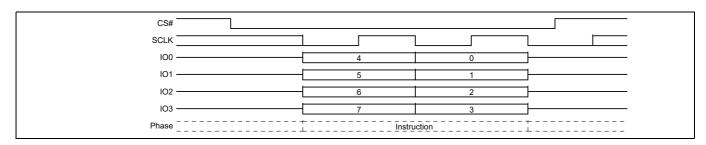
Figure 64 Exit QPI (QPIEX F5h) command sequence
