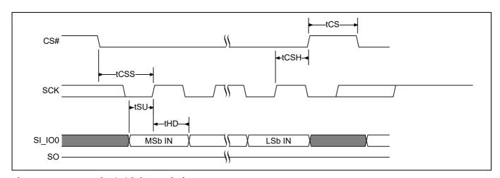
Figure 143 SPI single bit input timing
