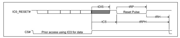
Figure 141 Hardware reset when quad or QPI mode and IO3 / RESET# are enabled
