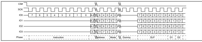
Figure 74 DDR Quad I/O Read initial access [40, 42]
