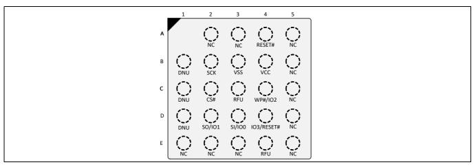
Figure 4 24-ball BGA, 5 x 5 ball footprint (FAB024), top view
