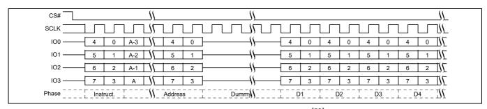
Figure 94 Security Regions Read command sequence QPI mode<sup>[52]</sup>
