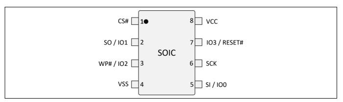
Figure 2 8-Pin plastic small outline package (SOIC8)
