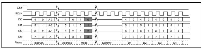
Figure 72 Quad I/O Read initial access command sequence QPI mode<sup>[38]</sup>
