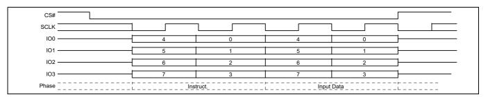
Figure 50 Program DLRNV (PDLRNV) command sequence - QPI mode
