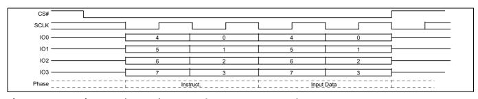
Figure 52 Write DLRV (WDLRV) command sequence - QPI mode
