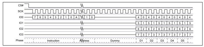
Figure 68 Quad Output Read command sequence<sup>[35]</sup>
