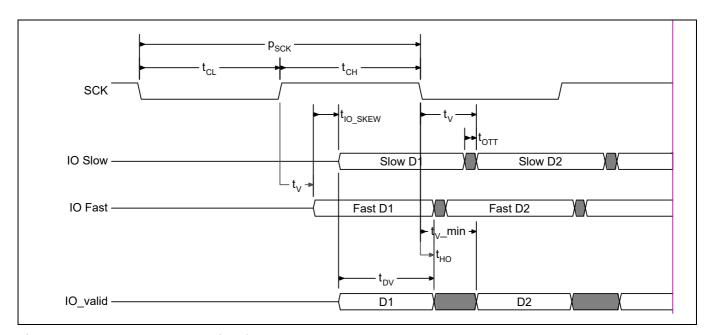
Figure 149 SPI DDR data valid window
