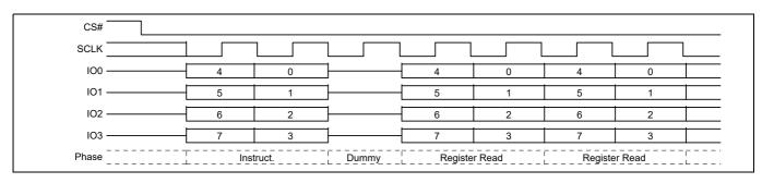
Figure 54 DLP Read (DLPRD) command sequence – QPI mode
