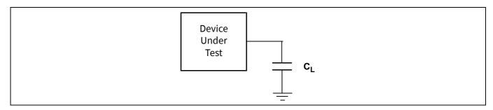
Figure 134 Test setup
