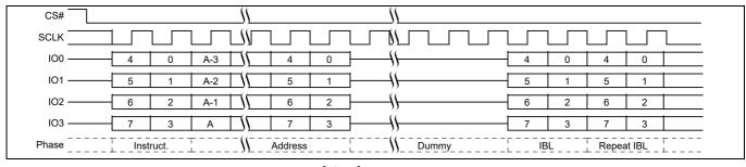
Figure 96 IBLRD command sequence QPI<sup>[53, 54]</sup>
