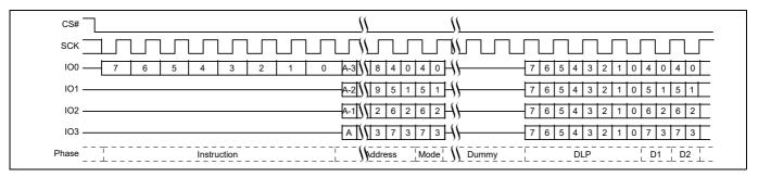
Figure 22 DDR Quad I/O Read command
