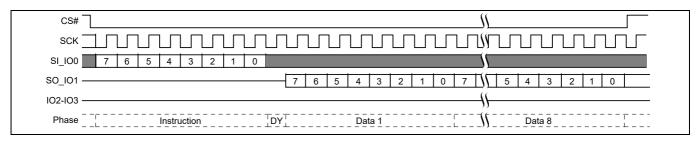
Figure 115 Password Read (PASSRD) command sequence
