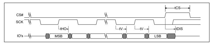
Figure 148 SPI DDR output timing
