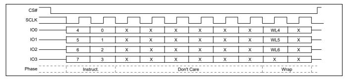
Figure 62 Set Burst Length command sequence QPI mode
