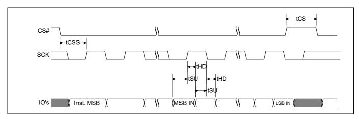
Figure 147 SPI DDR input timing
