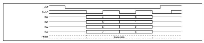
Figure 89 Program or Erase Suspend command sequence QPI mode
