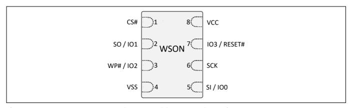
Figure 3 8-Connector package (WSON 6 x 8) (WSON 5 x 6), top view
