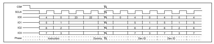
Figure 128 Read Identification (RES) QPI mode command
