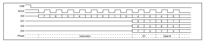
Figure 30 Read Quad Identification (RDQID) command sequence quad mode
