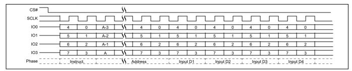
Figure 78 Page Program (PP 02h or 4PP 12h) QPI mode command sequence<sup>[44]</sup>
