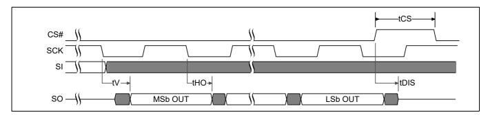
Figure 144 SPI single bit output timing
