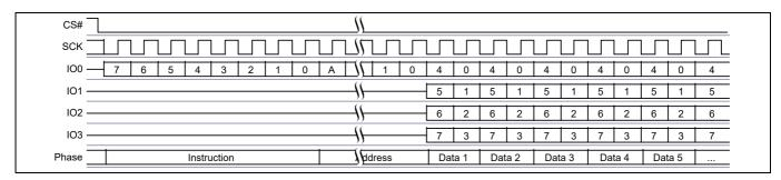
Figure 79 Quad page program command sequence<sup>[45]</sup>
