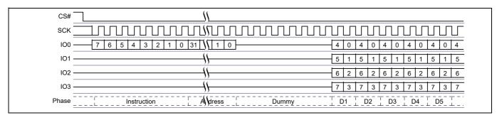
Figure 18 Quad Output Read command
