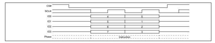
Figure 124 Deep Power Down (DPD) command sequence – QPI mode
