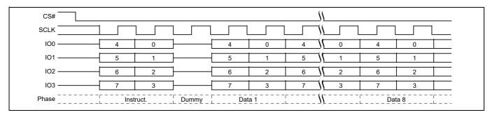
Figure 116 Password Read (PASSRD) command sequence – QPI mode
