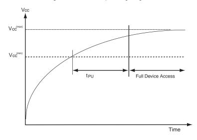
Figure 11.1 Power-Up Timing Diagram
