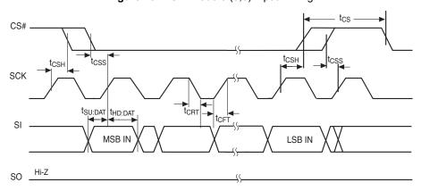
Figure 18.2 SPI Mode 0 (0,0) Input Timing
