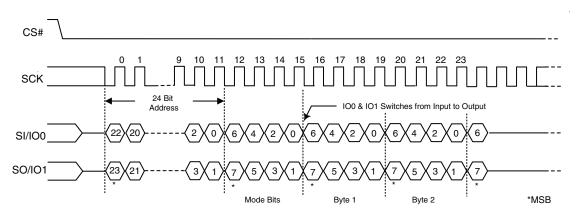
Figure 9.6 Continuous Dual I/O High Performance Read Instruction Sequence
