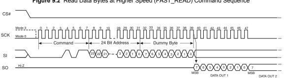
Figure 9.2 Read Data Bytes at Higher Speed (FAST READ) Command Sequence
