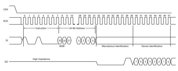
Figure 9.10 Read-ID (RDID) Command Timing Diagram
