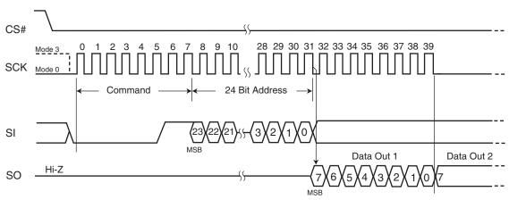
Figure 9.1 Read Data Bytes (READ) Command Sequence
