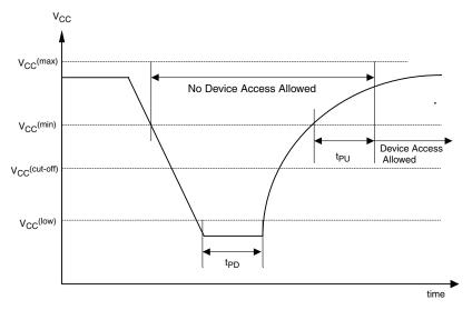
Figure 11.2 Power-down and Voltage Drop
