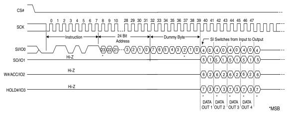
Figure 9.4 Quad Output Read Instruction Sequence
