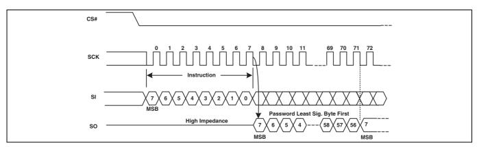
Figure 102 Password Read command sequence
