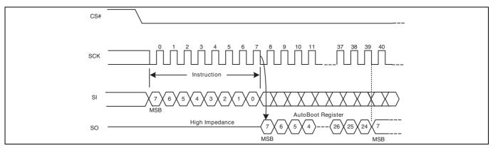
Figure 65 AutoBoot Register Read (ABRD) command
