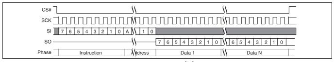
Figure 67 Read command sequence (READ 03h or 13h)<sup>[36]</sup>
