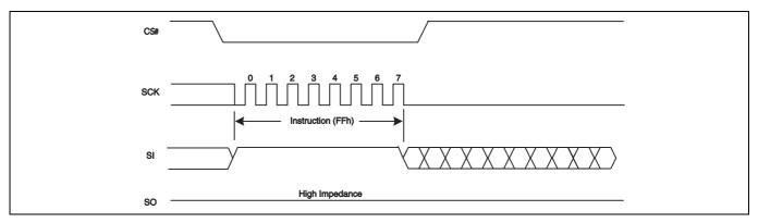
Figure 106 Mode Bit Reset command sequence
