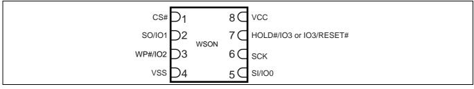
Figure 38 8-Contact WSON 6 x 5 mm, top view<sup>[29, 30]</sup>
