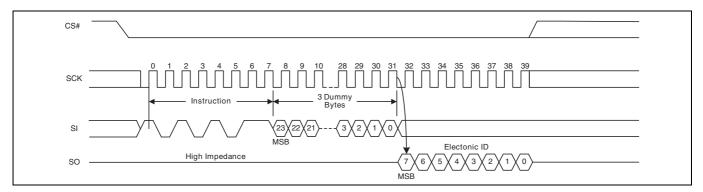
Figure 48 Read Electronic Signature (RES) command sequence
