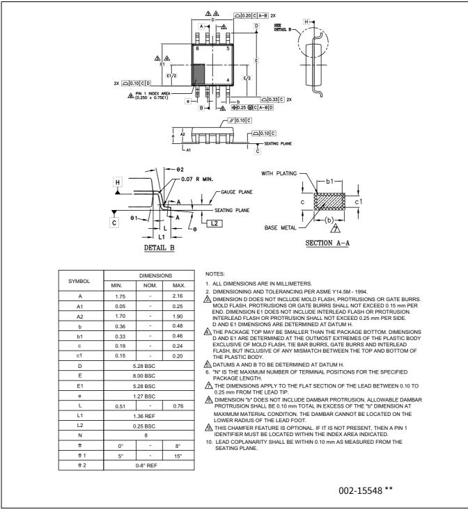
Figure 35 8-lead SOIC (5.28 × 5.28 × 2.16 mm) package outline, 002-15548
