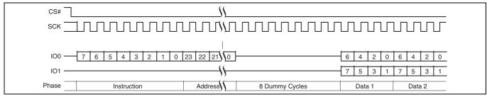
Figure 70 Dual Output Read command sequence (3-byte address, 3Bh [ExtAdd = 0], LC = 10b)
