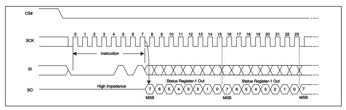
Figure 50 Read Status Register 1 (RDSR1) command sequence
