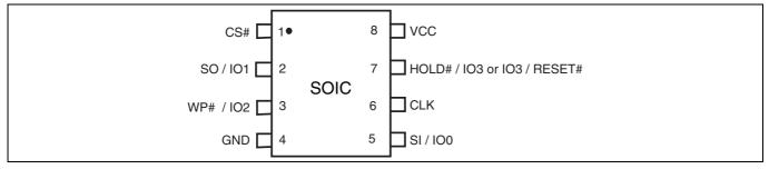
Figure 34 8-pin plastic small outline package (SO)<sup>[28]</sup>
