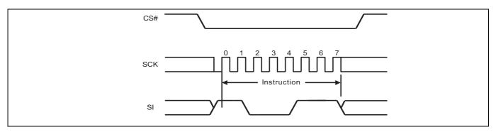
Figure 88 Bulk Erase command sequence
