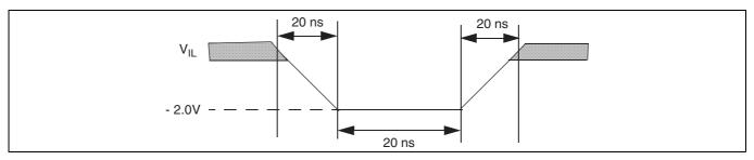
Figure 15 Maximum negative overshoot waveform
