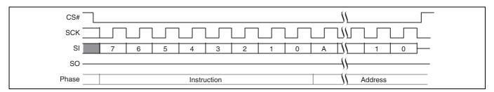
Figure 86 Parameter Sector Erase (P4E 20h or 4P4E 21h) command sequence<sup>[42]</sup>
