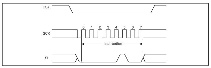
Figure 60 Write Disable (WRDI) command sequence
