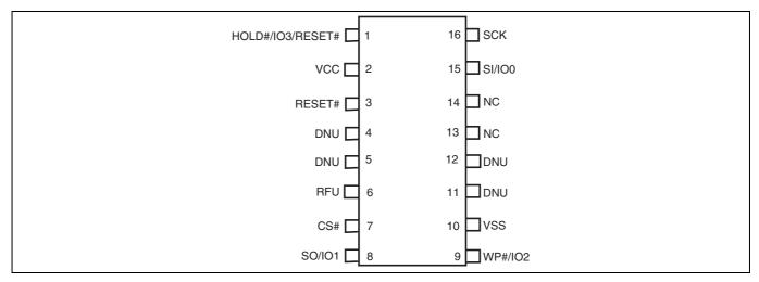
Figure 36 16-lead SOIC package, top view
