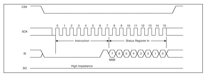
Figure 56 Write Registers (WRR) command sequence – 8 data bits
