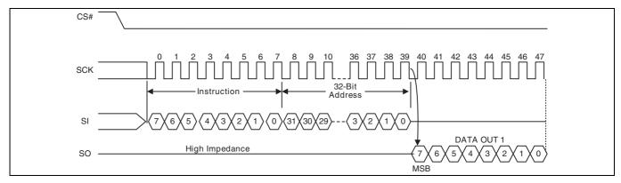
Figure 97 PPBRD command sequence
