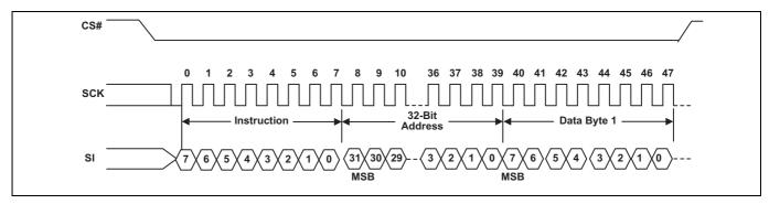
Figure 96 DYBWR command sequence
