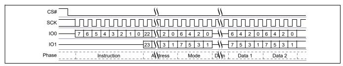
Figure 75 Dual I/O Read command sequence (3-byte address, BBh [ExtAdd = 0])
