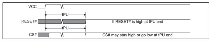
Figure 23 Reset HIGH at the end of POR
