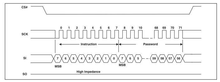
Figure 104 Password Unlock command sequence
