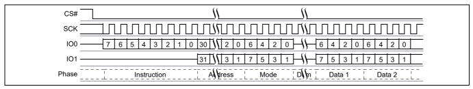
Figure 76 Dual I/O Read command sequence (4-byte address, BCh or BBh [ExtAdd = 1])<sup>[40]</sup>
