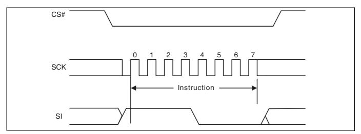
Figure 105 Software Reset command sequence
