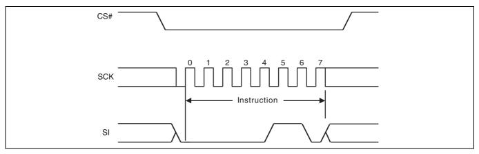
Figure 59 Write Enable (WREN) command sequence
