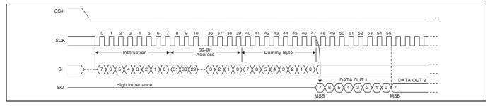
Figure 62 ECC Status Register Read command sequence
