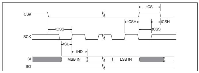
Figure 29 SPI single bit input timing
