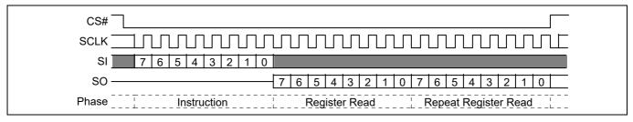
Figure 52 Read Configuration Register (RDCR) command sequence
