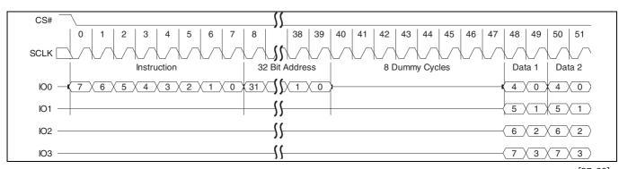
Figure 74 Quad Output Read (QOR 6Bh or 4QOR 6Ch) command sequence without read latency<sup>[37, 39]</sup>
