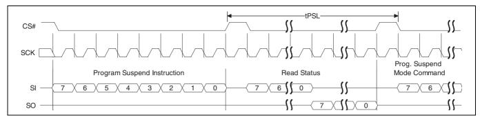
Figure 84 Program Suspend command sequence
