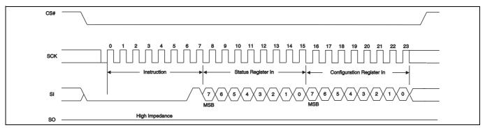
Figure 57 Write Registers (WRR) command sequence – 16 data bits
