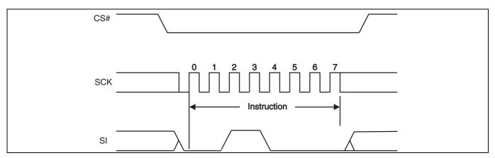
Figure 61 Clear Status Register (CLSR) command sequence
