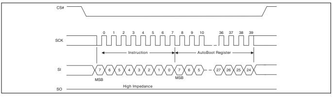
Figure 66 AutoBoot Register Write (ABWR) command
