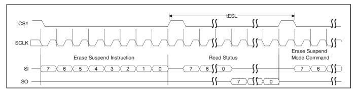
Figure 89 Erase Suspend command sequence
