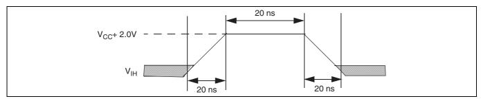
Figure 16 Maximum positive overshoot waveform
