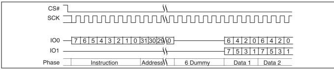
Figure 11 Dual Output command
