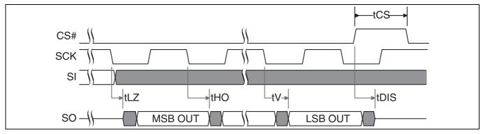
Figure 30 SPI single bit output timing
