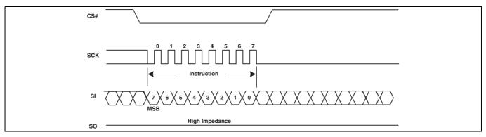
Figure 101 PPB Lock Bit Write command sequence
