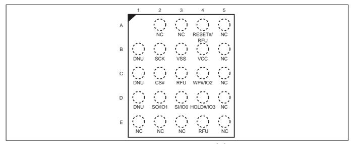
Figure 4024-ball BGA, 5 x 5 ball footprint (FAB024), top view
