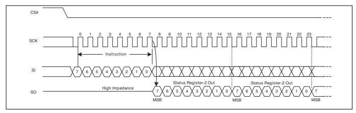
Figure 51 Read Status Register 2 (RDSR2) command
