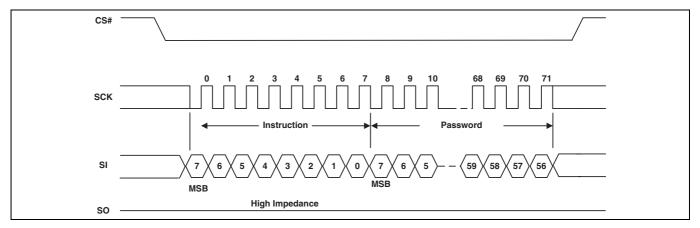
Figure 103 Password Program command sequence
