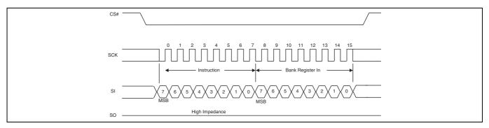
Figure 54 Bank Register Write (BRWR) command
