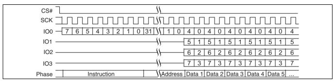
Figure 12 Quad Output command without latency
