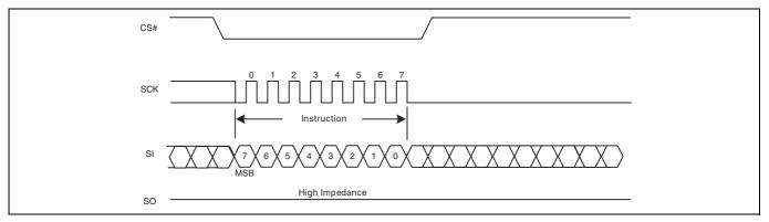
Figure 99 PPB Erase command sequence
