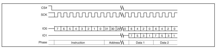
Figure 72 Dual Output Read command sequence (4-byte address, 3Ch or 3Bh [ExtAdd = 1, LC = 11b])
