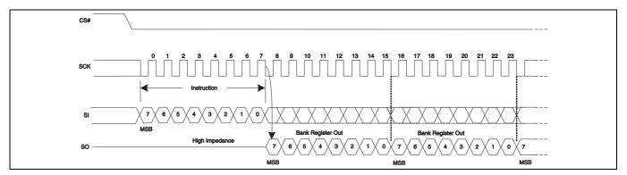
Figure 53 Read Bank Register (BRRD) command
