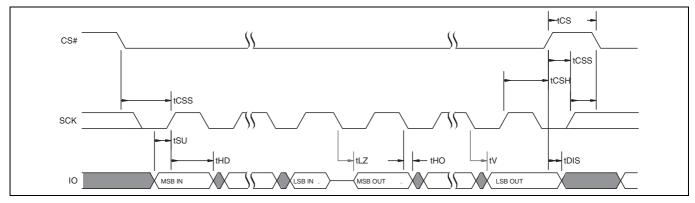
Figure 31 SPI MIO timing
