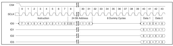
Figure 73 Quad Output Read (QOR 6Bh or 4QOR 6Ch) command sequence with read latency<sup>[37, 38]</sup>
