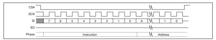
Figure 87 Sector Erase (SE D8h or 4SE DCh) command sequence<sup>[43]</sup>
