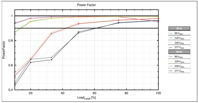
Figure 7 ICL8810 PFC-PSR-flyback reference design power factor
