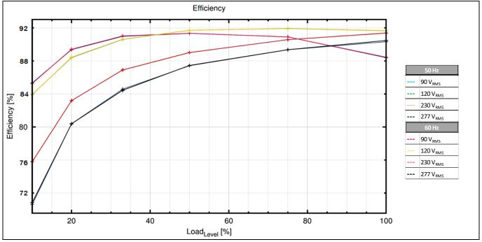
Figure 6 ICL8810 PFC-PSR-flyback reference design efficiency
