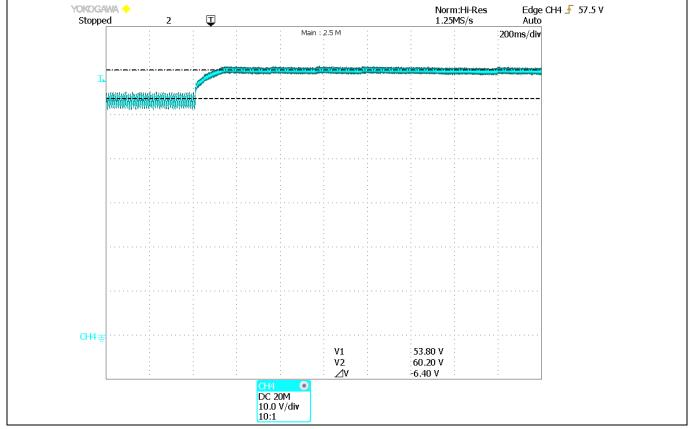
Figure 12 ICL8810 PFC-PSR-flyback reference design IC reaction to immediate output power jump from 100 percent to 0 percent with OVP
