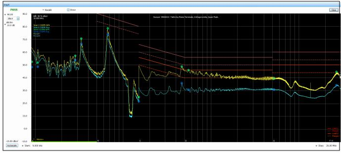
Figure 13ICL8810 PFC-PSR-flyback reference design EMC pre-compliance report. Input voltage<br/>120 V<sub>AC</sub>, 60 Hz, output power 42 W
