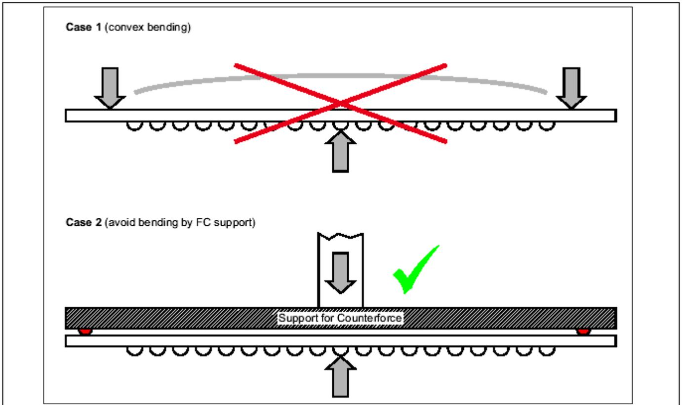
Figure 8 Case 1 shows bending stress applied on Wafer-Level Package by insufficient support. Case 2 shows a nozzle supporting the package and applying a counterforce.
