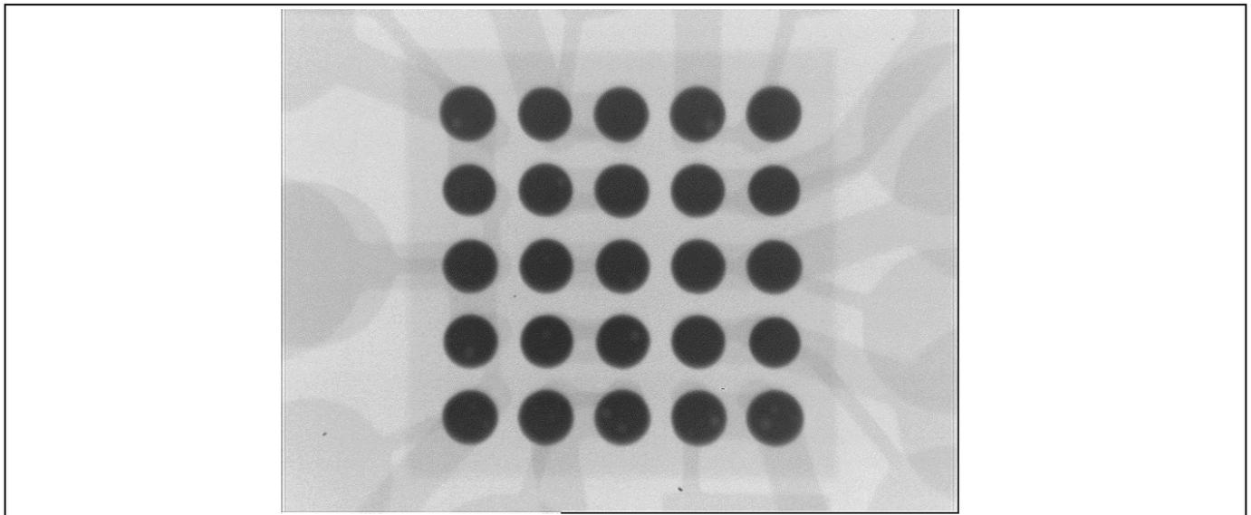
Figure 10 Example of an X-Ray image of an Infineon WLB package
