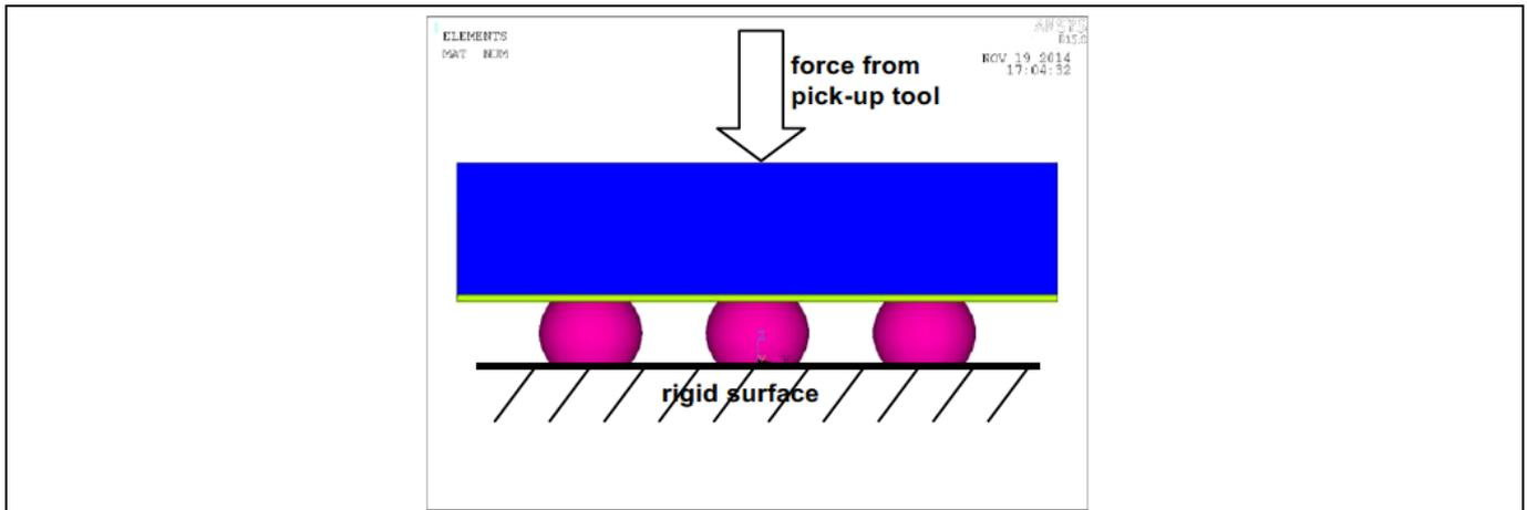
**Figure 7** Illustration of the simulation applying force to package top
