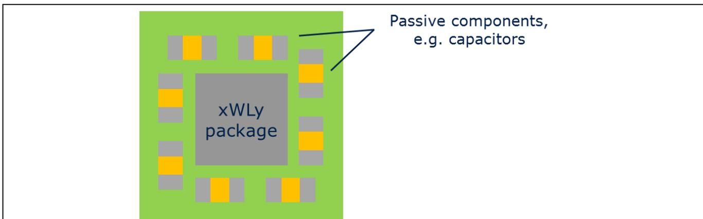
Figure 4 Schematic view of recommended placement of passive components around an xWLy package
