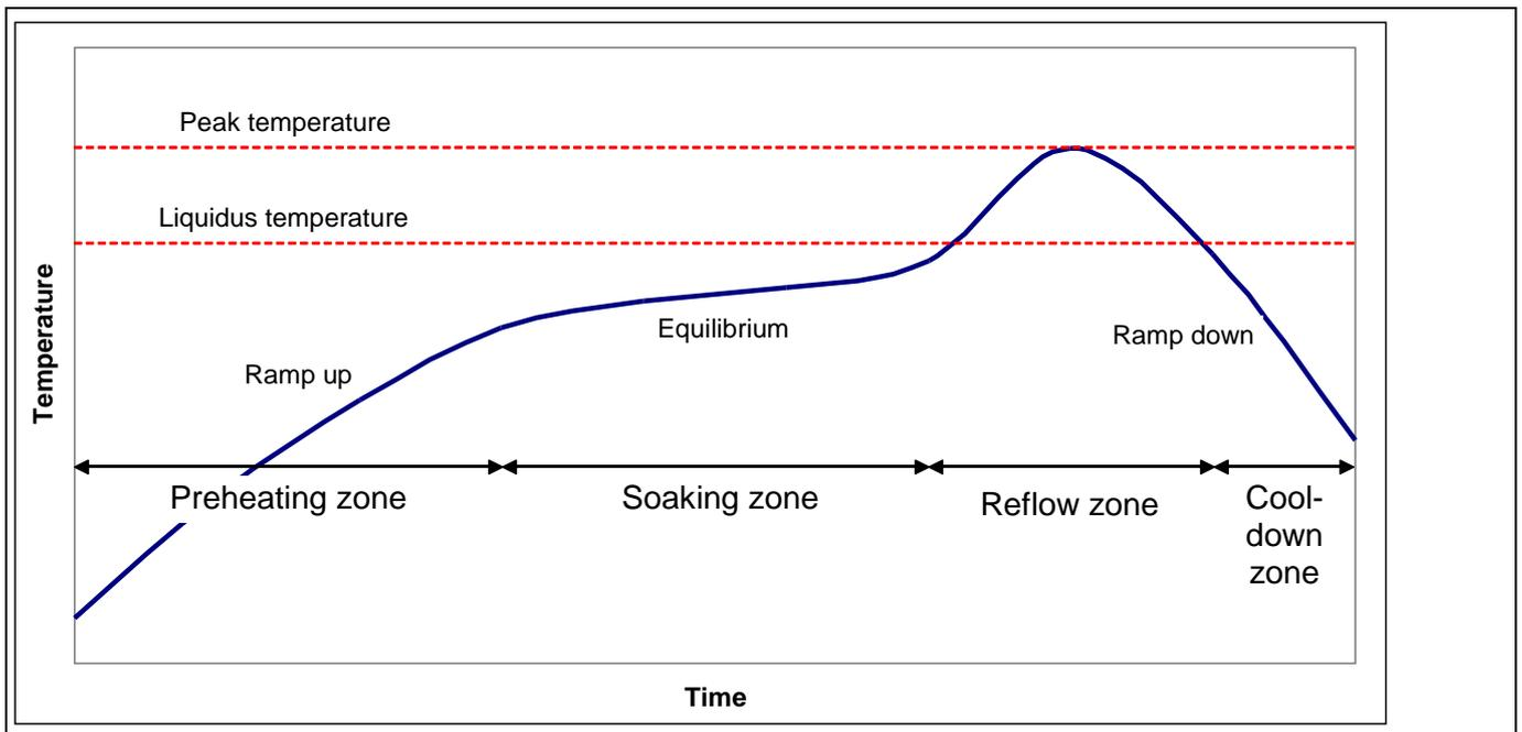
Figure 9 Various phases of a reflow solder profile
