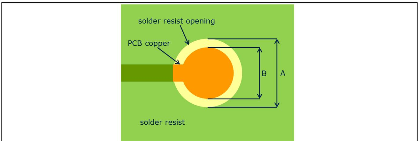
Figure 6 PCB pad design recommendation (NSMD pad)
