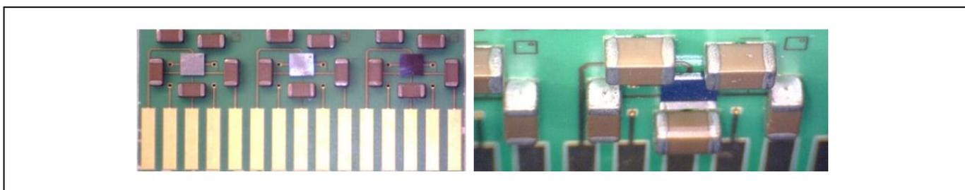
Figure 5 Typical PCB layouts using passive components to protect xWLy packages
