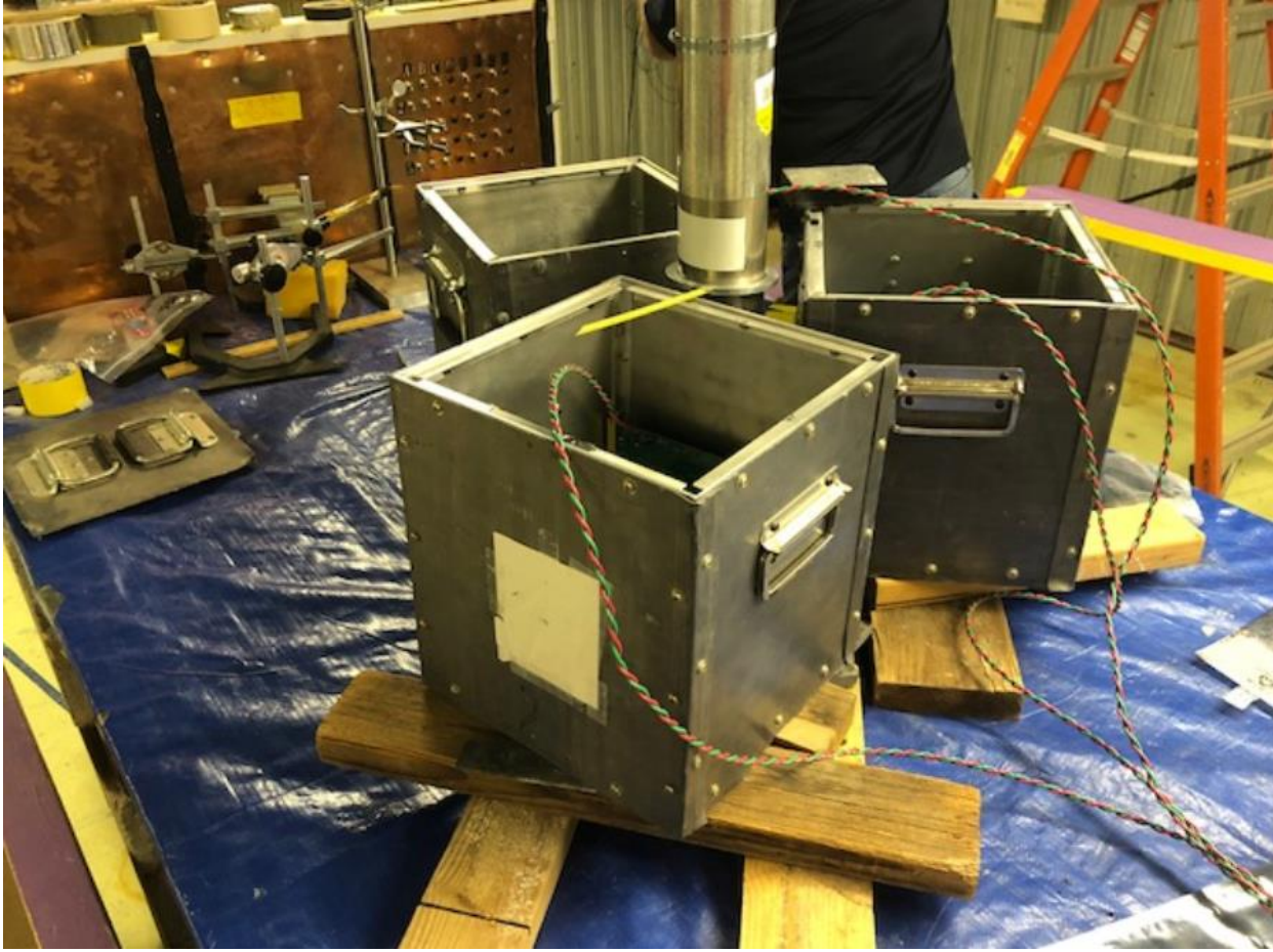
Figure 5. Three Bias Boards in Lead-Aluminum Boxes Surrounding CO-60 Shroud
