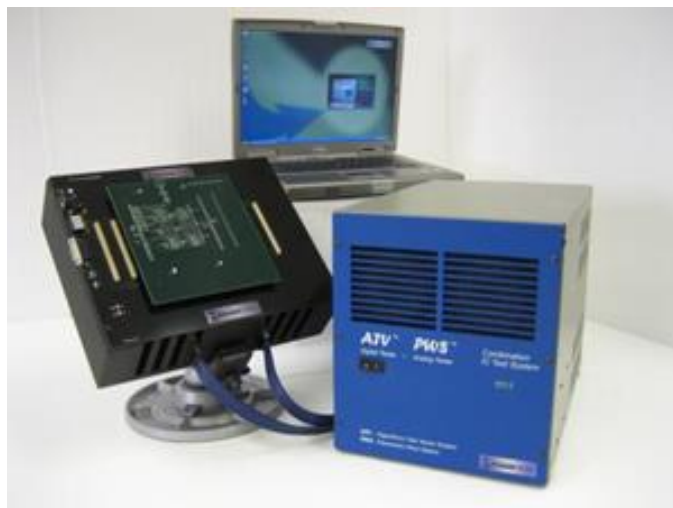
Figure 6. ATV Test System used for SEE Testing
