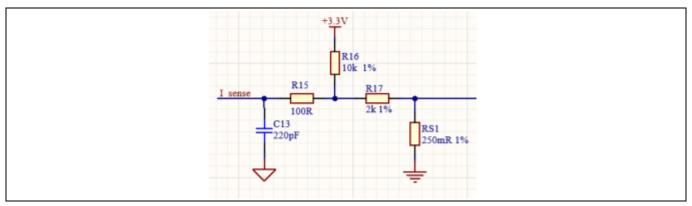
Figure 8 Current measurement shift stage
