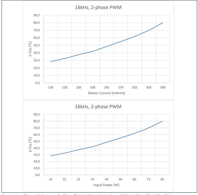
Thermal characterization of IMI111T-026H, 2-phase PWM, 16 kHz, FR4 PCB with 1 oz copper Figure 9
