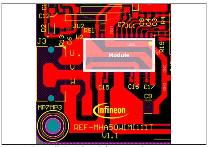
Figure 15 PCB layout used for thermal characterization: 1 oz copper, 1 layer
