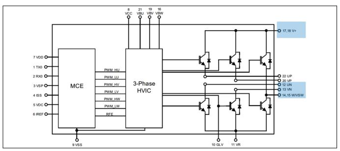
Figure 16 Critical pins for thermal PCB design
