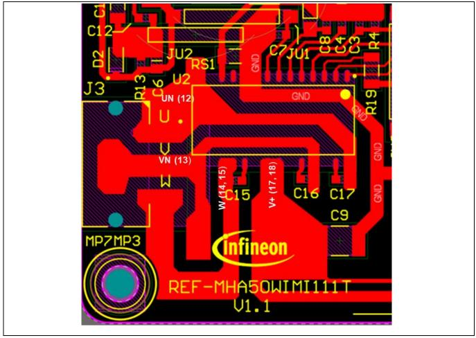
Figure 17 Reference board PCB design regarding critical pins
