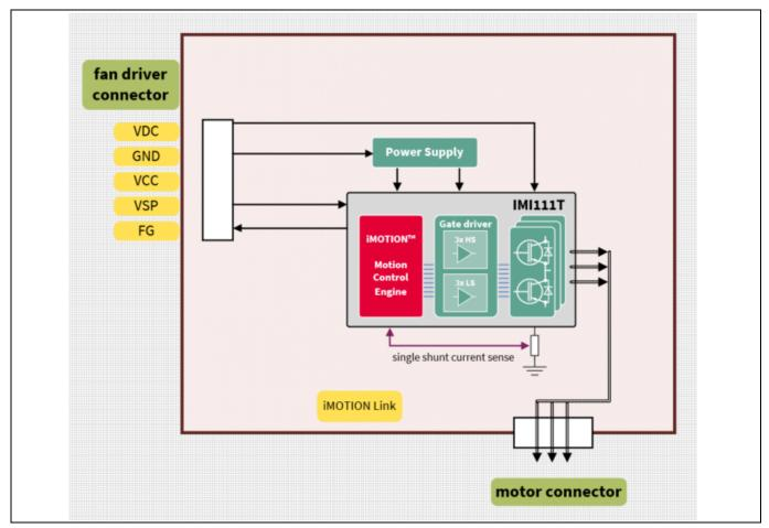
Figure 1 Block diagram of REF-MHA50WIMI111T
