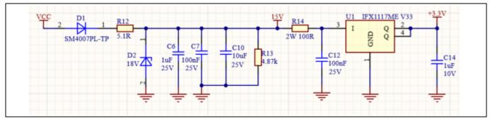
Figure 7 Power supply section of the REF-MHA50WIMI111T evaluation board
