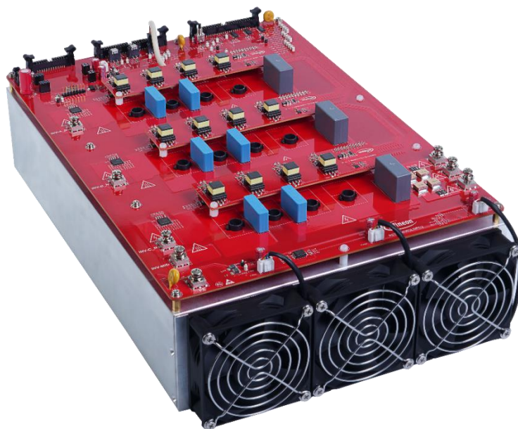
Power conversion board REF-10KW3LNPC2
