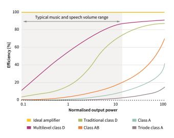
The graph shows efficiency as a function of output power for a range of different amplifier architectures.
