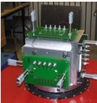
Fig. 11: experimental setup of vibration qualification
