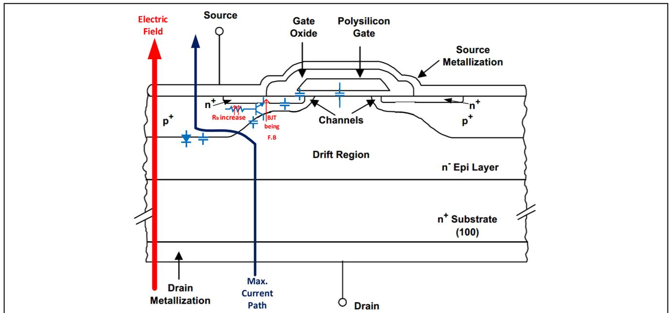
**Figure 5** Power MOSFET schematic under avalanche
