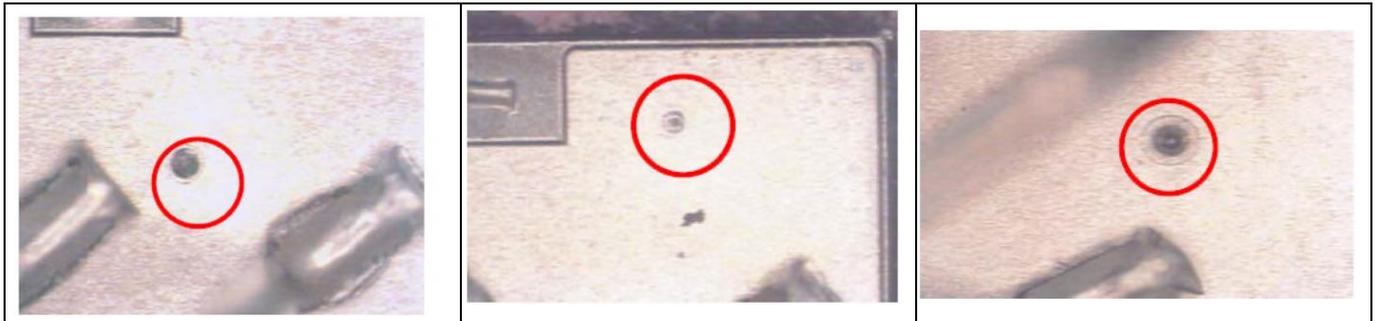
**Figure 7** Examples of power MOSFET random device failure spots
