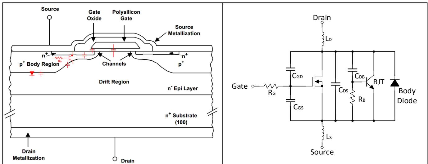
**Figure 4 Power MOSFET schematic (left) and circuit model (right)**
