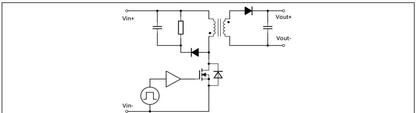
**Figure 1** Simplified flyback converter circuit example
