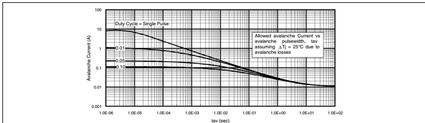
**Figure 17** Typical  $I_{AR}$  vs.  $t_{AV}$  for various duty cycles from the IRF7341GTRPbF datasheet
