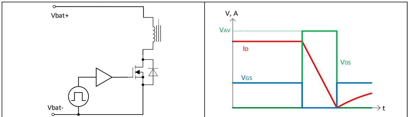
Figure 3 Simplified fuel injector coil circuit example (left) and illustrated waveforms in avalanche operation (right)
