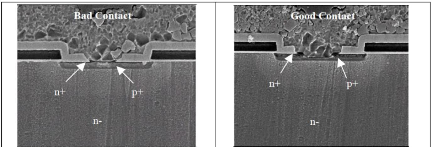
**Figure 8** Power MOSFET cross-section images – bad contact (left) and good contact (right)
