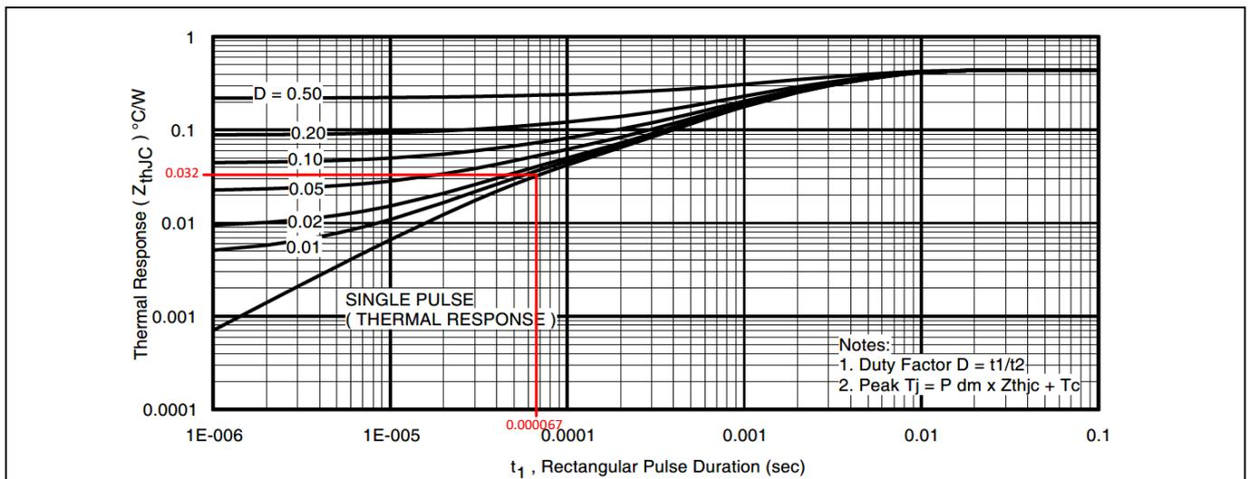
**Figure 14** Maximum effective transient thermal impedance, junction-to-case from IRF7749L1TRPbF datasheet
