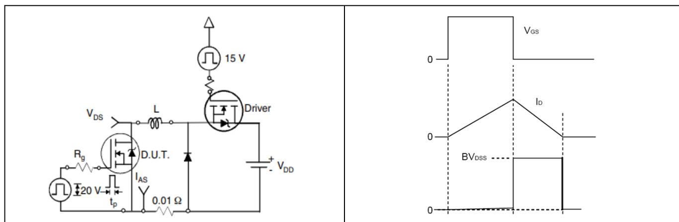
**Figure 11** Decoupled  $V_{DD}$  voltage source UIS test circuit (left) and illustrated output waveforms (right)
