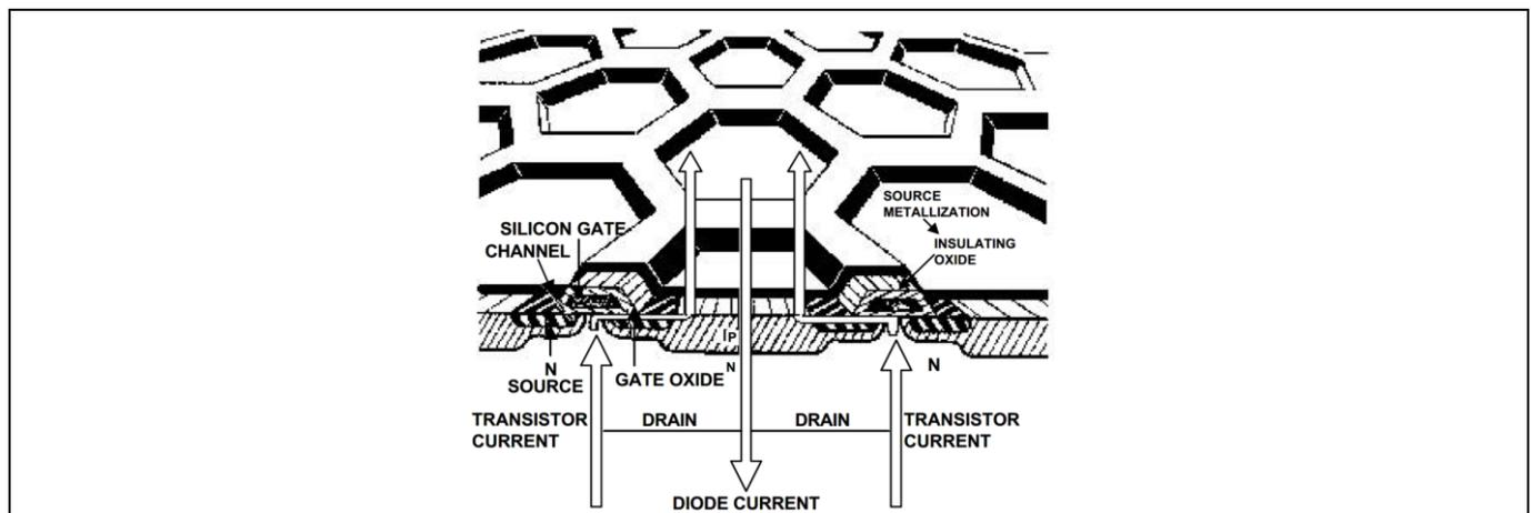
**Figure 6** Planar MOSFET structure example
