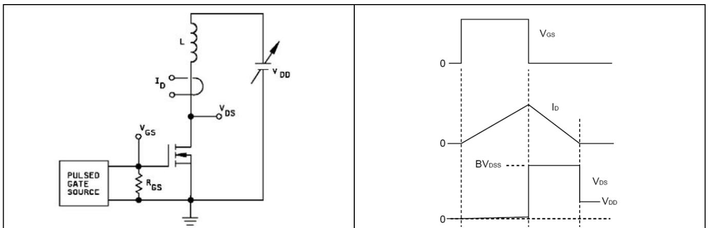
**Figure 10** Single pulse unclamped inductive switching test circuit (left) and illustrated output waveforms (right)
