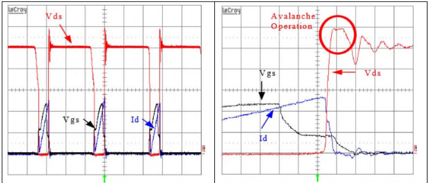
Figure 2 Flyback converter switch under avalanche waveforms (left) and detail (right)
