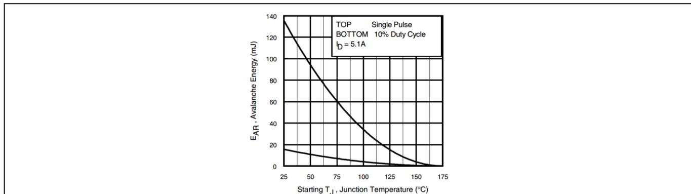
**Figure 16** Maximum  $E_{AR}$  vs.  $T_{START}$  for various duty cycles, single  $I_D$  from the IRF7341GTRPbF datasheet
