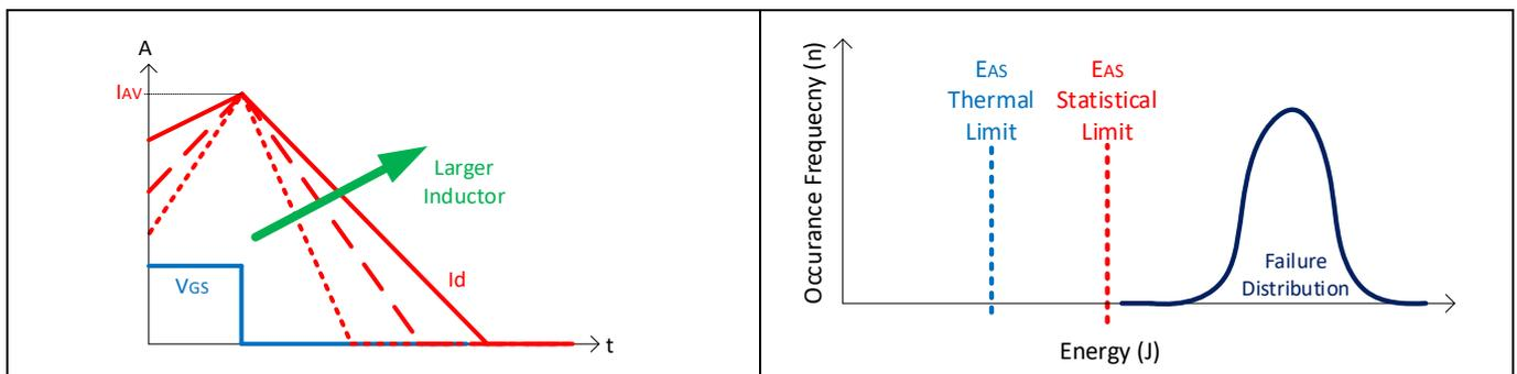
**Figure 20** Illustrated  $I_{AS(set)}$  vs.  $t_{AV}$  waveforms for various inductors (left) and failure energy distribution with limits (right)
