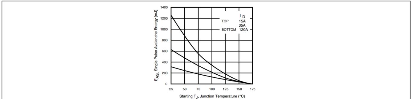
**Figure 15** Maximum avalanche energy vs. temperature for various  $I_D$  values from the IRF7749L1TRPbF datasheet
