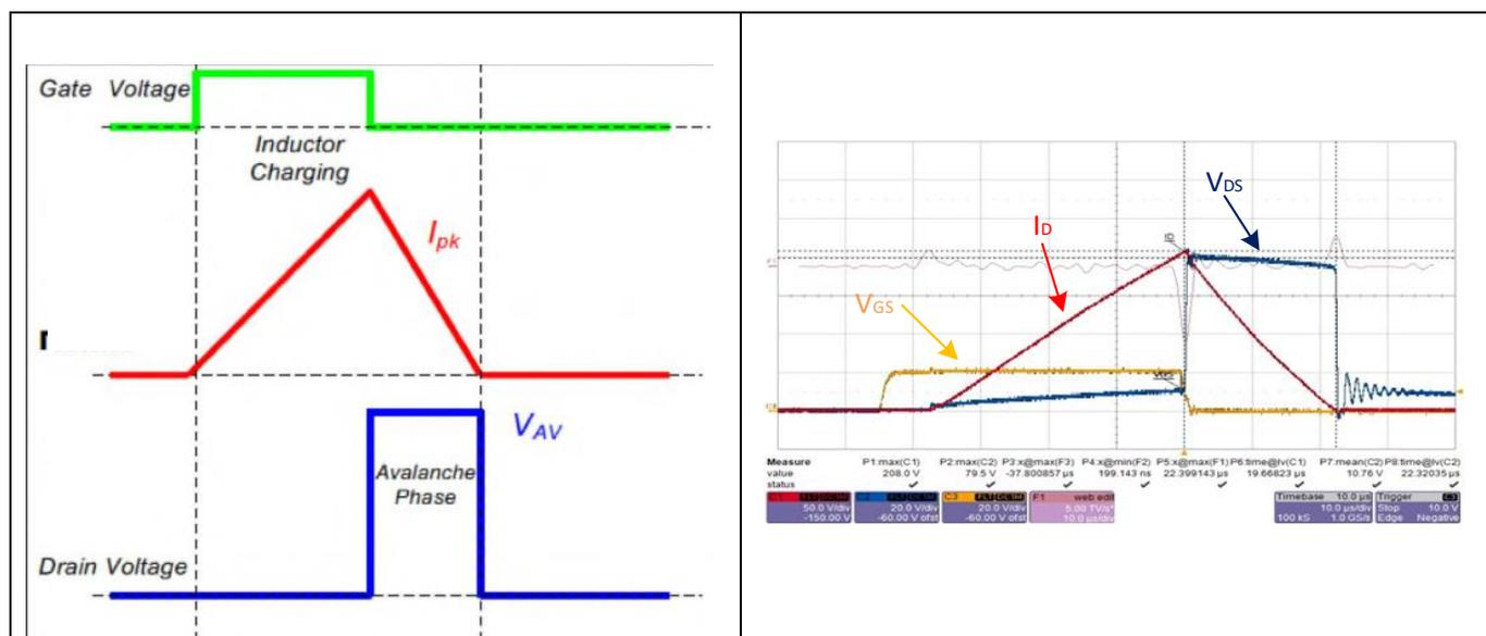
**Figure 12** Ideal illustrated avalanche waveform (left) and actual waveforms example (right)
