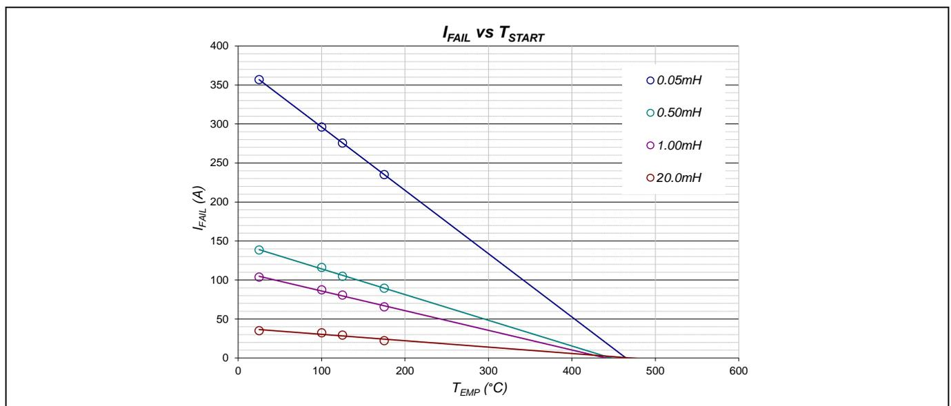
**Figure 9** Example plot of  $I_{AS}$  at failure vs.  $T_{START}$  with various inductances
