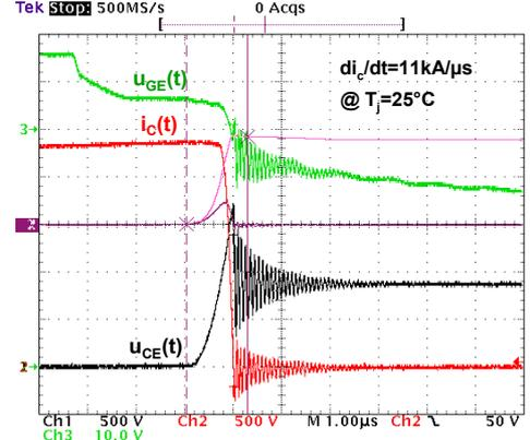
Fig. 2. Waveforms of FZ2400R17KE3 during turn-off,  $U_{DC}=900V$ ,  $I_C=2.4kA$ ,  $E_{OFF}=920mJ$ ,  $U_{CEmax}=1.72kV$ ,  $R_G=3.6\Omega$ ,  $L_Q=50nH$
