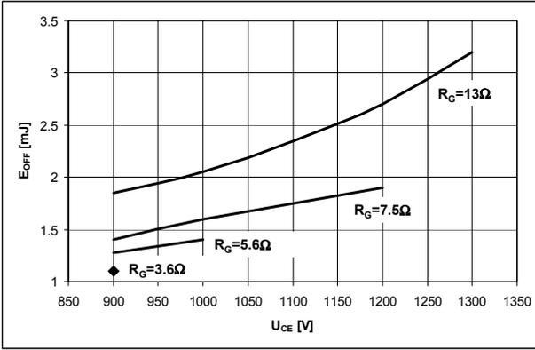
Fig. 4. Comparison of energy losses during turn-off transients of FZ2400R17KE3 versus value of the gate resistor and DC voltage link when:  $I_C = \text{const} = 2400\text{A}$ ,  $T_J = 125^\circ\text{C}$ ,  $L_O = 50\text{nH}$
