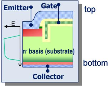
Fig. 1. Vertical cross-section of Trench-/Field-Stop IGBT structure.
