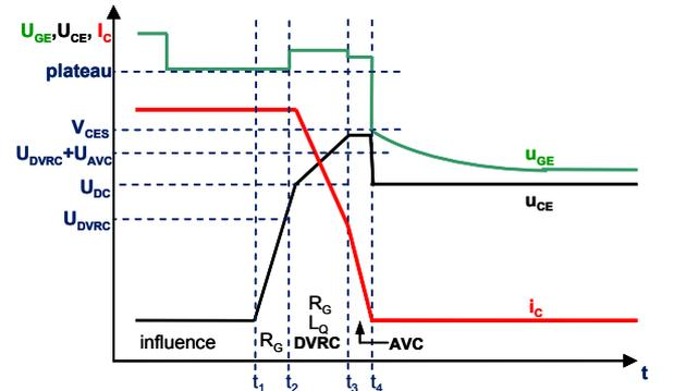
Fig. 6. Theoretical waveforms of DVRC functionality
