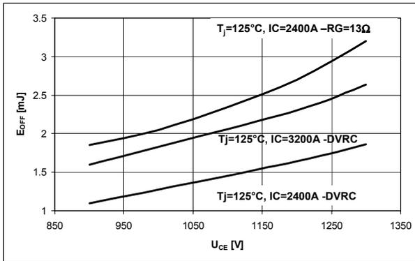
Fig.12. Comparison of energy losses during turn-off of FZ2400R17KE3 between DVRC and gate resistor method versus DC voltage link at:  $I_C=2400A/3200A$ ,  $T_j=125^\circ C$ ,  $L_Q=50nH$
