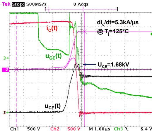
Fig.11. Waveforms of FZ2400R17KE3 during turn-off,  $U_{DC}=1300V$ ,  $I_C=3.2kA$ ,  $E_{off}=2.64J$ ,  $U_{CEmax}=1.68kV$ ,  $R_G=2\Omega$ ,  $L_Q=50nH$
