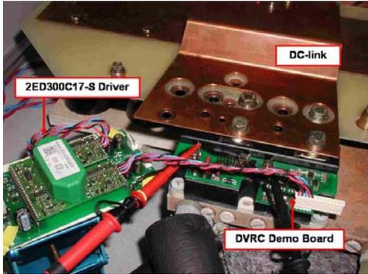
Fig. 9. A part of laboratory setup for FZ2400R17KE3 module investigation
