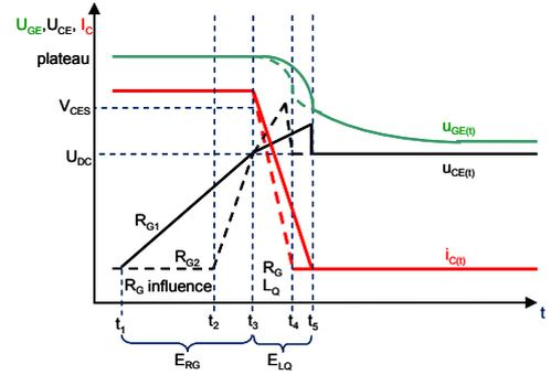
Fig. 3. Influence of gate resistor value on turn-off performances in theory when  $R_{G1} \gg R_{G2}$
