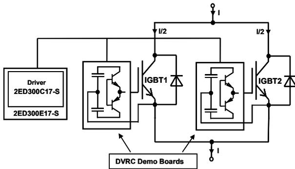
Fig. 7. Block diagram for IGBT paralleling using DVRC technology.
