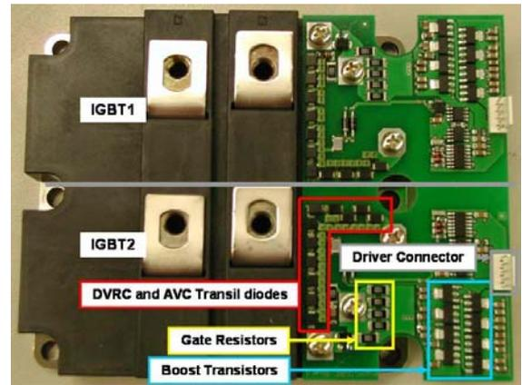
Fig. 8. FF1200R12KE3 - half bridge module equipped with suitable DVRC demo board.
