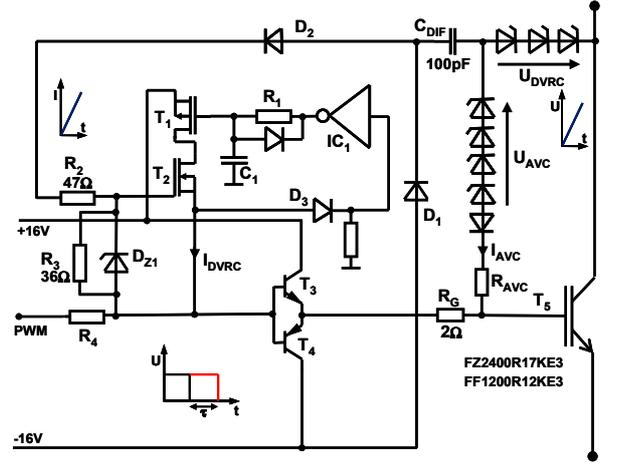
Fig. 5. Operational circuit diagram of DVRC function
