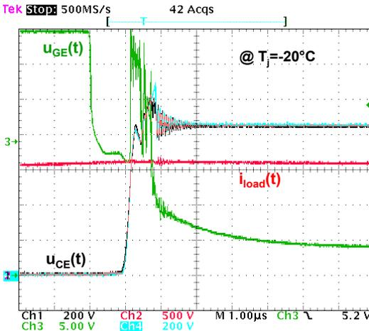
Fig. 13. Waveforms of FF1200R12KE3 connected in parallel during turn-off,  $U_{DC}=900V$ ,  $I_C=1680A$ ,  $U_{CEmax}=1100V$ ,  $R_G=2\Omega$ ,  $L_Q=50nH$
