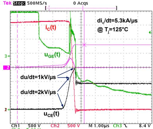
Fig. 10. Waveforms of FZ2400R17KE3 during turn-off,  $U_{DC}=900V$ ,  $I_C=3.2kA$ ,  $E_{off}=1.6J$ ,  $U_{CEmax}=1.48kV$ ,  $R_G=2\Omega$ ,  $L_Q=50nH$
