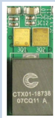
DC/DC converter stage with Blade 3x3 package (driver on backside of the PCB)
