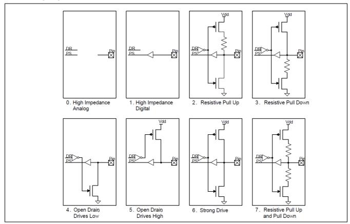
The following diagram illustrates the various available GPIO output drive modes.
