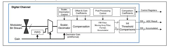
Figure 10 Digital channel data path
