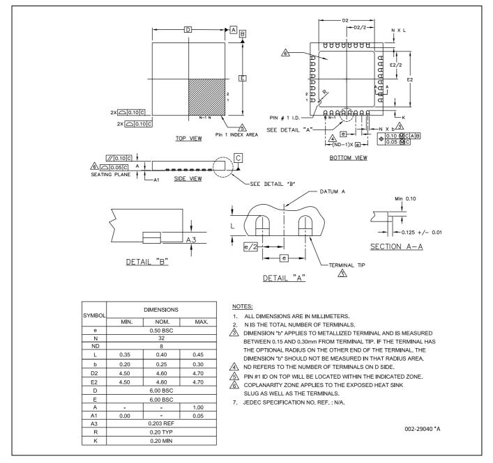
Figure 24 32-Pin QFN with wettable flank (6.0 × 6.0 × 1 mm)
