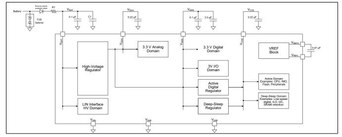
Figure 1 Power system block diagram
