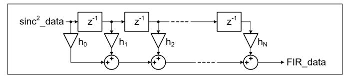
Figure 14 General structure of the FIR filter
