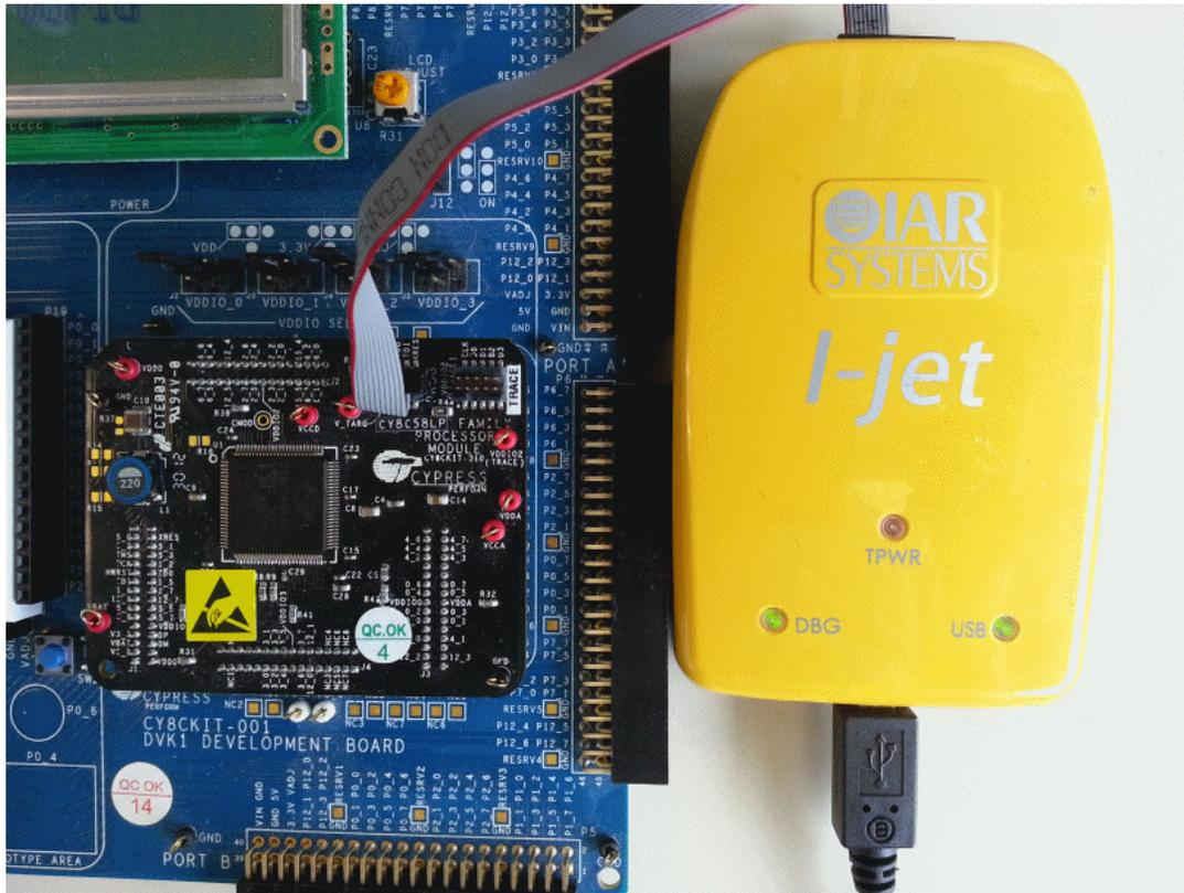
For **PSoC 4/PRoC BLE**, connect the I-jet with 10-pin adapter to the "PSoC 4/PRoC BLE Prog" 10-pin connector on the CY8CKIT-042 (Pioneer Kit).
