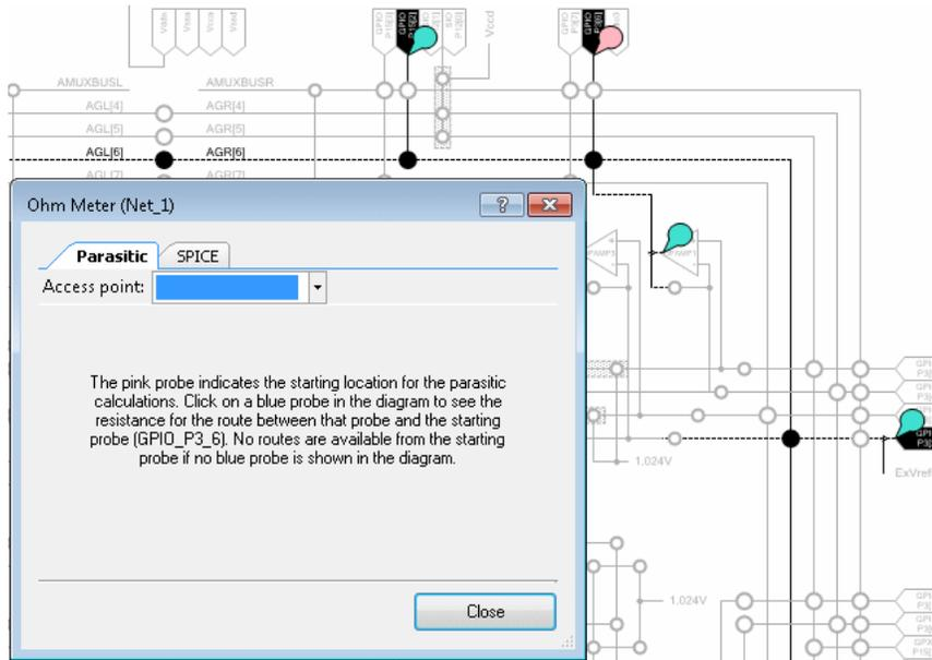
Probes are displayed in the interconnect diagram with an attached pin. The first-placed pin is pink and, when it is placed, all legal destination probe points are automatically marked with blue probes. Select a blue pin to see the resistance for that route. Re-selecting the start-point for probing clears previous probes, clears the dialog results, and refreshes the legal destination (blue) probes.
