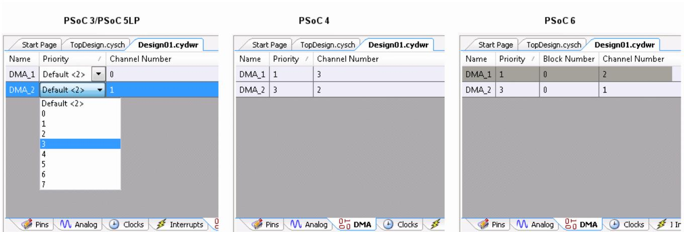
The image shows three screenshots of the DMA Editor interface for different PSoC devices. Each screenshot displays a table with columns for Name, Priority, and Channel/Block Number, and a dropdown menu for selecting a channel number.
