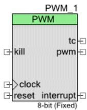
3. In the Component Catalog, expand the "Digital > Logic" folder, drag a Logic Low Component onto your design, and connect it to the **kill** terminal on the PWM. Connect another Logic Low to the **reset** terminal.
