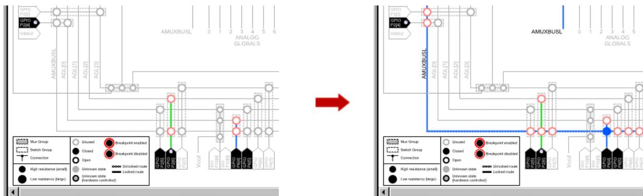
Open switches are shown as hollow circles; closed switches are shown as solid circles.
