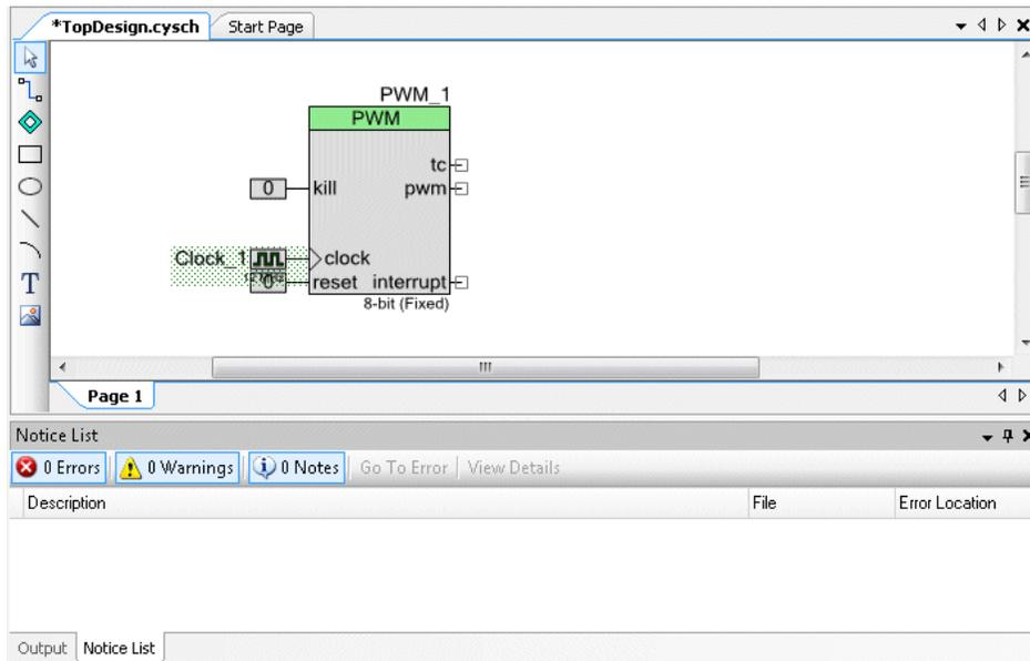
5. Double-click the Clock to open the Configure dialog, change the **Desired Frequency** value to 0.25 kHz, and click **OK**.
