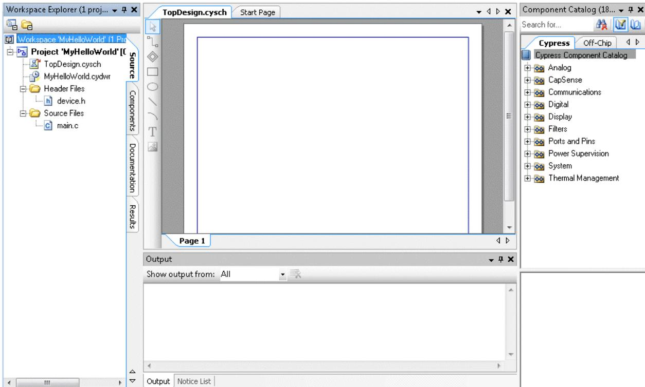
The [Schematic Editor](#) displays the top-level schematic file (*TopDesign.cysch*) as a document window, and the [Component Catalog](#) opens to display a list of Components to use in your design.
