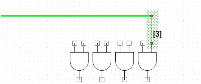
8. Connect the bus to each of the other single-bit terminals. Label them [0], [1], and [2], respectively, using the same process as described above.
