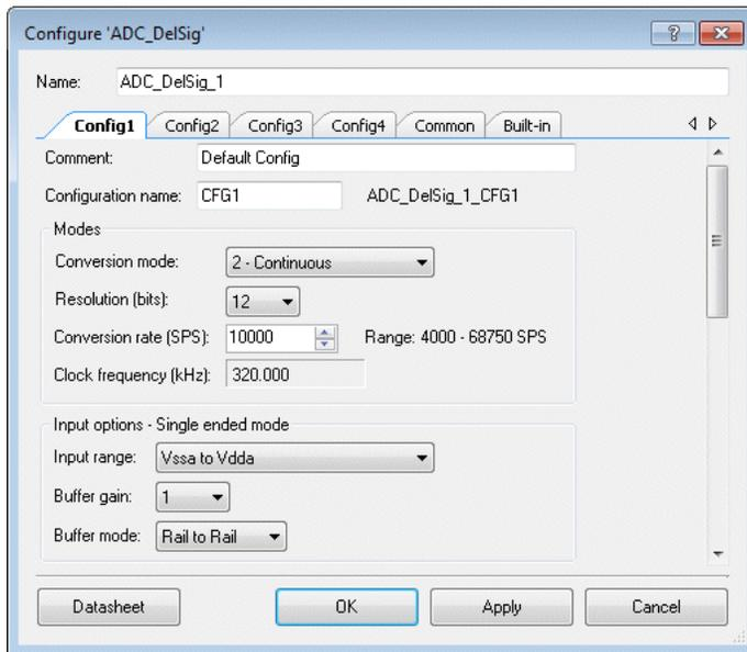
By default, the Delta Sigma ADC is configured as 16-bit, with an input range of +/- 1.024 V. For more information about the Delta Sigma ADC Component, refer to its datasheet.
