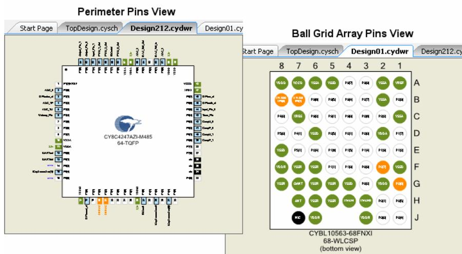
The coloring of the pins, as well as the port/pin numbers and labels are the same for both views. The process for assigning and locking pins is also the same for both views. However, for the perimeter view, any assigned signal name displays adjacent to the pin, but it doesn't for the ball grid array view.
