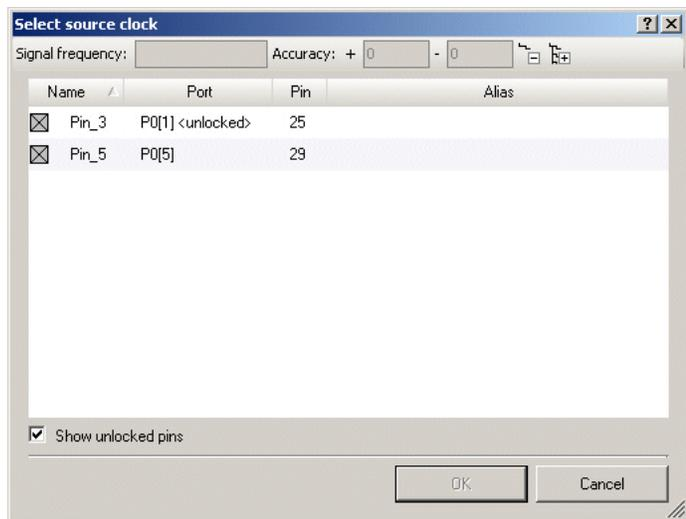
To be used as a clock input, a signal must meet be a digital input pin.
