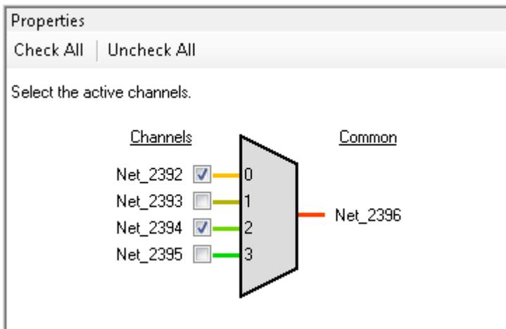
The diagram includes check boxes to choose the active channel(s) of the mux. It also shows the net names associated with each channel and the common terminal. The coloring for each net will be the same as that chosen in the table. When you select and de-select a channel, the change is reflected in the interconnect diagram and the Ohm meter.
