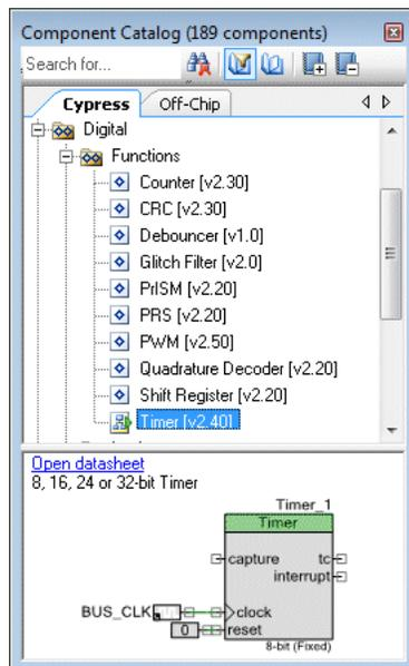
Notice that the Timer is already connected to a Clock Component and a Logic Low Component. This is because the Timer is an example of a [Schematic Macro](#).
