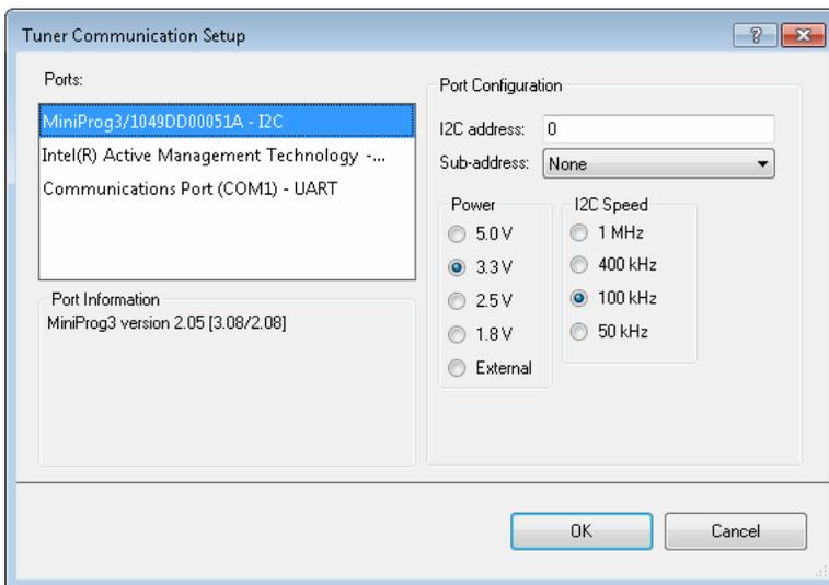
Currently, tuners only support communication via I<sup>2</sup>C. This can be done using the EZ I<sup>2</sup>C Component or the standard I<sup>2</sup>C Component.
