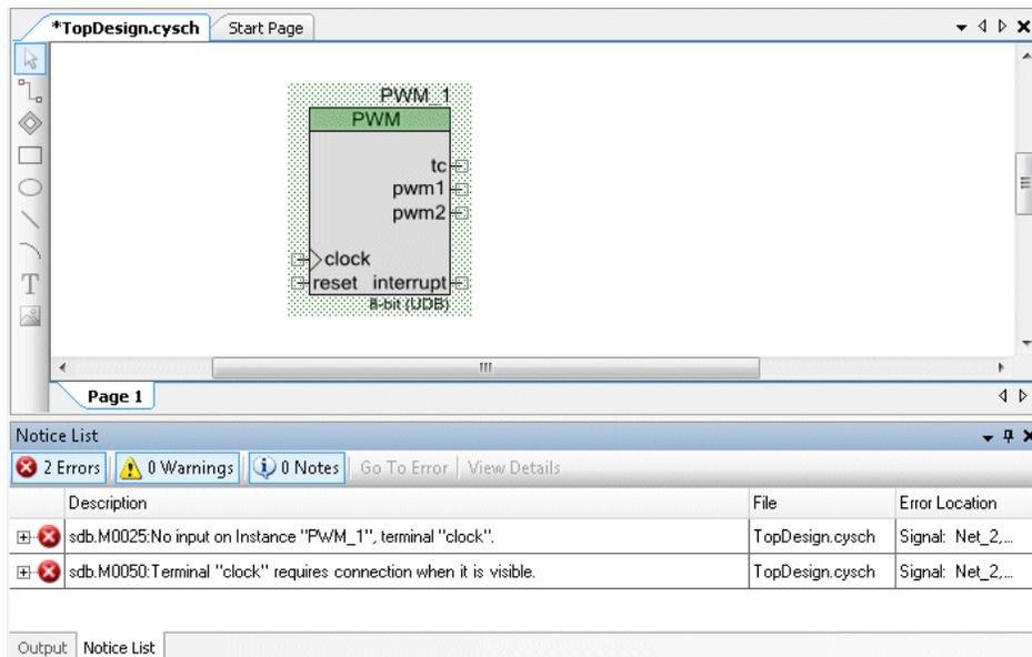
2. Double-click the PWM Component to open the Configure dialog, change the **Implementation** setting to "Fixed Function," and click **OK**.
