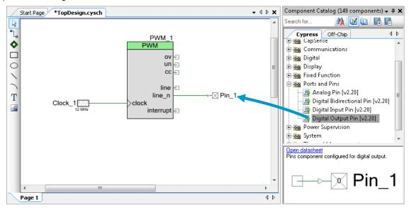
If needed, connect various components using the Wire tool.
