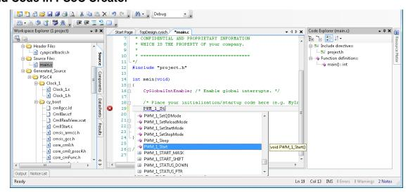
Inside PSoC Creator, open the main.c file and insert the necessary code for your application.
