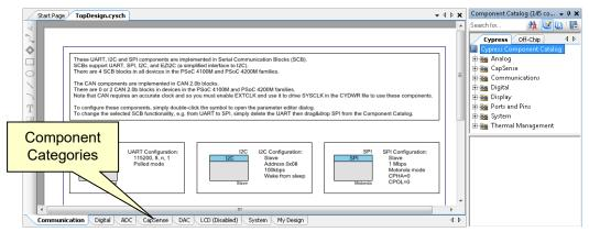
As needed, add a Pin, Clock, and other Components to complete the design by dragging items from the Component Catalog.
