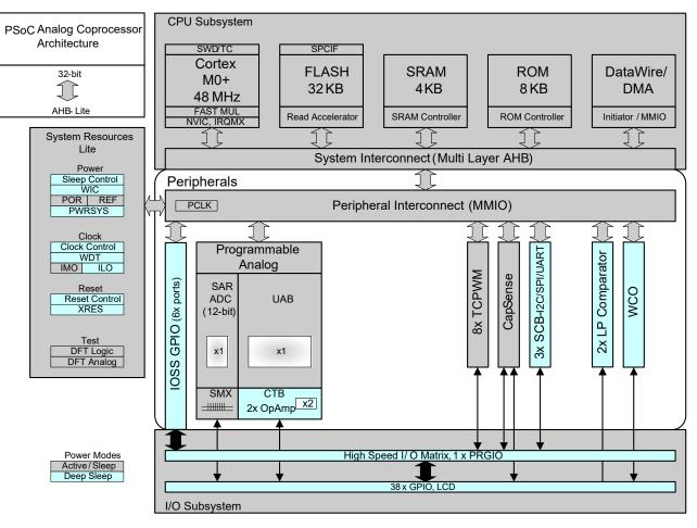
Figure 2. Block Diagram
