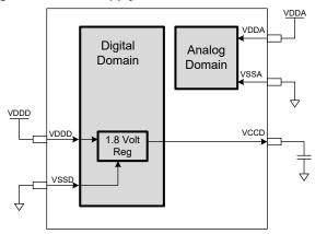
There are two distinct modes of operation. In Mode 1, the supply voltage range is 1.8 V to 5.5 V (unregulated externally; internal regulator operational). In Mode 2, the supply range is  $1.8 \text{ V} \pm 5\%$  (externally regulated; 1.71 to 1.89, internal regulator bypassed).
