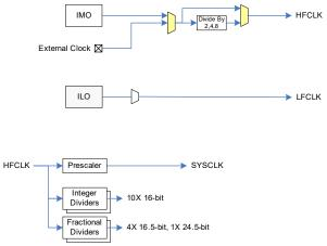
The HFCLK signal can be divided down to generate synchronous clocks for the analog and digital peripherals. There are 15 clock dividers for the PSoC Analog Coprocessor. The 16-bit capability allows flexible generation of fine-grained frequency values (there is one 24-bit divider for large divide ratios), and is fully supported in PSoC Creator.
