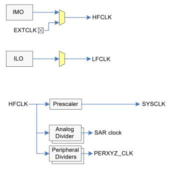
The HFCLK signal can be divided down (see PSoC 4100 MCU Clocking Architecture) to generate synchronous clocks for the analog and digital peripherals. There are a total of 12 clock dividers for PSoC 4100, each with 16-bit divide capability. The analog clock leads the digital clocks to allow analog events to occur before digital clock-related noise is generated. The 16-bit capability allows a lot of flexibility in generating fine-grained frequency values and is fully supported in PSoC Creator.
