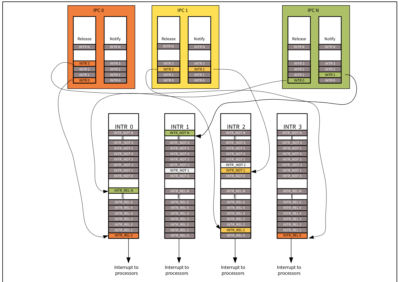
Figure 6-4. IPC channels and interrupts
