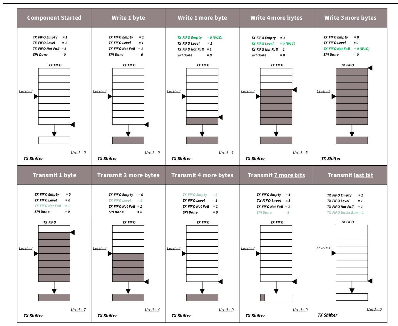
Figure 27-46. TX interrupt source operation
