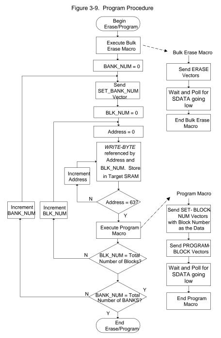
A Bulk Erase operation must be executed to prepare the flash for programming.
