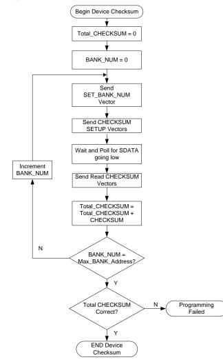
To get the Checksum Value from the target, the programmer sends the appropriate CHECKSUM-SETUP vector to the target. The programmer releases the SDATA line, then waits and polls. After the target signals that the operation is complete, the READ-CHECKSUM vector reads back the two-byte checksum value from the target. This value from the target is compared to the device checksum value from the *.hex* file (Appendix B on page 27). If the values are not equal, a programming error has occurred.
