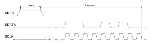
Figure 3-5. Using Reset to Initialize
