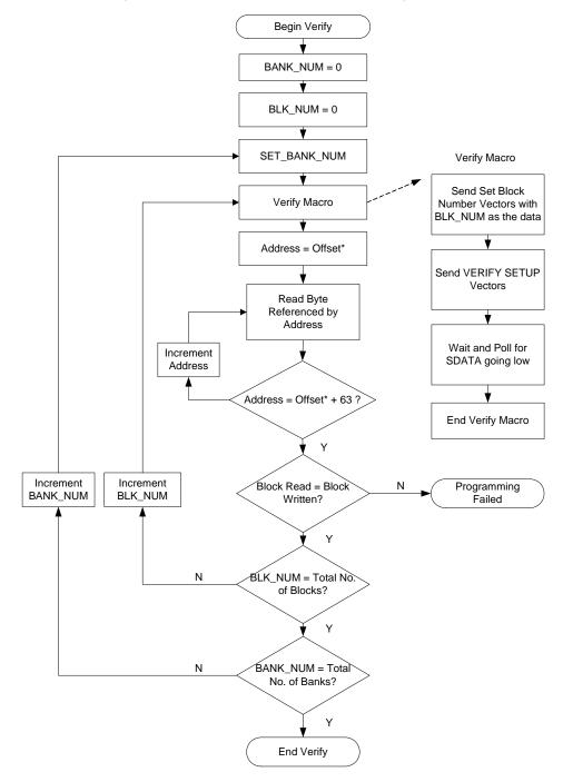
Figure 3-12. Verify Procedure (Offset = 0x80 in figure)
