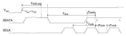
Figure 3-6. Using Power Cycling to Initialize
