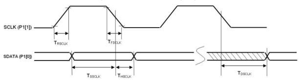
Figure 3-2. SCLK, SDATA Timing Diagrams
