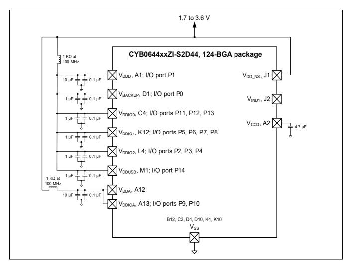
Figure 14 124-BGA (No Buck) Power Connection Diagram
