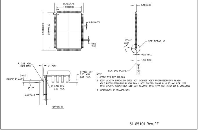
Figure 18 A128RA package outline (PG-TQFP-128), 51-85101
