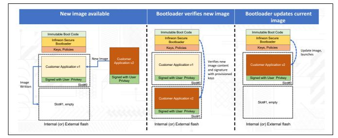
**Figure 12** shows a typical application update scenario using the bootloader:
