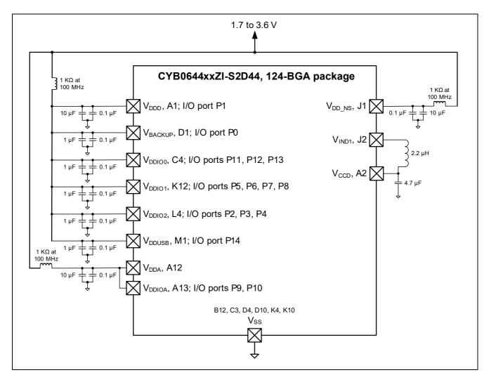
Figure 13 124-BGA Power Connection Diagram
