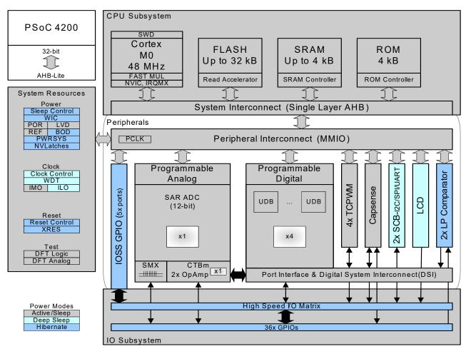
The PSoC 4200 devices include extensive support for programming, testing, debugging, and tracing both hardware and firmware.
