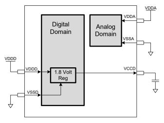
The PSoC 4200 family allows two distinct modes of power supply operation: Unregulated External Supply and Regulated External Supply modes.
