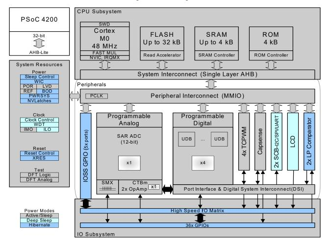
Figure 2. Block Diagram
