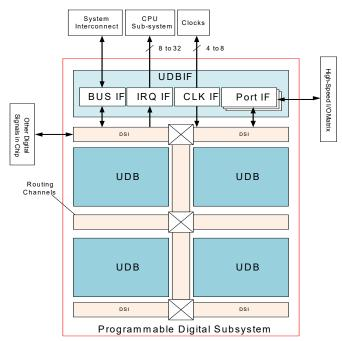
UDBs can be clocked from a clock divider block, from a port interface (required for peripherals such as SPI), and from the DSI network directly or after synchronization.
