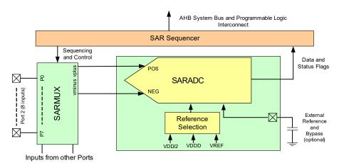
Figure 4. SAR ADC System Diagram
