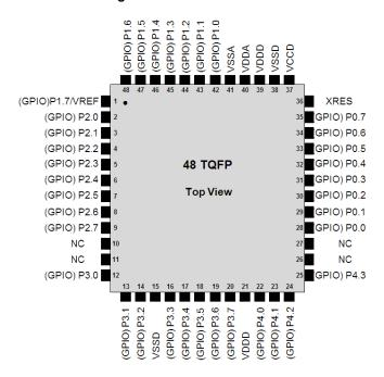
Figure 7. 48-Pin TQFP Pinout
