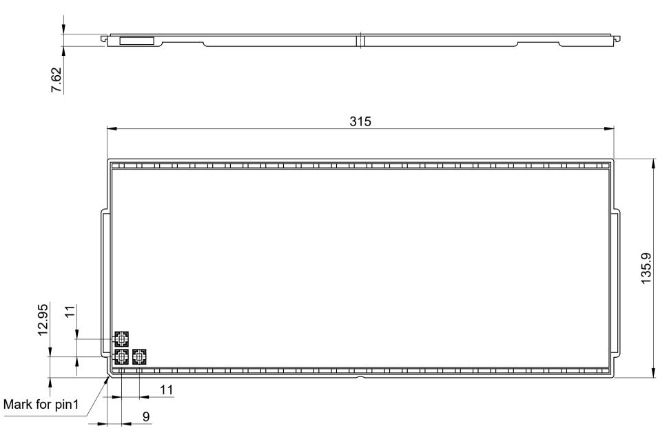
All dimensions are in units mm The drawing is in compliance with ISO 128-30, Projection Method 1 [ $\bigcirc \oplus$ ]
