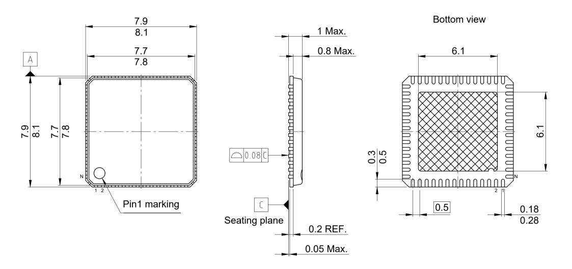
$\boxtimes$  Hatch is solderable exposed metal.All dimensions are in units mm  $\frac{\min}{\max}$ .The drawing is in compliance with ISO 128-30, Projection Method 1 [ ] ]
