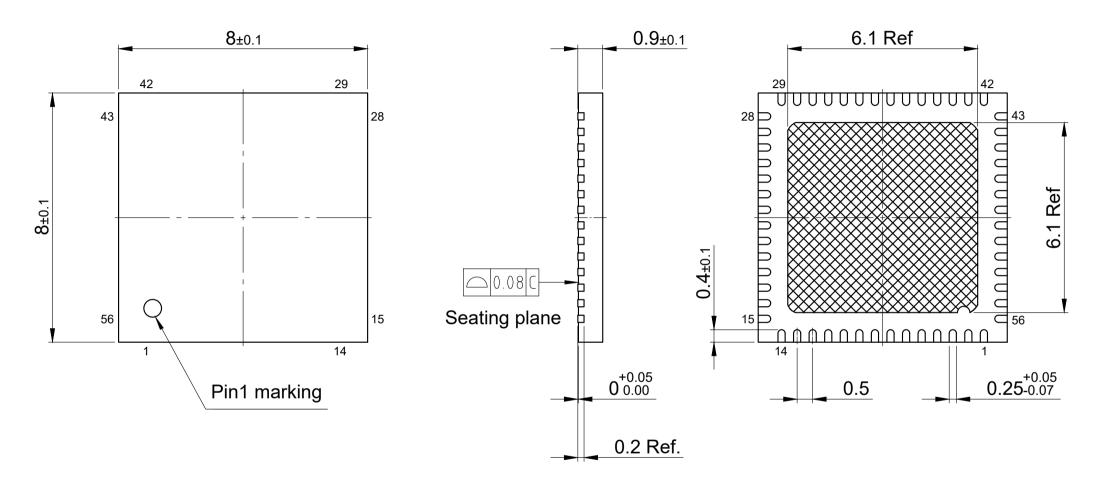
$\boxtimes$  Hatch area is solderable exposed metal.
