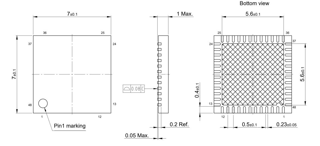
$\boxtimes$  Hatch area is solderable exposed metal.
