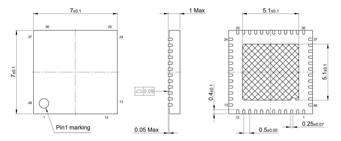
Hatch area is solderable exposed metal. All dimensions are in units mm The drawing is in compliance with ISO 128-30, Projection Method 1 [-]
