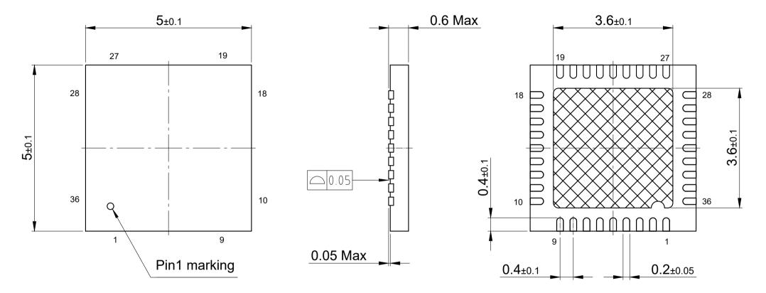
$\boxtimes$ Hatch area is solderable exposed padAll dimensions are in units mmThe drawing is in compliance with ISO 128-30, Projection Method 1 [ ] []
