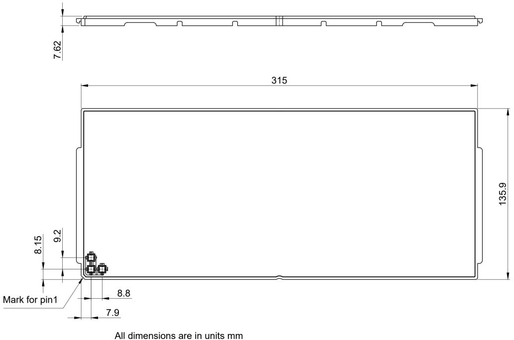
The drawing is in compliance with ISO 128-30, Projection Method 1 [ $\bigcirc \oplus$ ]
