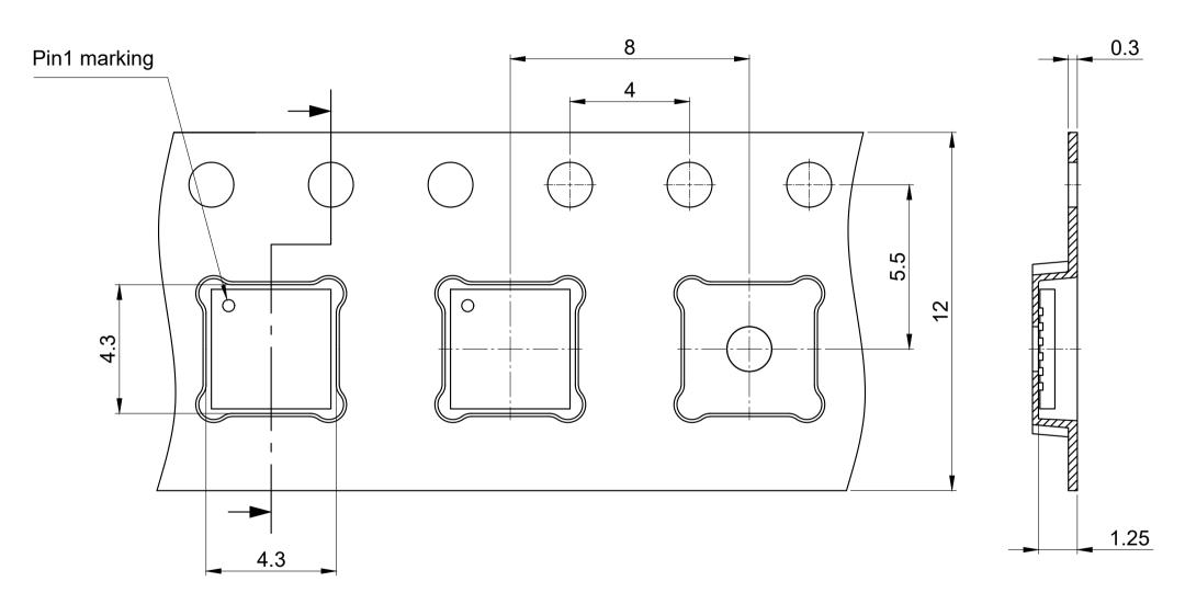
All dimensions are in units mm The drawing is in compliance with ISO 128-30, Projection Method 1 [ $\bigcirc \phi$ ]
