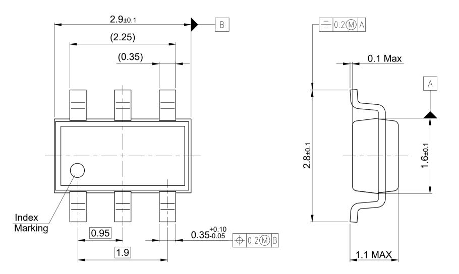
All dimensions are in units mm The drawing is in compliance with ISO 128-30, Projection Method 1 [
