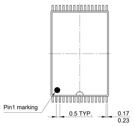
All dimensions are in units mm  $\frac{\text{min.}}{\text{max.}}$ The drawing is in compliance with ISO 128-30, Projection Method 1 [
