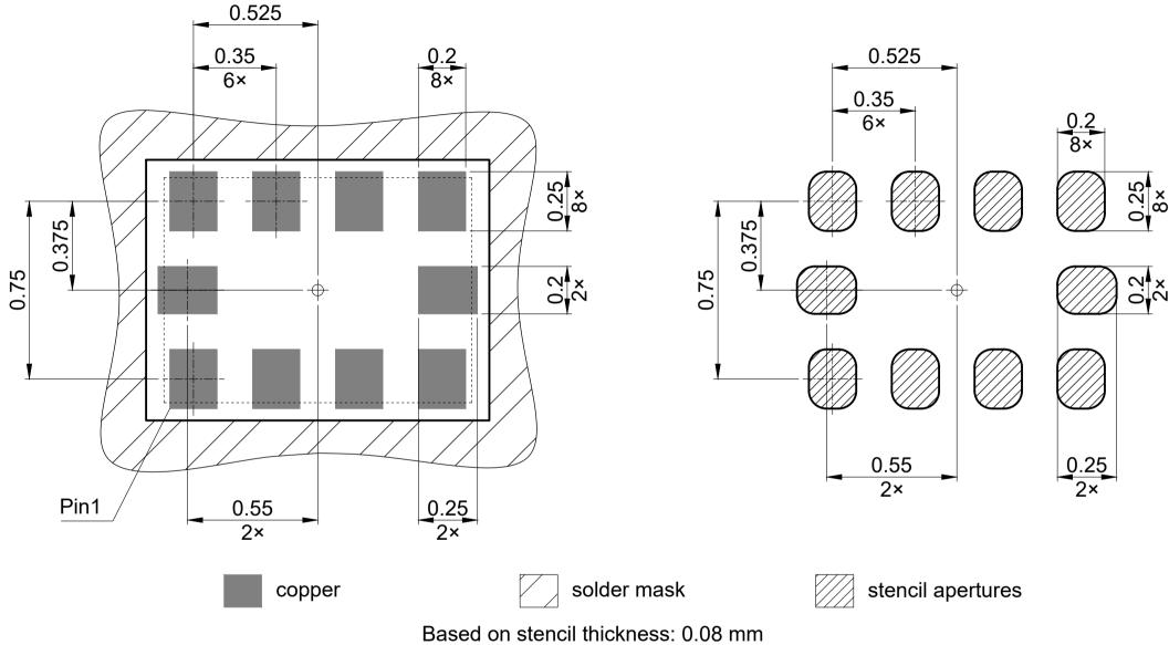
Based on steller trickless. 0.06 mill Based on solder paste: type 5
