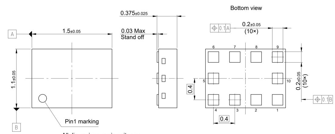
All dimensions are in units mm The drawing is in compliance with ISO 128-30, Projection Method 1 [  $\bigcirc$   $\bigcirc$  ]
